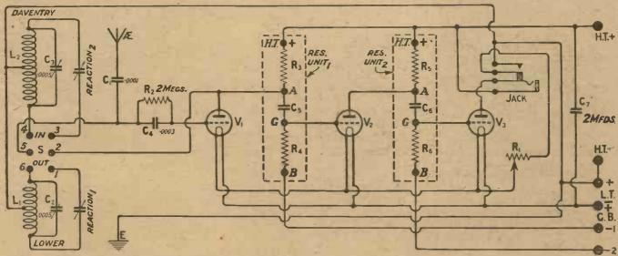
Fig. 1.-A filament switching jack is used, so that the set is brought into operation by inserting the loud-speaker plug.
