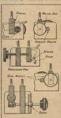
Fig. 2.—Some of the mechanical principles applied to the slow-motion control of coil holders are illustrated here
