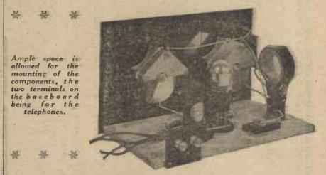
receiver such as this. There are only eight holes to be drilled in the panel, two of these, namely, those for the variable condensers, being 9-16th in. in diameter. If you do not happen to possess a drill of this size drill the should be drilled in the proper positions when the other panel drilling is
