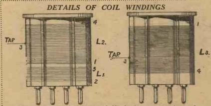
Fig. 4.—The coils are wound with No. 34 d.s.c. copper wire on the bakelite formers, turns touching.
