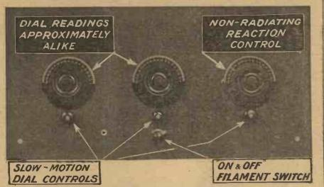
The tuning controls are simple, full non-radiating reaction is provided, and one switch brings the set into operation.
