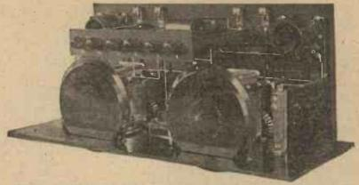
In the American Grebe receiver a form of "reduction gearing" is provided by presenting only the edge of the dial to the hand of the operator.
