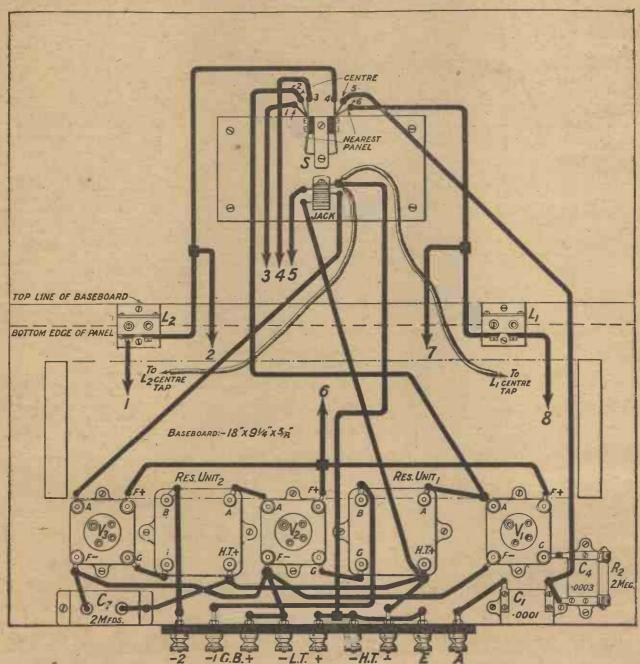
Fig. 4.—The numbered connections on the lower back-of-panel diagram go to the correspondingly numbered points on the sub-panel, shown above. Blueprints Nos. 1066C and 1066D are also available.
