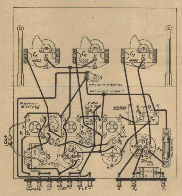
Fig. 5.—The layout of the components on the baseboard should be adhered to accurately. A full-size Blueprint,
