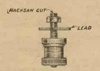
Fig. 1.—This method of adapting a terminal for connections is easiest with 2 B.A. shanks.
