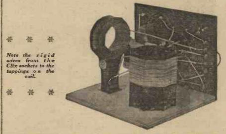
wire through these, so that it is quite secure, and commence winding the first turn about & inch from the end of the to prevent the latter coming loose, drill a small hole through the base of one of the ridges on the former.
