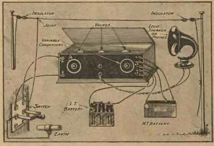
Fig. 1.—Here are the principal points in the set and its accessories which are likely to need attention.
