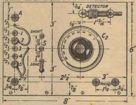
Fig. 2.—The dimensions for laying out the panel may be taken from this diagram. Blueprint No. 1068A is also obtainable.
