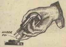
Fig. 1.—This method of inserting a valve in its holder will prevent damage to the filament.
