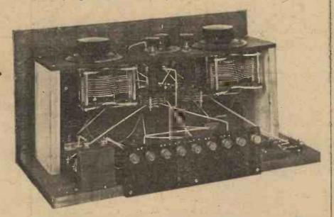
This view of the set shows clearly the disposition of the wiring to the components on the tuning control panel.
