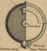
Fig. 1.—This form of geared dial is rotated by means of the small knob at the bottom, which turns a pinion engaging with the large gear wheel fixed on the spindle.
