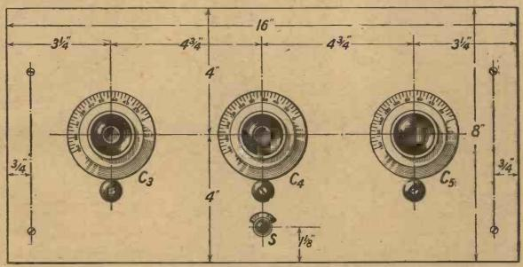
Fig. 2.—No difficulty should be experienced in laying out the panel, with the aid of this drawing. Blueprint, No. C1059A, is also obtainable.
