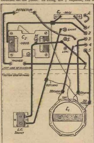
Fig. 3.-Note that stiff wire leads connect the tap-, pings on the coil
