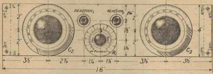
Fig. 2.—The drilling layout of the panel carrying the tuning controls is quite simple. Blueprint No. 1066A.
