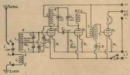
Fig. 1.—In this circuit diagram C1 and C2 represent the two halves of the balancing condenser.
