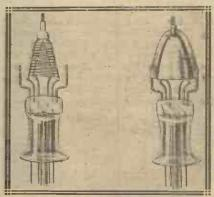
Showing the disposition of the electrodes in the Cossor Point One valves,
