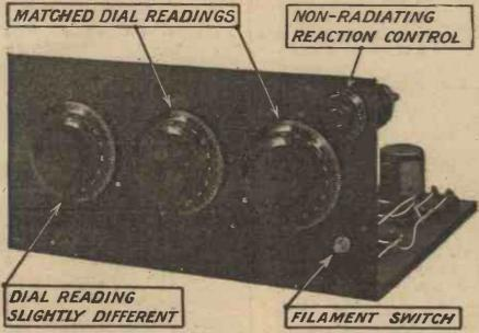
The operation of the "Night Hawk" is rendered simple by the small number of controls to be handled. A single switch sets all the valves
