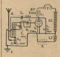
In order to make reaction possible over the whole of the broadcast range, a small fixed condenser Co was connected as shown, so that the aerial
