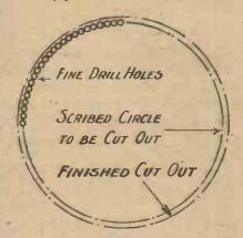
Fig. 1.—When no special tool is available, a large hole may be made in the manner shown.
