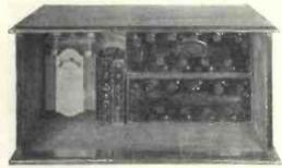
This photograph shows how the batteries are placed in position before the set itself is positioned
