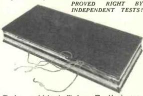
The frame aerial for the Wayfarer. The side pieces are sheets of paxolin, separated by bars of ebonite
