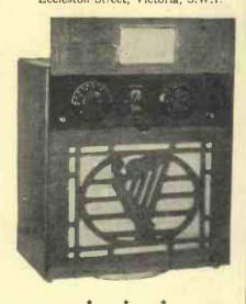
Beginners should note that a set with one screened-grid H.F. stage will be practically as good as one with two ordinary (three electrode) H.F. Stages
