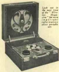
Adaptable for external aerial and earth. external loud-speaker, but for external batteries only if leads are lengthened.
