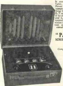
It consists of S.G. H.F. Valve, Det., 1 L.F., and 1 Power Valve. H.T. Consumption is very low and a long life is given from the L.T. ateach charge. Tuning is by drum control. Volume and Long and Short wave controls are fitted and provision is made for the operation of two loud-speakers simultaneously if desired.
