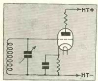
1.—Typical circuit for an anode-bend system for A.C. working
