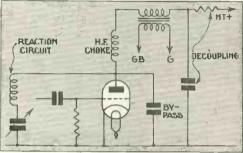
Fig. 8.—Transformer-coupled circuit with addition of high-frequency choke and anode by-pass condenser
