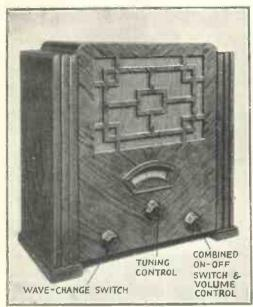
VERY MODERN APPEARANCE The modern design of the Futura cabinet is very striking. The tuning scale is calibrated in wave-lengths and the principal stations are marked
