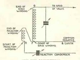
NEW COIL CONNECTIONS Fig. 7.—Note that the end of the reaction winding is connected to the start of the grid winding
