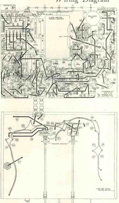
If desired a full-size blueprint can be obtained for half price, that is 9d., post free, if the coupon on the last page of the issue is used by December 31. When ordering ask for blueprint No. WM305. It should be noted that all the connecting wires are numbered separately in the best order of assembly; connect up in the proper numerical sequence and it will be impossible to make a mistake
