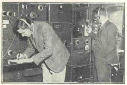
THE POST OFFICE MEASURES FREQUENCY At Dollis Hill, in north-west London, the Post Office owns a research station. This photo-graph shows part of the frequency-measuring equipment
