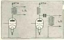
Fig. 2.—Output circuit for three-electrode valve, with and without a choke-condenser filter
