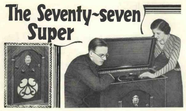
Here are details of an absolutely up-to-the-minute one-knob super-het radio gramophone for A.C. mains operation developed by the "Wireless Magazine" Technical Staff. It comprises seven valves with eight tuned circuits and under normal testing conditions has received over seventy foreign stations at good strength—in short, a set for the connoisseur!
