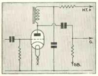
Fig. 5.—Choke-coupled detector circuit to avoid large drop in high-tension voltage
