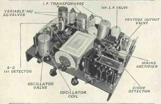
Here is the completed assembly of the Seventy-seven Super with all the valves and colls in position. The top of the baseboard is covered with metal foll
