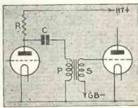
Fig. 2.—A high resistance substituted for the low-frequency choke of Fig. 1
