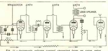
Fig. 11.—Automatic volume control operating from an extra valve controlled by the output circuit
