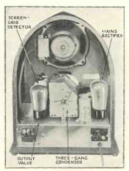
THE "WORKS" DISCLOSED A photograph showing the internal layout of the Bush A.C.3. Dry electrolytic condensers are used for mains smoothing
