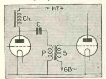
Fig. 1.—Valve anode circuit with ironcored low-frequency choke
