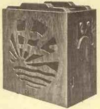
One of the most attractive sets on the market is the Pye model Q, a four-valve screen-grid battery receiver
