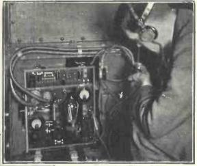
TESTING THE GEAR Marconi apparatus fitted in a Vickers-Armstrong tank. The wavelength used is between 7 and 8 metres
