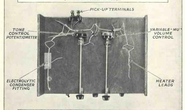
A view of the under side of the baseboard-chassis showing the potentiometers for radio volume control and for tone control. In this way long leads ore avoided
