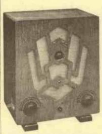
The Zetavox type ST seven-valve superhet receiver. It is housed in a bakelite cabinet
