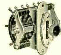
**Ganging Pattern Anti-Capacity Switch.** Prov. Pat. 28495/29. Embodies essential anti-capacity characteristics, but very compactly designed. Can be ganged. Fixed contacts moulded into bakelite arc, moving contacts of spring-temper Nickel Silver. Stocked 1- to 6-pole change-over but multi-pole sizes to order.
