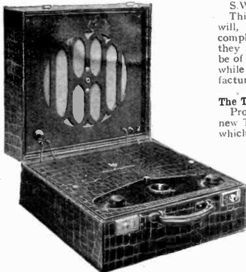
ROLLS-CAYDON.—The Rolls-Caydon "Ranger" portable receiver, which has two S.G. H.F. stages.
