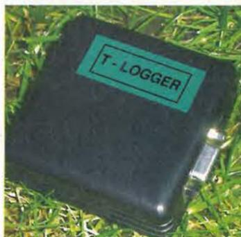
Small, simple and battery operated, this temperature logger wakes up from time to time to take a reading. When it's full, it connects to a PC for data uploading. See page 26.
