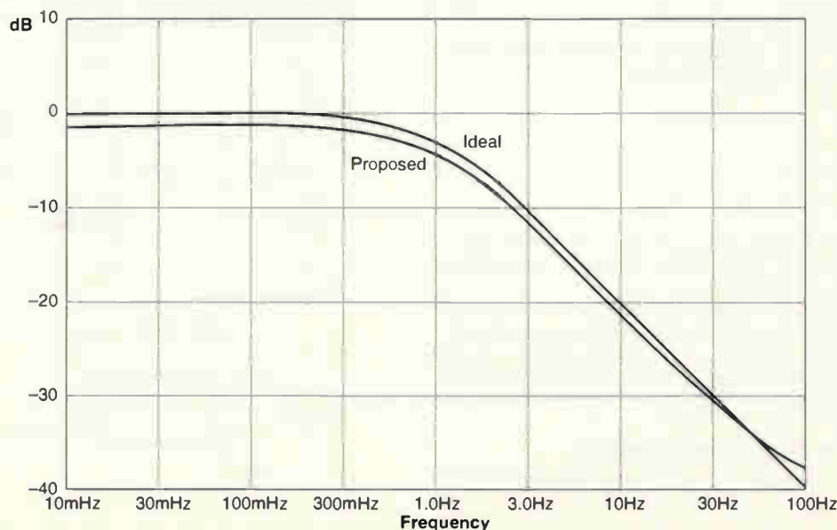
Fig. 9. Magnitude responses for an ideal RC filter and the one proposed in Fig. 8.
