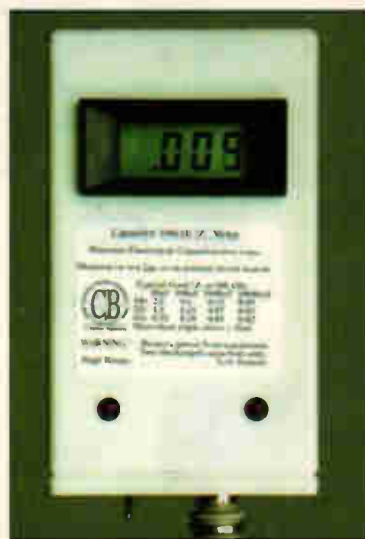
Capacitor guru Cyril Bateman has designed this 100kHz impedance meter with two ranges - 0-25Ω and 0-20kΩ. Read about it on page 473.
