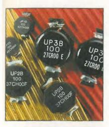
range of Uni-Pac surface mount inductors with the UP1B, UP2B, UP3B and UP4B with protective cases to reduce the risk of core breakage. They are for use within energy storage applications and DC/DC converters. Operating temperature is -40 to +85°C ambient with an rms current rating of 19.2 to 0.47A. Standard inductance is set at 0.47 to 100µH; modified values for higher applications are available on request. Cooper
