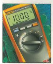
emit an audible tone to signal that a new minimum or maximum reading has been sensed and stored. Frequency. capacitance and resistance ranges are up to 100kHz. 10000 $\mu$ F and 50M $\Omega$ . Fluke Tel: 01207 9420700
