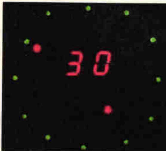
The speaking clock's face. Hours are indicated by the red LEDs while the seven-segment display shows minutes. Seconds are indicated in BCD using further red LEDs
