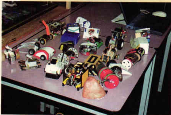
These ant-weight fighting robots took a trip to Hursley EMC recently to deal with some EMC difficulties. Creator and engineer Peter Waller had been having a few problems with interference and receiver saturation - the latter from up to six competing transmitters clustered around the tiny fighting arena. Solutions were: more suppression on his wheel motors and shorter receiver aerials. The robots pictured are: ANTcyclone, CombatANT and MilitANT. Each weighs under 150g and fits in a 100mm cube. The next ant-weight championship will be in Aylesbury in October. www.robotwars101.com for ant-weight rules.
