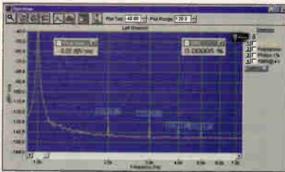
Figure 7: This now discontinued Philips extended foil/Polystyrene 1% axial lead capacitor, with 4 volt signals and 18 volt DC bias, shows negligible distortion. With test signals increased to 6 volt and DC bias to 30 volt second harmonic increased less than 4dB and distortion to 0.00007%. There was no visible intermodulation.
