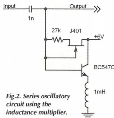
Fig.2. Series oscillatory circuit using the inductance multiplier.
