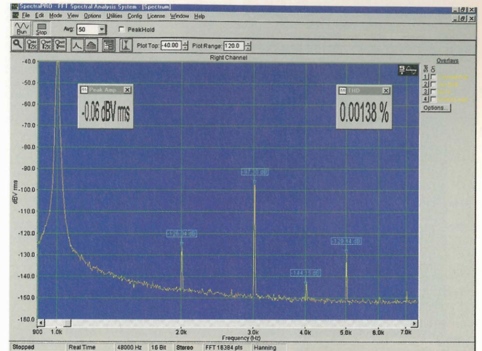
**Fig. 11.** This multi-turn cermet trimmer, set as a 5.6kΩ variable resistor and tested with a 6V signal from 1kΩ source impedance, generated this enormous -97dB third harmonic, 0.00138% harmonic distortion. Tested exactly the same a low cost carbon control produced 0.00129% while a conductive plastic control and 10-turn wirewound generated only 0.00009% and 0.00007%.
