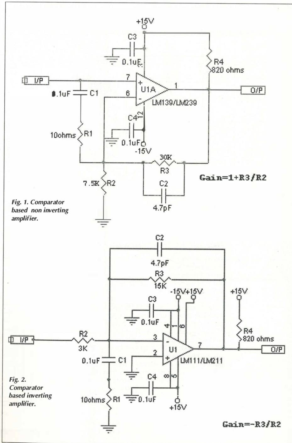
Fig. 1. Comparator based non inverting amplifier.
