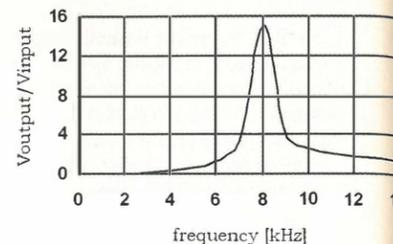
Fig.3. Frequency response of the oscillatory circuit.
