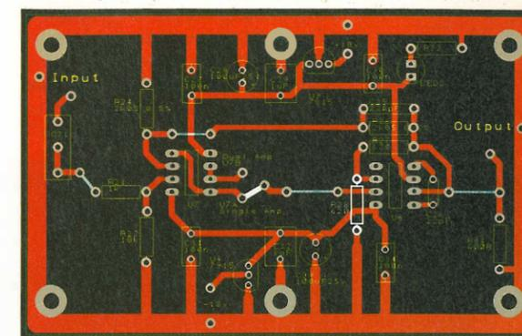
Fig. 3. The test PCB and component values used for this article. The link which changes from measuring the 'single' to 'dual' configurations is highlighted in white. Resistor R2B, highlighted in white, must be removed when using an NE5534AN or similar amplifier also the DIL header for U8. With a current feedback AD811AN for U8, resistor R2B is required, so should be refitted.
