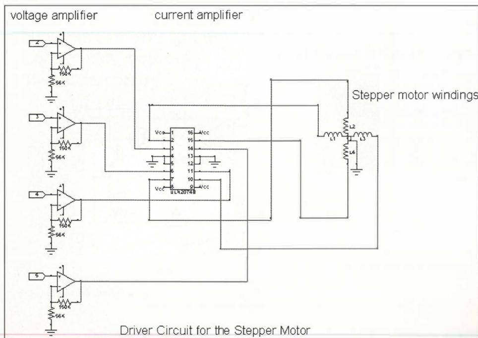
In the circuit shown below a 12V, 1.5A, 10kg - cm torque stepper motor is interfaced to the PC via its parallel port. This is done in order to automate the motion of the stepper motor. This circuit is mainly IC based which makes it easy for construction, has fewer components and is also cost effective.
