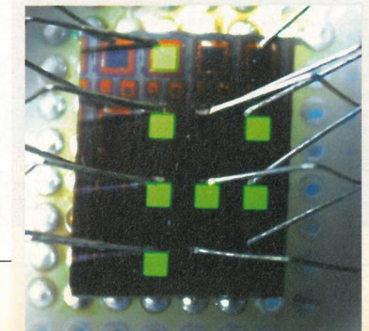
STMicroelectronics has produced light from silicon by doping with rare-earth materials. This is not new, many research teams have done it before but, unlike most attempts, ST's devices are easily visible - as Electronics World witnessed during a visit to the development labs in Catania, Sicily. The emitters have been used to construct working all-silicon opto-isolators.
