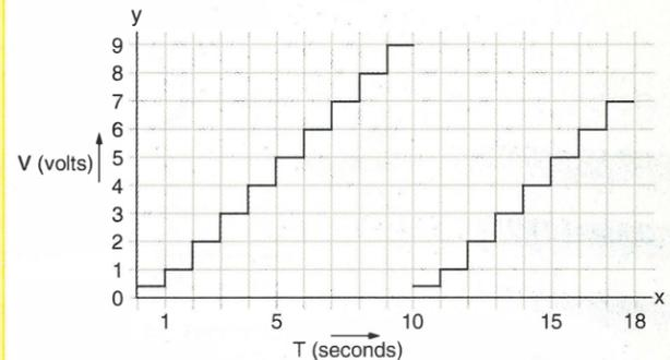
Output waveform when the circuit is used as a staircase generator.
