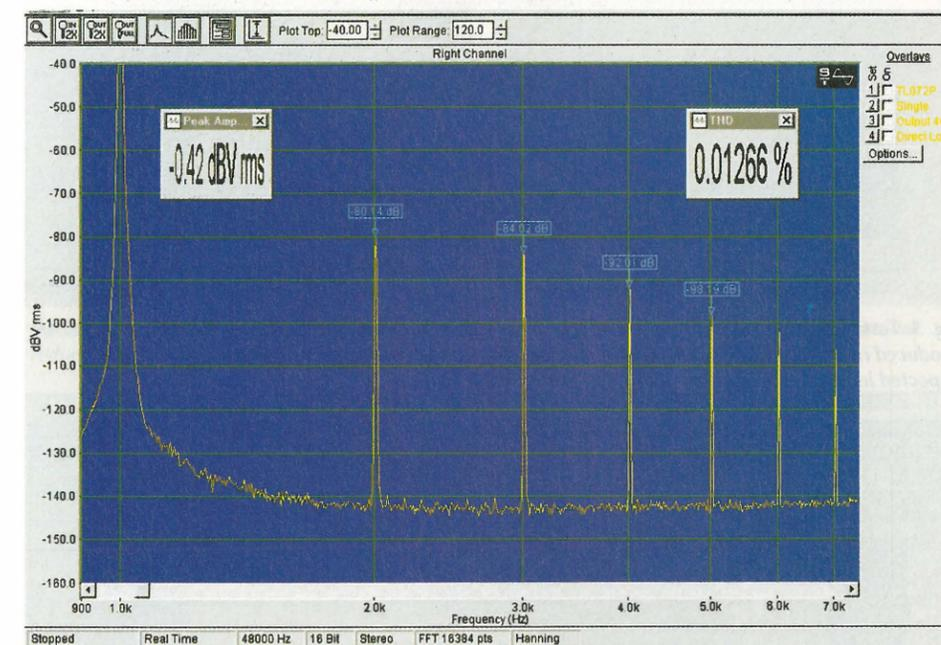
Fig. 4. Single amplifier distortion measured using the 'A' section of a TL072CP driving into my 575 $\Omega$  10.2nF test load. For this IC the 4V nominal test voltage had to be reduced to 3.8V.
