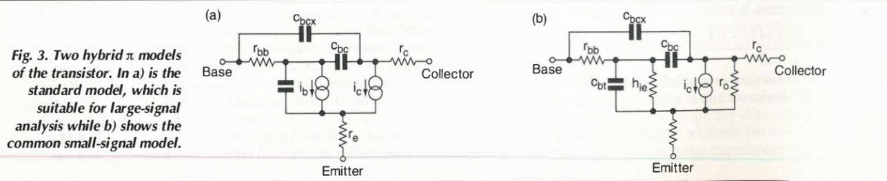
Fig. 3. Two hybrid  $\pi$  models of the transistor. In a) is the standard model, which is suitable for large-signal analysis while b) shows the common small-signal model.
