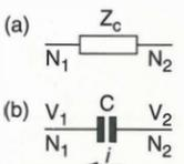
Fig. 2. Two views of a capacitor. Component (a) is for small-signal analysis while (b) is for transient analysis.
