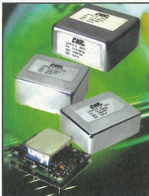
The device is designed to provide a holdover performance of better than 7µs over 24 hours in stable ambient conditions and a frequency stability better than 2 x 10<sup>-10</sup> peak-to-peak over an operating temperature range from -20 to +70°C. Package size is 51.0 x 41.0 x 19.0mm.
