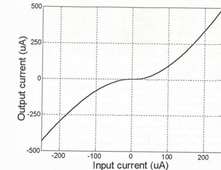
Fig. 4. Transfer function of the isolator.
