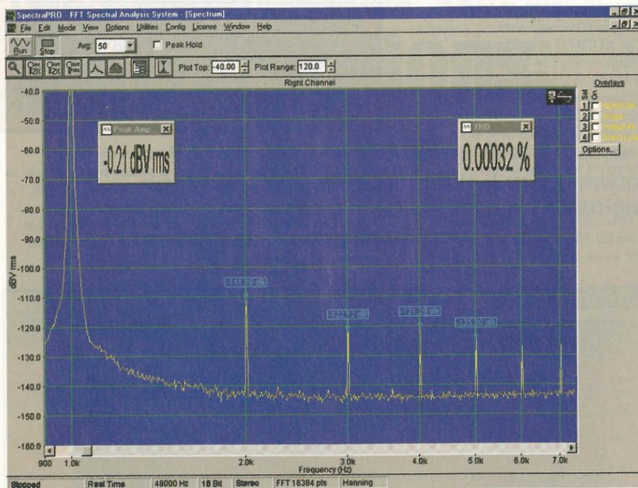
**Fig. 5.** Tested at 4V output, but otherwise exactly as Figure 4, this 'single' amplifier test of an NE5532AN produced remarkably little distortion driving this difficult test load, a heavier load than would be expected in any real world circuit or interconnect cable loading.
