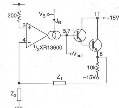
Using a transconductance op-amp, one simple circuit can act as a voltage-controlled resistance, capacitance or inductance.
