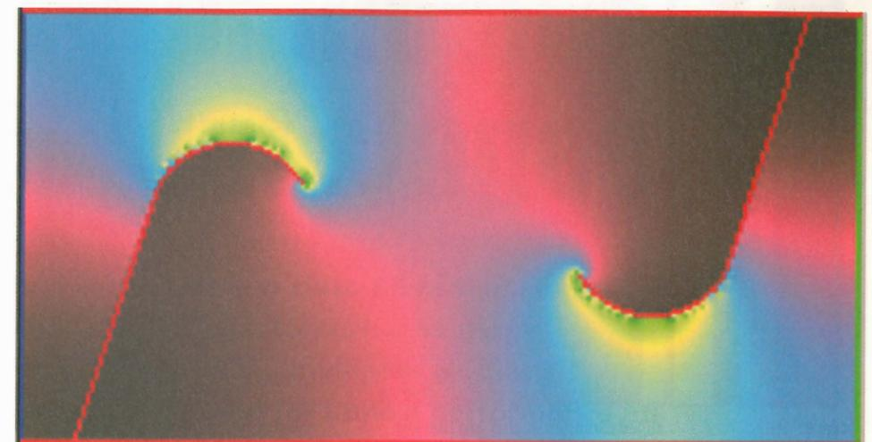
Fig. 6. Gradient plot of an improved trim method, a lazy-J serpentine trim.
