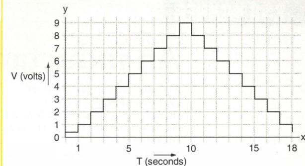
Output waveform when the circuit is used for producing a triangular waveform.
