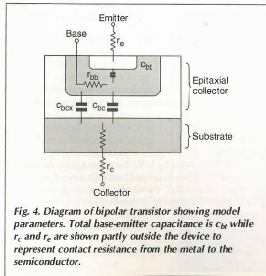
Fig. 4. Diagram of bipolar transistor showing model parameters. Total base-emitter capacitance is  $C_{bt}$  while  $r_c$  and  $r_e$  are shown partly outside the device to represent contact resistance from the metal to the semiconductor.
