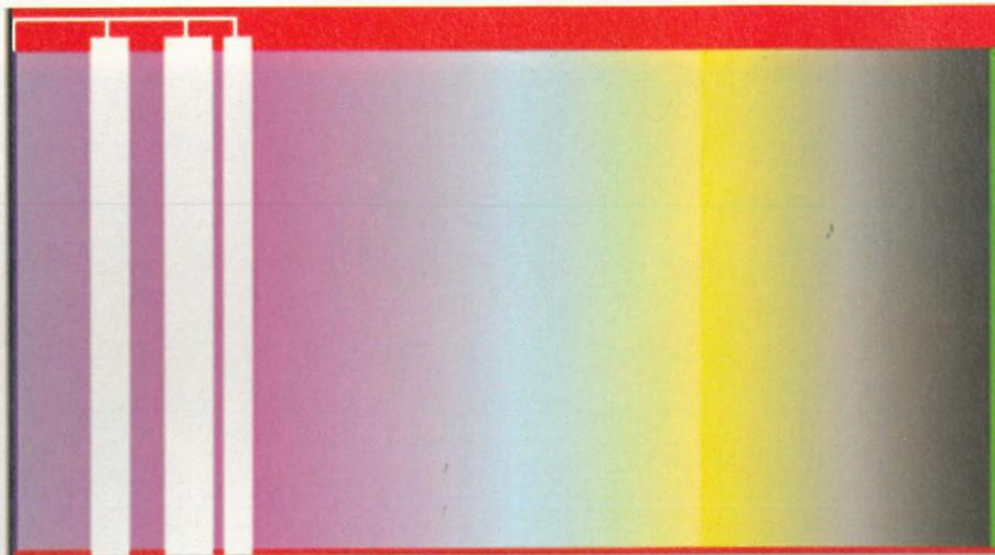
Fig. 8. Equipotential plot of the ultimate in stress-free trimmed resistors. The white strips are conductive material either over or under the resistive film.
