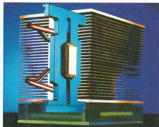
The photos show the microchannel heat collector attached to a mounting plate that connects the heat collector to the CPU. Fluid flows through the collector, back to a radiator that transfers heat to the air, then into a pump located below the radiator. The pump moves the fluid back through the microchannel heat collector, completing the sealed loop.
