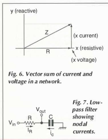
Fig. 6. Vector sum of current and voltage in a network.
