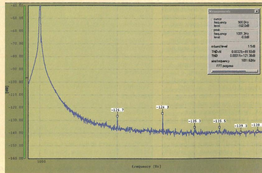
Fig 13. The Dr Jordan software, measuring a 511Ω resistor at 1V and 1kHz.
