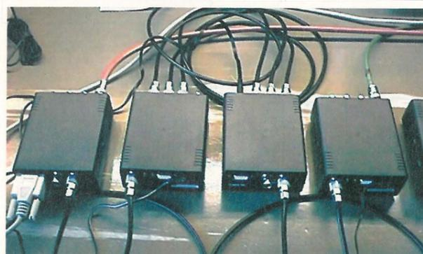
Cascaded operation of the encoders/decoders.
