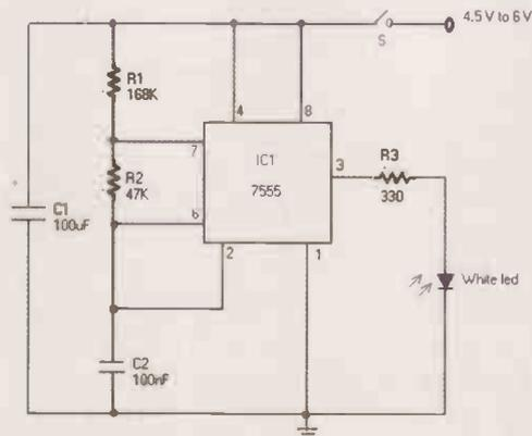
a traditional green LED is between 1.8V and 2.7V, a white LED has a higher forward voltage drop that lies between 3.1V and 4.0V depending upon the manufacturer. This means that whereas a green LED can be
