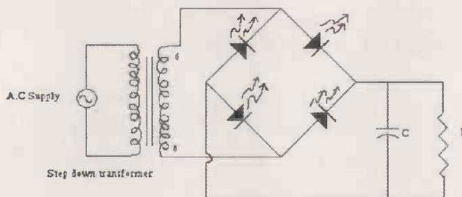
made of LEDs is connected to the output of a stepdown transformer and a load resistor is connected across the outputs. Rectification occurs as in an ordinary bridge but the ripple factor is found to be greater. In a bridge rectifier using ordinary
