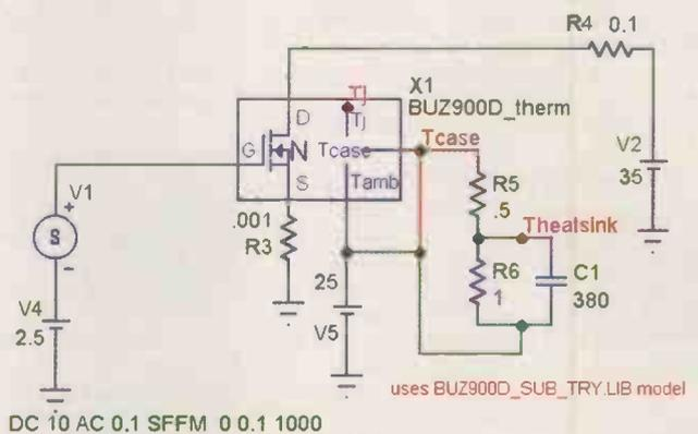
For DC set R4 to 0.001, V2 to 10v and V4 to 0v.
