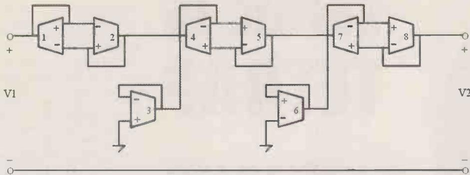
Figure 2: An OTA realisation of the ideal transformer in figure 1
