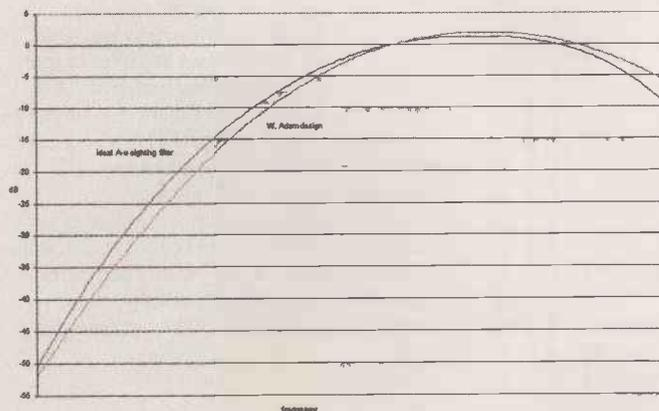
Fig. 4 PSpice simulation: Ideal A-weighting filter and W. Adam's design
