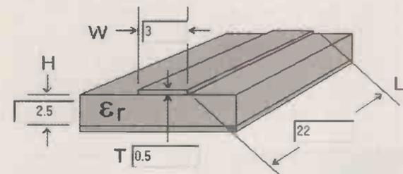
Figure 8: Layout of the  $\lambda/4$  Teflon transformer calculated using HP-AppCad  $\lambda/4$  transformation from 130 to 50 $\Omega$ . The transformer is realised using a Teflon plate (22x30mm) and a copper stripe with  $W=3\text{mm}$ ,  $Th=0.5\text{mm}$ , at the beginning of the Helix
