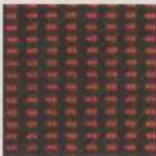
*A sub-Angstrom resolution image looking straight down on a silicon crystal. Each dumbbell-shaped row of atoms is 0.78Angstrom apart.*
