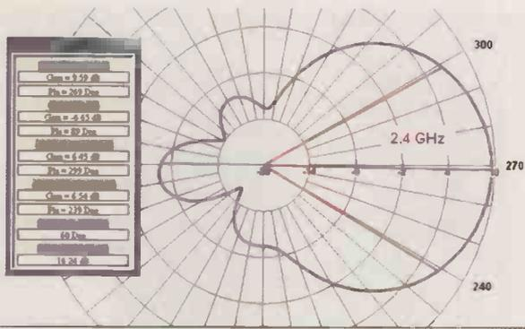
Figure 6: NEC-Win Pro simulated radiation diagram of the 1.7 turn conic 2.4GHz helix (pitch=20mm, conic dia. = 62/41mm)
