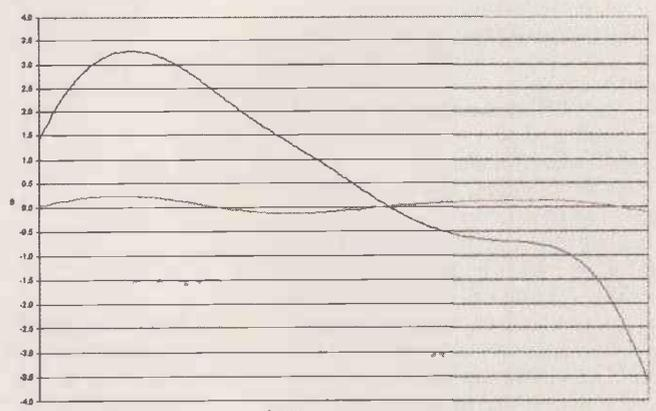
Fig. 5 PSpice simulation: Differences between the ideal A-weighting filter and W. Adam's original and improved filter design
