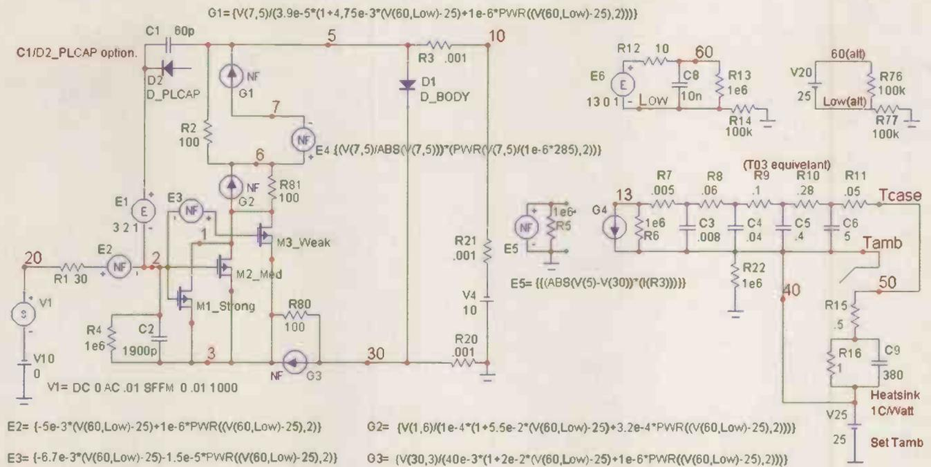
Figure 8: Having completed a model for the 'N' MosFet, the values used in the equations and the MosFet parameters were used to start the 'P' model development. However as can be seen in the figure, the polarity of a few components must be reversed and the three 'N' MosFet devices replaced with 'P' types. No changes are needed for the thermal control network.
