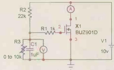
Figure 11: This simple test circuit allows direct measurement of drain current by gate voltage, for the critical subthreshold region that with three overlapping curves in the datasheet, was almost impossible to decipher.
