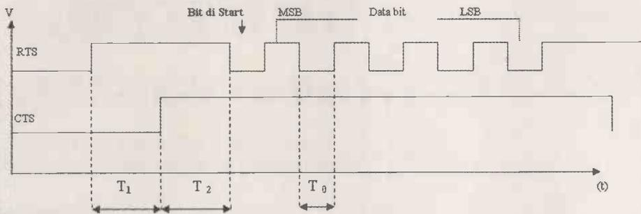
To develop a data transfer system, one often needs a data flow control between the transmitter and the receiver. The popular RS232 protocol is a simple mode to transfer data that has the RTS/CTS (Request To Send/Clear To Send) protocol as data flow control. This protocol needs 4 wires to link the two units. Here, I show that it is not generally necessary to have 4 wires, and that two wires can suffice to develop a data flow control. This is an advantage in the microcontroller system design.
