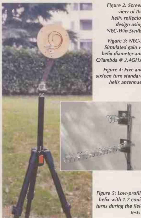
**Figure 5:** Low-profile helix with 1.7 conic turns during the field tests.
