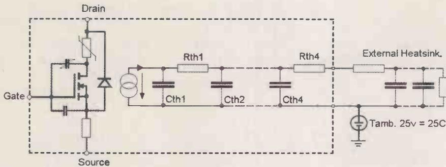
Figure 4: A heatsink model is easily attached to the R/C ladder network thermal model for a transistor. This figure illustrates the basic method used to calculate transistor junction temperature for this article.
