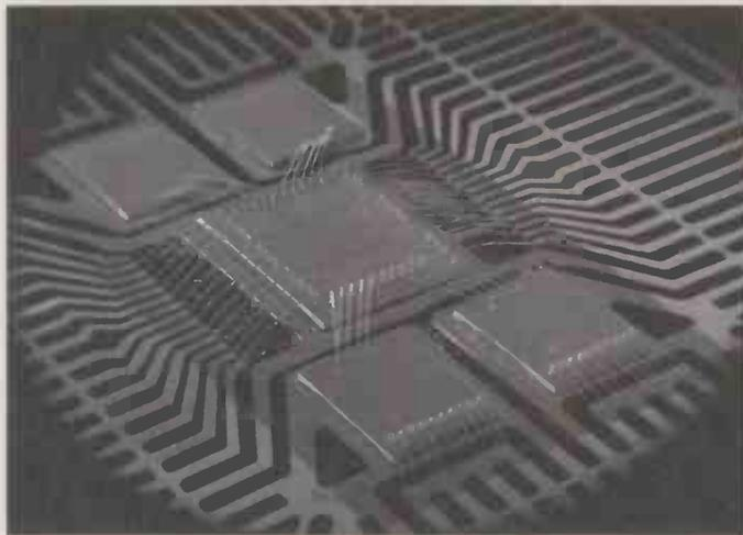
*In this experimental automotive load driver a central load controller operates four power mosfets, offering smart protection during faults.*
