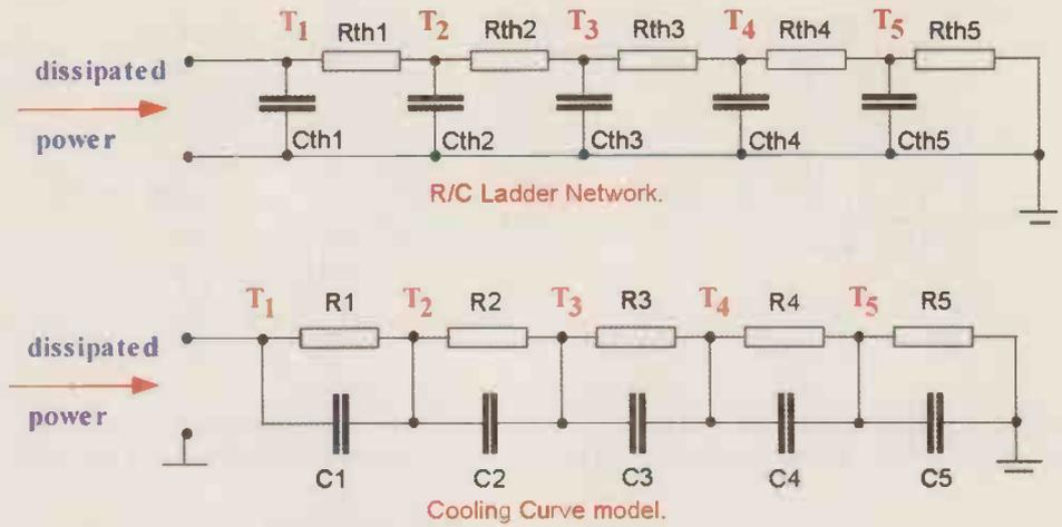
Figure 2: Two common circuits used to model the thermal transfer path in a transistor. Component values for the cooling curve circuit can be derived directly from a cooling curve measurement, favoured by semiconductor makers, unfortunately this circuit cannot easily be fitted with a heatsink. Component values for the R/C ladder network can be used unchanged together with established heatsink models.
