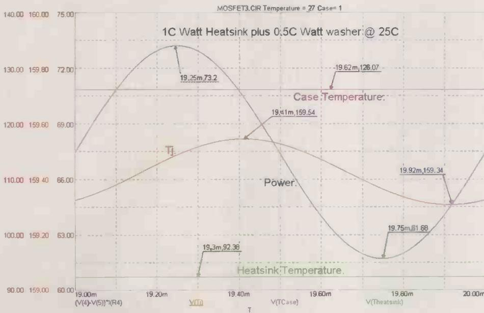
10) Removing the red link in figure 1 to now use the 1°C/watt heatsink and a mica washer, we see how dramatically the transistor junction and case temperatures increase. With much lower mean power dissipation of 67.5W, we see the junction temperature now exceeds the 150°C maximum rating for this device. The TO3 case temperature has risen to 126°C and the heatsink to a very hot 92°C.
