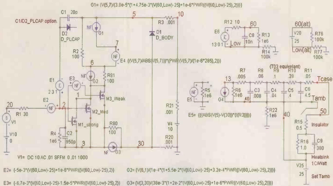
Figure 6 : My finished schematic model for the BUZ900/01D lateral power 'N' MosFet. This circuit works correctly as shown, used either with the C1 or the C1 diode model, chose one only deleting the other. Nodes 60 and Low control the models junction temperature. Move nodes 60 also Low to the alternate positions shown to fix the transistor junction temperature while developing the model. With nodes 60 and Low as shown the model is self-heating.
