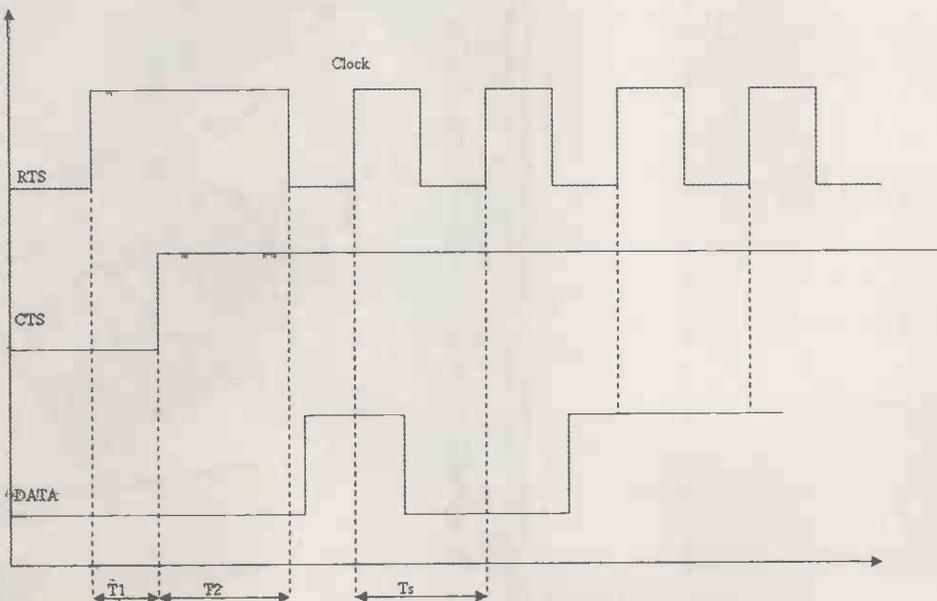
$T_1$  and  $T_2$  are the timeout and  $T_s$  is the sample time.
