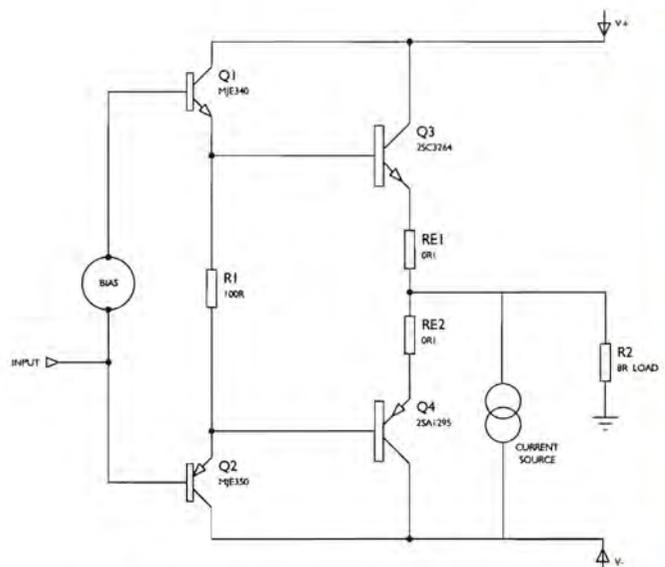
**Figure 6:** The concept of constant-current crossover displacement
