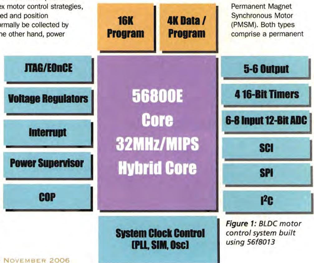
Figure 1: BLDC motor control system built using 56f8013
