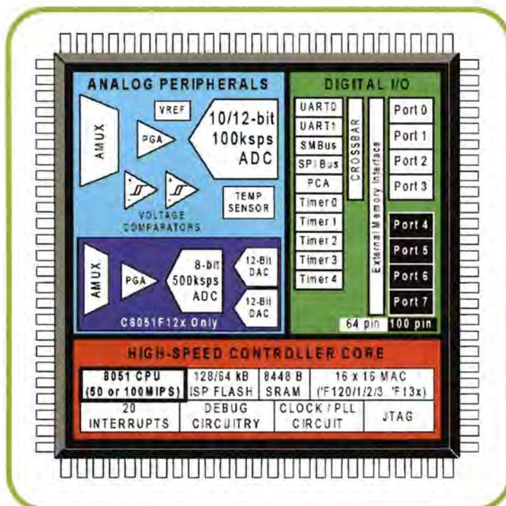
**Figure 1:** Block diagram of a modern microcontroller from SI Labs, featuring full JTAG IEEE Std 1149.1 compatible boundary-scan and embedded JTAG programmable flash memory [Diagram copyright SI Labs Inc.]
