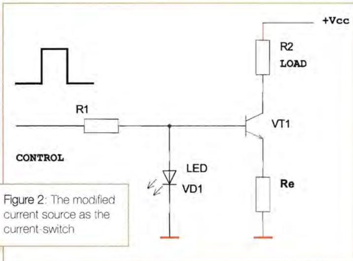
Figure 2: The modified current source as the current-switch
