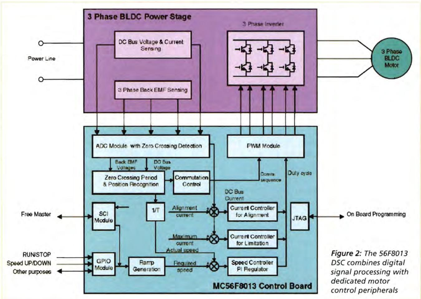
Figure 2: The 56F8013 DSC combines digital signal processing with dedicated motor control peripherals
