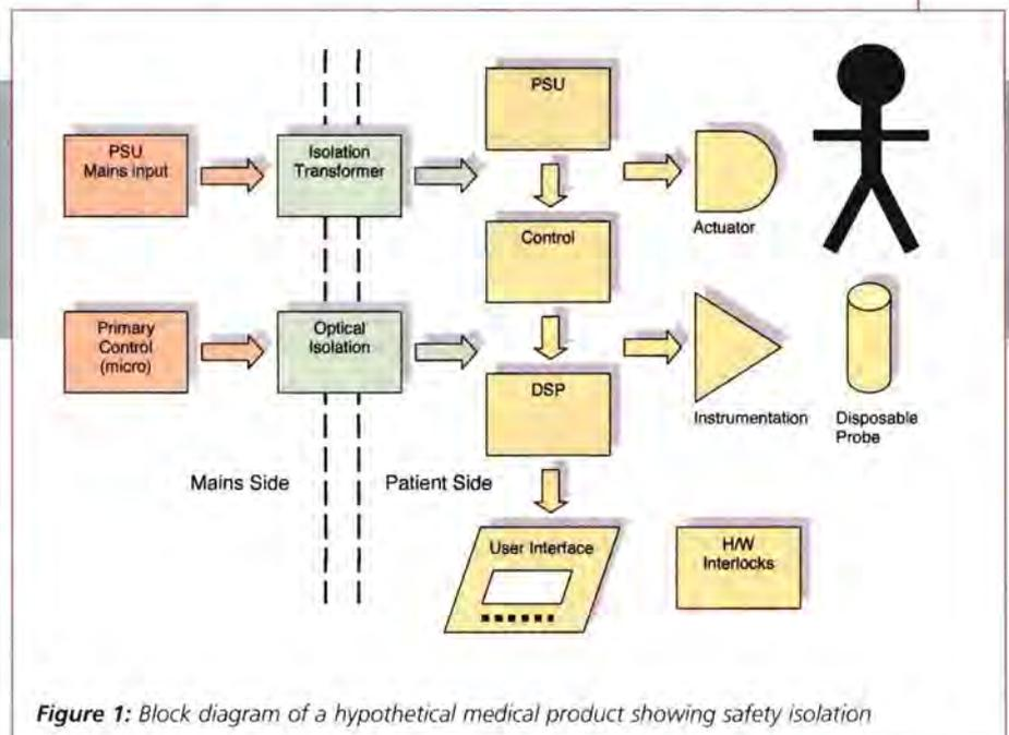
Figure 1: Block diagram of a hypothetical medical product showing safety isolation
