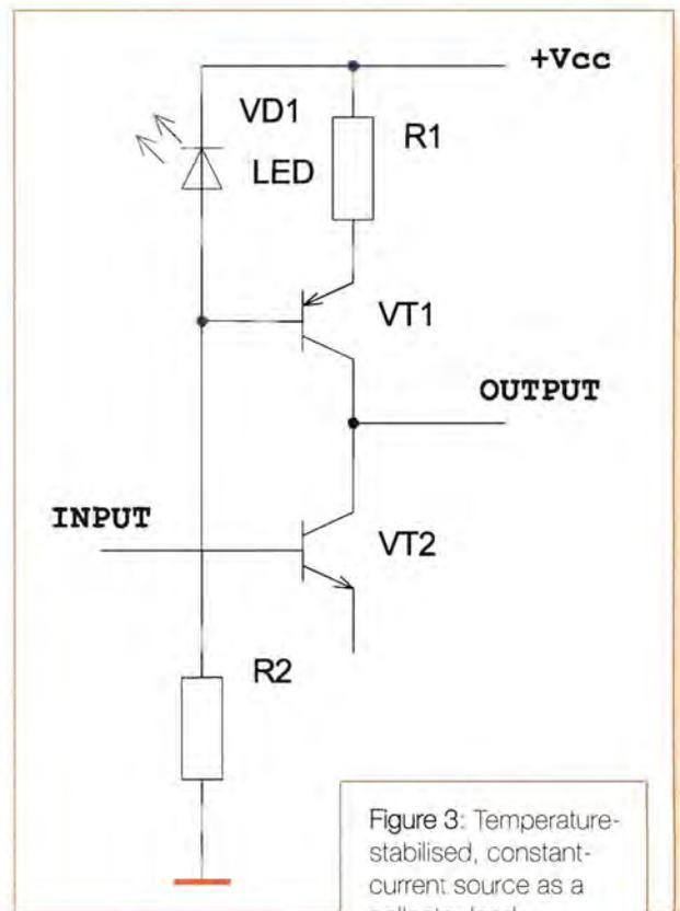
Figure 3: Temperature-stabilised, constant-current source as a collector load
