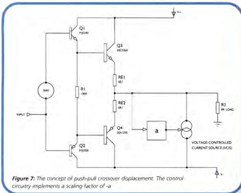
Figure 7: The concept of push-pull crossover displacement. The control circuitry implements a scaling factor of -a
