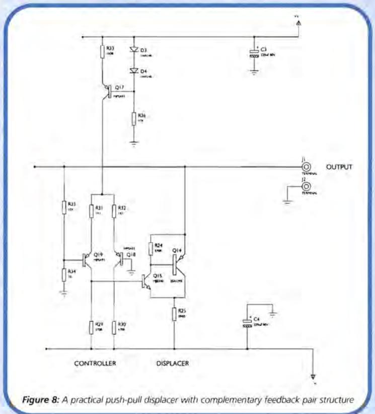
Figure 8: A practical push-pull displacer with complementary feedback pair structure
