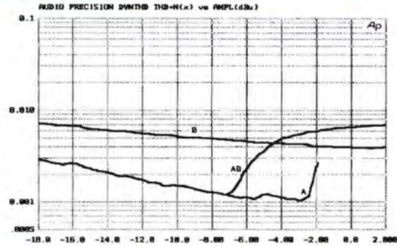
Figure 2: THD versus level for Classes B, A and AB. 0dB is 30W into 8Ω, so this graph runs from 500mW to 48W
