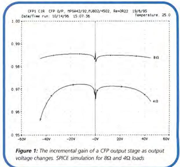
Figure 1: The incremental gain of a CFP output stage as output voltage changes. SPICE simulation for 8Ω and 4Ω loads
