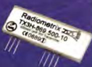
The TX3H-869-10 is a FM transmitter module with a power output of 450mW nominal. The module operates on European 869.40 - 869.65MHz sub-band allocation for 500mW and is designed for applications requiring operating range in excess of 3km or it can be used when space or ergonomic limitations dictate the use of small and inefficient antennas.
