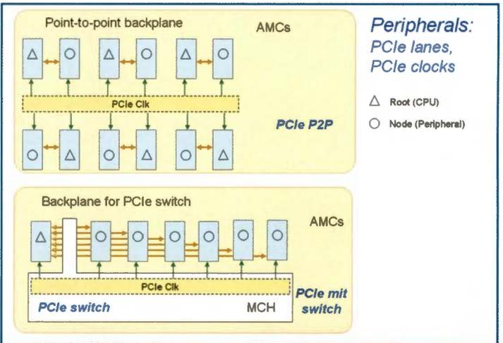
Figure 3: AMC port mapping and backplane
