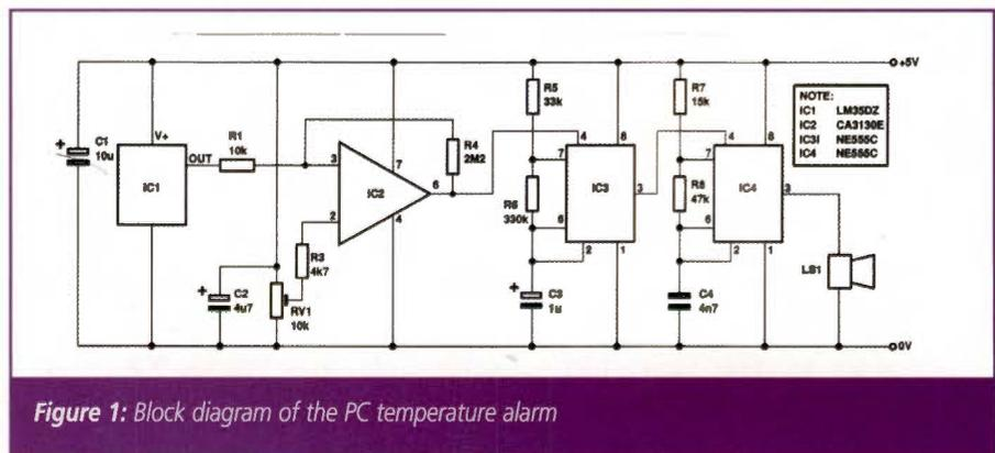
**Figure 1:** Block diagram of the PC temperature alarm
