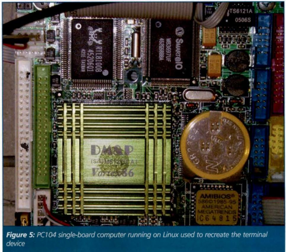
Figure 5: PC104 single-board computer running on Linux used to recreate the terminal device
