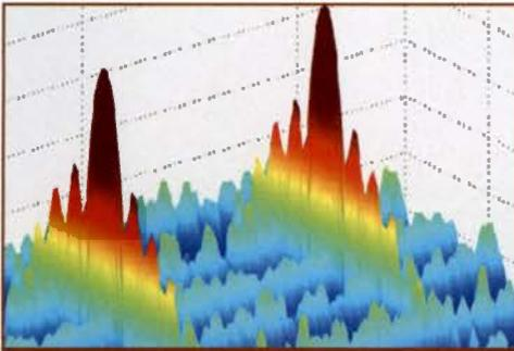
**Figure 2: The 3D capture of the cross-correlation function between a PRN code and the captured GPS signal (Z axis). The Doppler frequency shift and the code delay, representing a bi-dimensional acquisition search space, are reported on the Y and X axis respectively**
