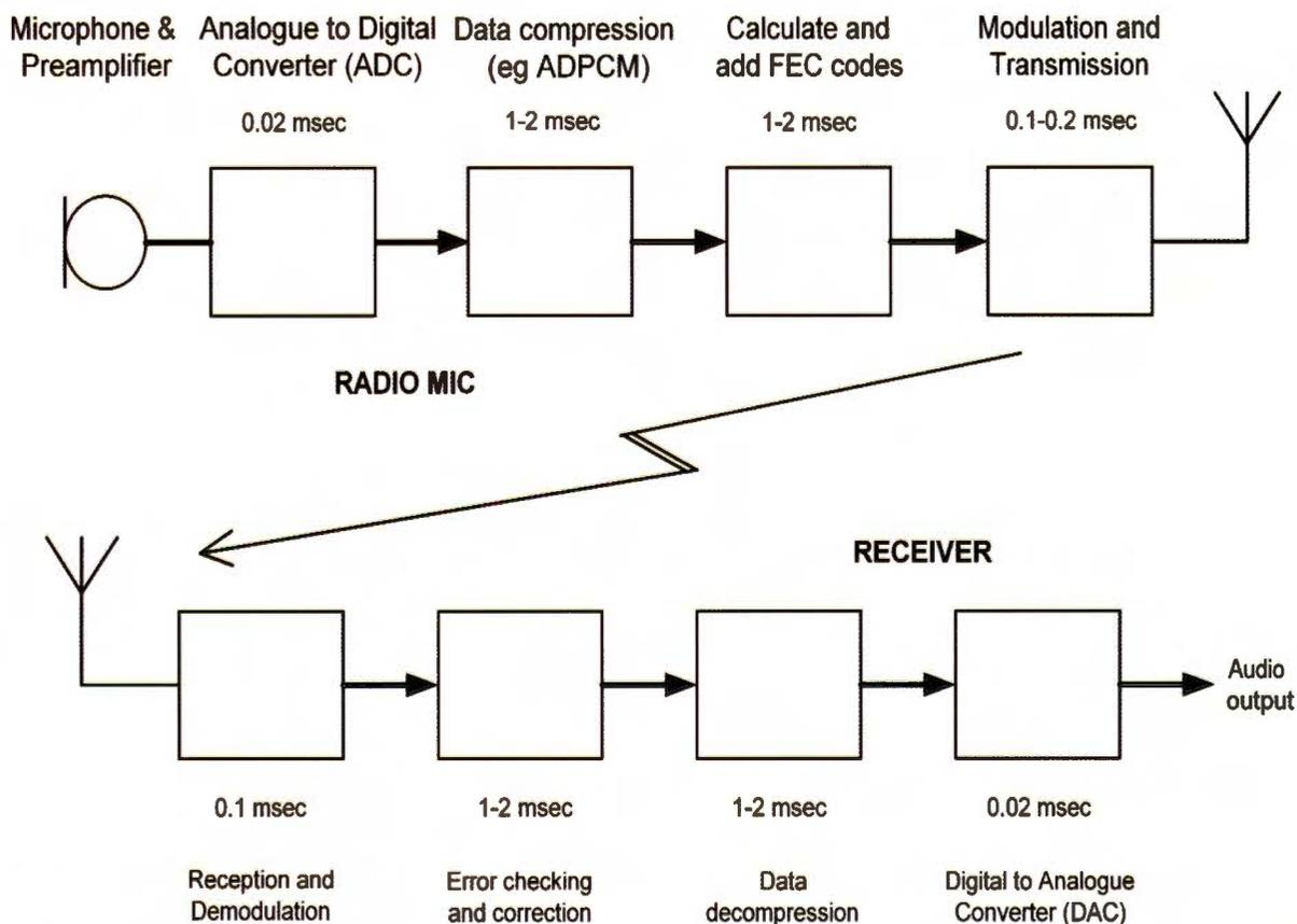
Figure 1: A simple digital radio microphone system
