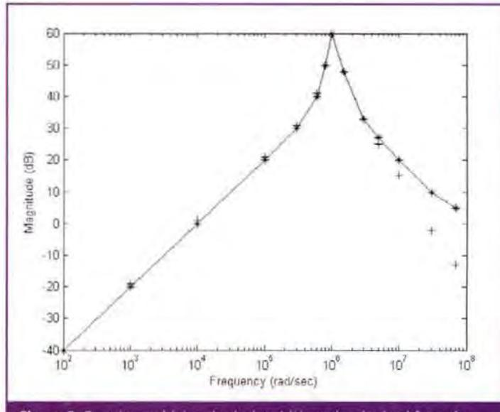
**Figure 3:** Experimental (+) and calculated (\*) results obtained from the bandpass realisation
