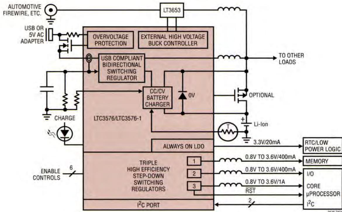
Figure 1: LTC3576 simplified block diagram
