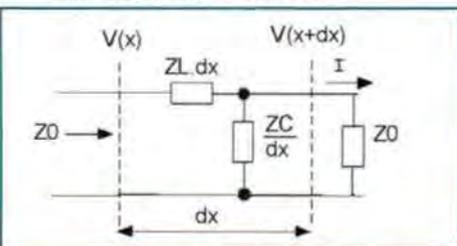
Figure 6: Lumped element model this time showing voltage and currents in line
