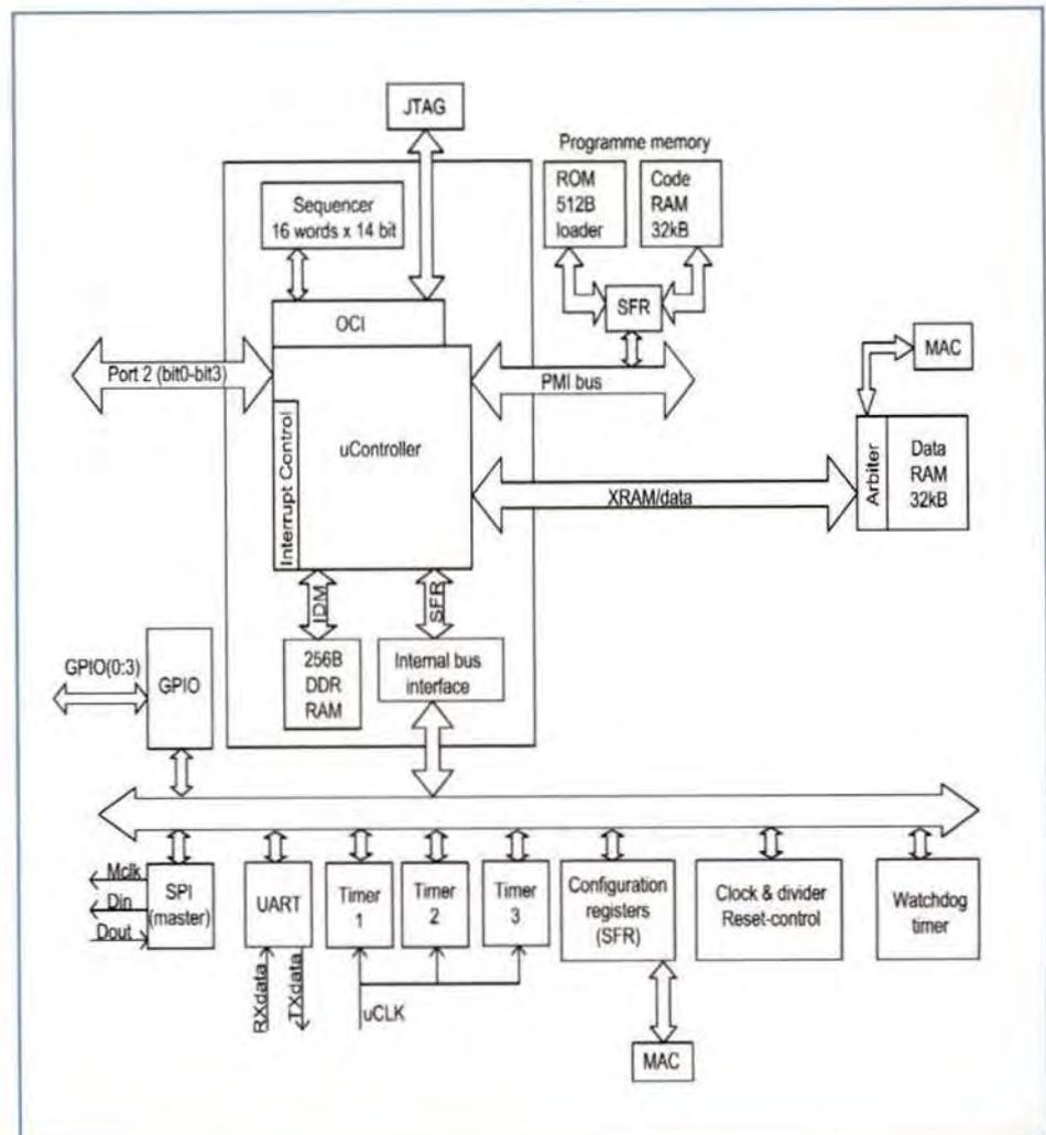
**Figure 1:** Block diagram of the digital section showing the microprocessor core, peripherals, memory and I/O structures
