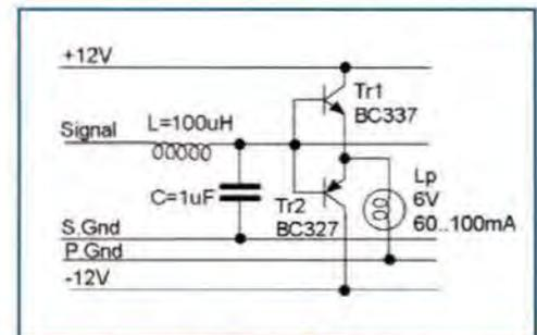
Figure 7: Line element of the model. There are 15 such sections.
