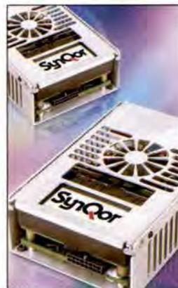
SynQor continues its entrance into the AC/DC marketplace with the introduction of the latest product designed specifically for medical applications. The AcuQor AQ0500M series of off line power supplies packs 500W of useable power into just 3.5" x 5.25" x 1.63", which is one of the the smallest cardiac care, medical grade AC/DC converter for this power level around.
