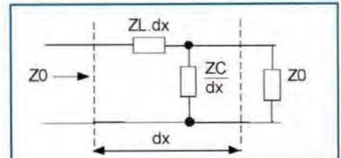
**Figure 5: Lumped element model of line showing impedances for the line section dx**
