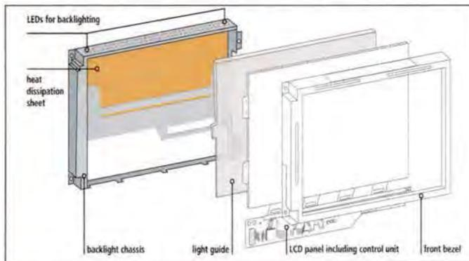
Sharp has launched an enhanced range of LED backlit liquid-crystal panels for industry applications. The portfolio now incorporates five displays in the screen diagonals of 3.5 to 15 inches.
