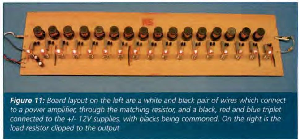
**Figure 11:** Board layout on the left are a white and black pair of wires which connect to a power amplifier, through the matching resistor, and a black, red and blue triplet connected to the  $\pm 12\text{V}$  supplies, with blacks being commoned. On the right is the load resistor clipped to the output
