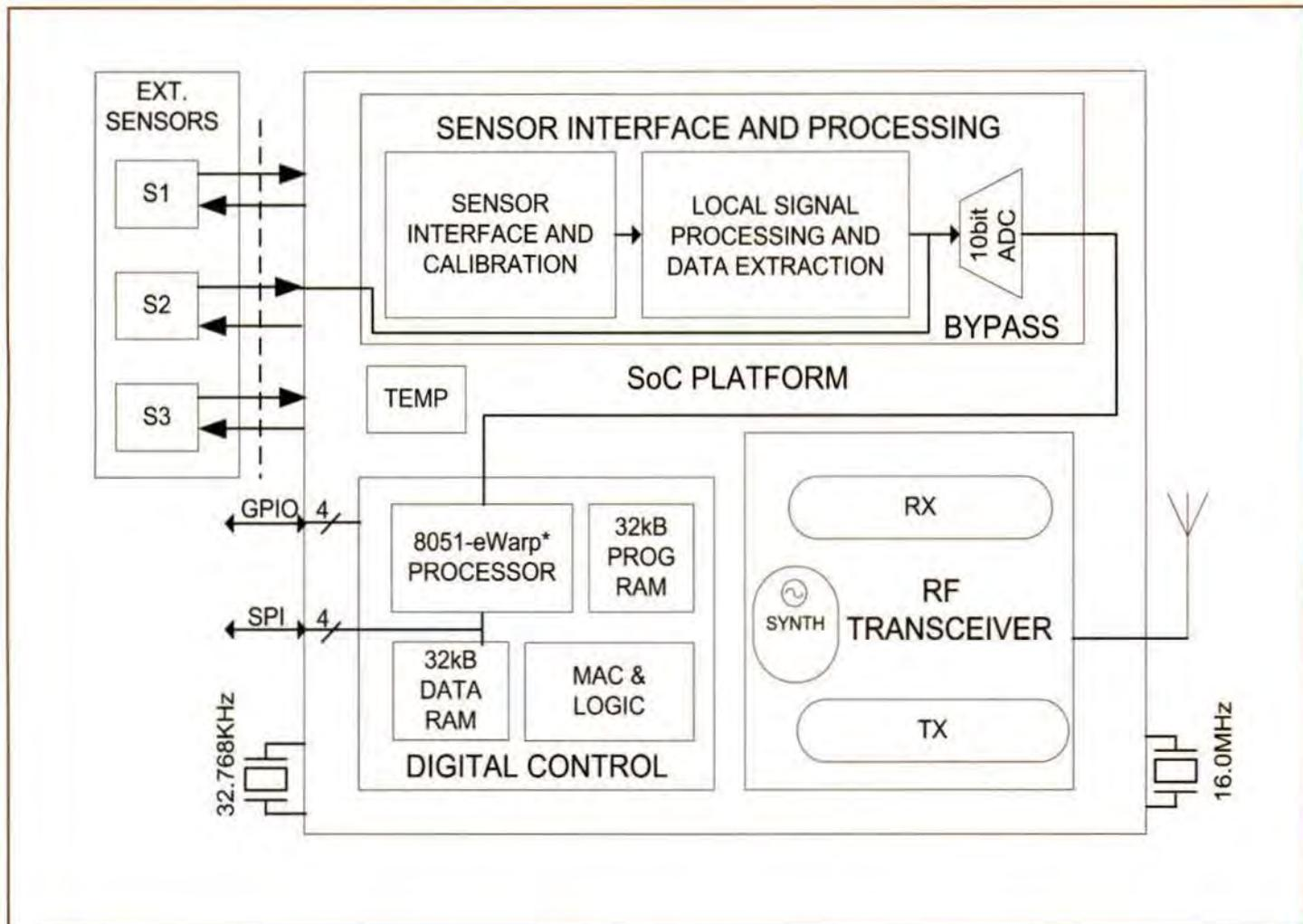
Figure 2: Block diagram of the Sensium SoC
