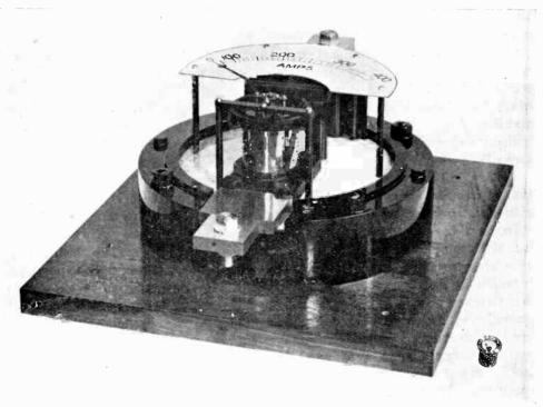
400-AMPERE TYPE WITH COVER REMOVED.
