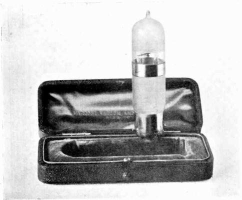
THE MARCONI VACUUM AMPERE GAUGE WITH ITS LEATHER CASE.
