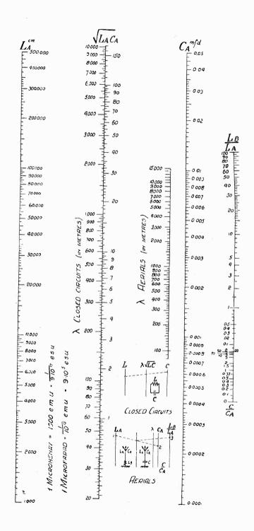
The use is the same when instead of a condenser there is a self-induction coil  $L_{\rm B}$ , but  $\frac{C}{C_{\star}}$  must be changed into  $\frac{L_{\rm B}}{L_{\star}}$ .
