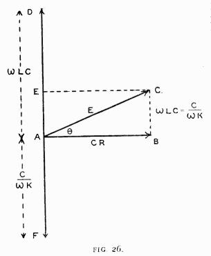
In the vector diagram, Fig. 26, let AB represent CR in phase with the current, ADequals  $\omega LC$ , 90° in advance of the current, and AF equals  $\frac{C}{\omega K}$ , 90° behind the current.
