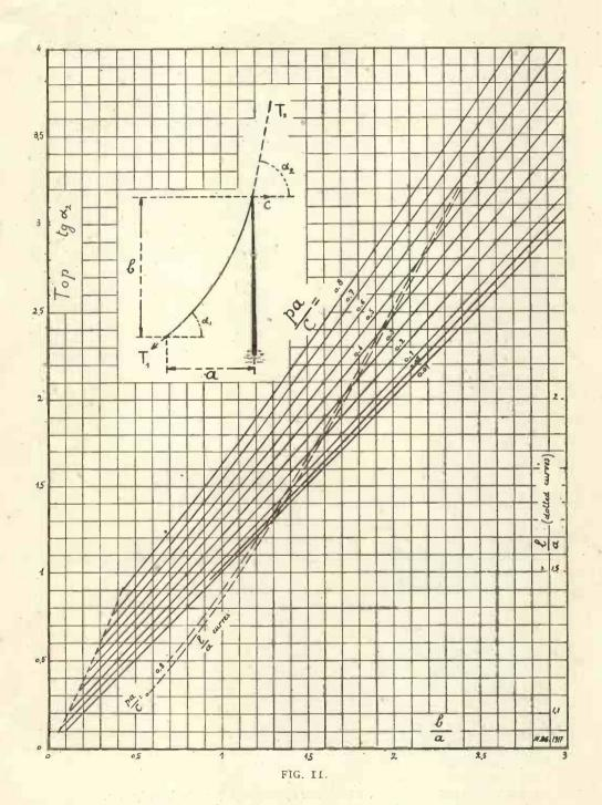
The section of the cable should be calculated (roughly and on the safe side) in order to support a strain  $T = \frac{c}{\cos \theta}$ .
