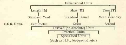
Force (continued).—The foregoing section on units was interpolated in order to clear the way to a fuller treatment of Force. The C.G.S. unit of Force has been referred to as the dyne, to explain which we must here introduce the ideas of Velocity and Acceleration.
