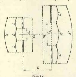
(September 10th, 1915). Tables are also given in the excellent book of Mr. W. H. Nottage.‡ When inductances having coupled flat coils are to be used, the reader may be referred to a paper of the author in *The Electrician*.§ Curves (Fig. 13) give the coupling coefficient in per cent. of two coaxial flat spiral coils (see Fig. 12).
