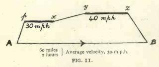
of a journey the velocity of a train will vary because the latter cannot start from a position of rest at its maximum velocity, and in order to stop (without being wrecked) it must gradually slow down. Fig. II represents graphically
