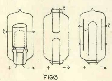
a current through the vacuous space between the insulated electrode and the hot filament. provided that the negative pole of the cell is connected to the negative side of the filament. If the connections of the cell are reversed. practically no current passes, the small amount of obtained current being due to
