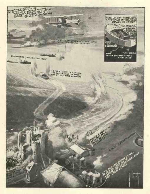
CREWLESS HUN BOAT LOADED WITH T.N.T. AND CONNECTED TO THE SHORE BY CABLE THROUGH WHICH IT IS ELECTRICALLY STEERED. THE COURSE IS SIGNALLED TO THE SHORE BY WIRELESS FROM A CONVOYING AEROPLANE.
