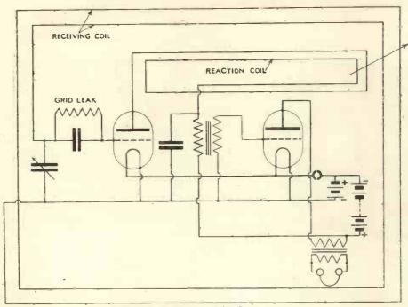
CONNECTIONS OF PORTABLE RECEIVER
