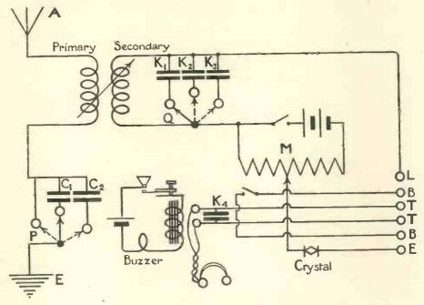
Fig. 29. Schematic wiring diagram of Tb Receiver.
