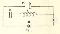
or other noble metal, C is a hard carbon contact, K a condenser, L an inductance, T an instrument which it is desired to operate by the battery B on closing the switch Pt. C. The battery charges the condenser, and when the switch closes the condenser discharges through the inductance and oscillations pass across the points Pt C and improves the contact at those points.
