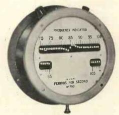
Fig. 6. Frequency Meter, as seen through stroboscope.
