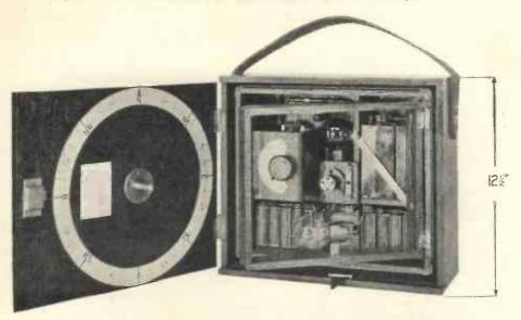
Fig. 1. Portable Receiver, showing pivot on detachable cover.
