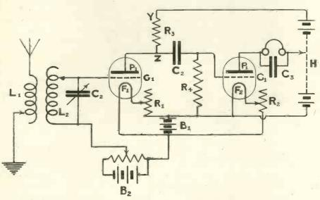
Fig. 15. Two-valve Resistance Amplifier
