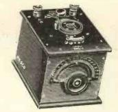
VARIOMETER. New efficient pattern with short wave switch, giving all control from 125 to 8,000 metres. Chart of approxi nate wave lengths sent with these. Welt made and fi.ted in mahogany case approx. 2 ins. × 5 ins. K ins. Insulation guarantee. Price 110/-
