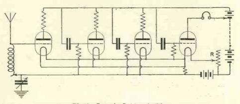
Fig. 16. Four-valve Resistance Amplifier.
