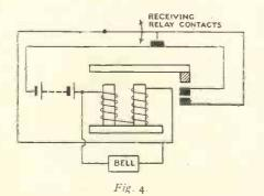
magnet, and so long as the latter is energised the bell will ring.
