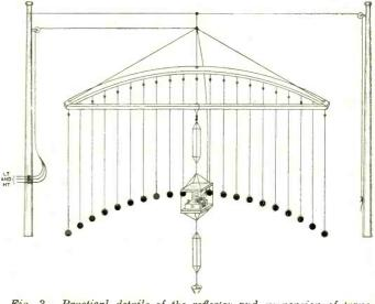
Fig. 3. Practical details of the reflector and suspension of transmitting apparatus and aerial.
