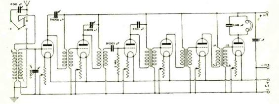
Fig. 1. "RADIO" (Mon.). The diagram gives the connections of a six-valve receiver with two H.F., rectifier and three L.F. valves. Tuned transformers are employed to couple the H.F. valves. No reaction is provided, and the circuit is suitable for the reception of broadcast transmissions.
