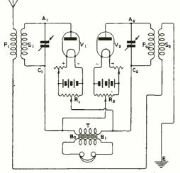
Fig. 5. Circuit arranged to eliminate interference.
