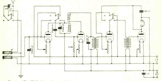
Fig. 4. "T.A.W." (Chingford). This is a diagram of a four-value receiver with H.F., detector and two stages of note magnification. The H.F. and the last note magnifier may be switched out of circuit when desired. The tuned anode method of H.F. amplification is used and the reaction coil is coupled with this circuit. The circuit is suitable for broadcast reception.
