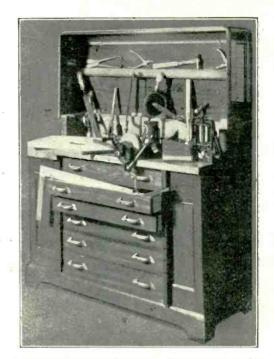
A fully equipped work cabinet. When not in use the back rack of this cabinet is arranged to close down over the table.
