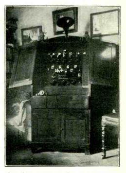
Our photo shows the five-valve receiver constructed by Mr. Arthur W. Botten, of "Red Cottage," Bourne End. By means of Dewar type switches, any combination of valves can be obtained. Compactness has been aimed at throughout, and the only visible wires are those to the 'phones or loud speaker.
