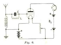
$\square$  I now come to the last of the three functions of the valve which I mentioned earlier, namely rectification. In Fig. 6 is shown a typical detector valve arrangement to assist in the explanation.
