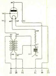
Fig. 7. Circuit of single valve amplifier unit.
