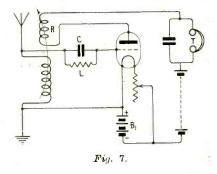
leak method of rectification. It is to be noted, however, that when this method is employed, actual signals in the telephone receivers are due to a *reduction* of anode current.
