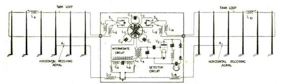
Fig. 9. Another and improved arrangement devised by Weagant.
