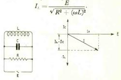
Fig. 66. Inductance capacity and resistance of R ohms in parallel. The vector relationship is shown. The current I is the total current from the supply.
