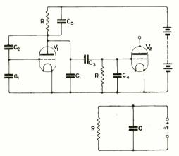
Fig. 56. Diagrammatic arrangement to show the capacities which shunt a resistance used in the anode circuit of a valve.
