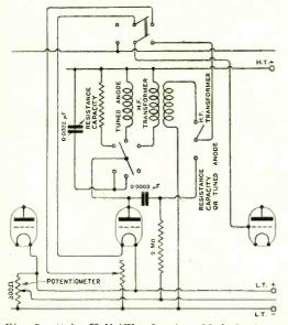
Fig. 5. "A. K." (Charlton). Method of connecting a switch so that the resistance-capacity, tuned anode, or transformer method of coupling may be used.
