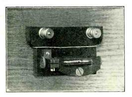
By courtesy of the Institution of Electrical Engineers. Detector used by Marconi to receive the first Transatlantic Signals (type invented by P. Castelli).
