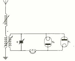
Fig. 6. Balanced valve circuit.
