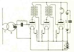
Fig. 8. Circuit of short wave receiver.
