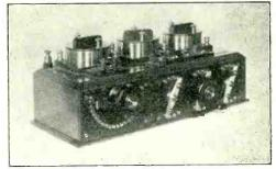
By courtesy Marconi's Wireless Telegraph Co., Ltd. An early Multiple Tuner.
