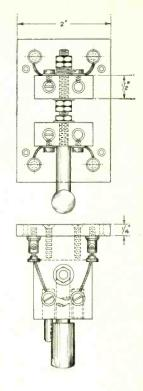
The writer strongly recommends the plug-in type of switches. They are easy to make, look neat, and have a further advantage in that temporary connections can easily be made to either the plugs or sockets, for the purpose of trying out new circuits, etc. The method of constructing these is shown in Fig. 5.
