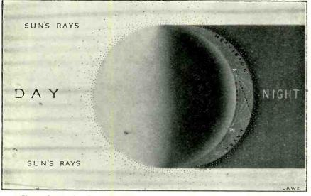
The earth, showing the action of the sun's rays in producing an electrified layer.
