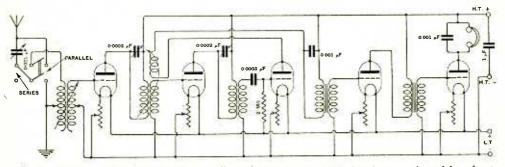
Fig. 5. "H.H." (Leyton, E.10). A five-value receiver suitable for the reception of broadcast transmissions with two H.F. (transformer coupled), rectifier, and two stages of note magnification.
