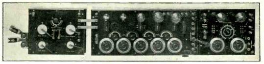
Fig. 2. The tuner, detector and amplifying units.
