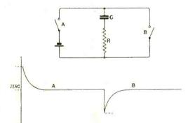
Fig. 58. Curves illustrating the charging and discharging of a condenser in a circuit as shown.
