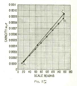
Having by this means made a determination of these stray capacities, they can be used to correct the measurements made at the ends of the curve in the manner that has already been described, since these stray capacities should be added to the true capacity of the comparison (fixed) condenser in each case, in order to obtain the true *effective* value of the condenser as used with the switch, etc., in their working positions.
