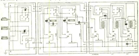
Fig. 1. "M.D." (Edinburgh). The figure gives the connection of three units. (1) Tuner with series-parallel and tune stand-by switches. (2) H.F. panel with two values coupled with tuned anode coil and grid condensers and leaks, with switches to disconnect them when required. (3) Detector and two L.F. connected values, with switches to cut out the note magnifiers when required.
