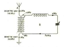
Fig. 10. Distribution of current and potential in receiving oscillatory circuits.
