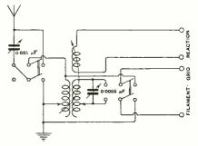
Fig. 4. " C.C." (Surrey). Showing the connections of a series-parallel, and a tune stand-by switch.
