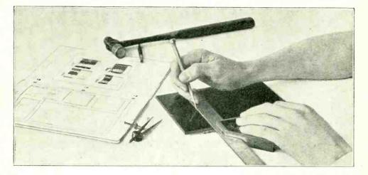
Photo: Radio and Model Engineering Using a scriber for setting out positions on the face of the panel as measured from one on the edges.
