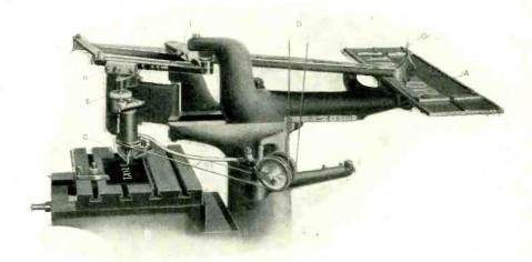
[By courtesy of Messrs. Taylor, Taylor and Hobson, Ltd.] The mechanism of the Engraving Machine, showing the pantograph action and the revolving cutter.
