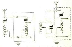
Figs. 3 and 4. Simple filter circuits joined with the receiver. The condenser may have a maximum value of 0.0005 mfds.
