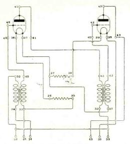
Fig. 10. Circuit of the 2-value L.F. amplifier unit.
