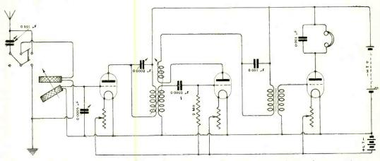
Fig. 3. "C.J.E." (London, W.C.1.) Connections of a three-valve receiver for broadcast reception— H.F., detector and L.F. The reaction coil is coupled with the H.F. transformer.
