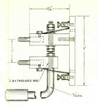
Fig. 4. Constructional details of the two-coil holder.
