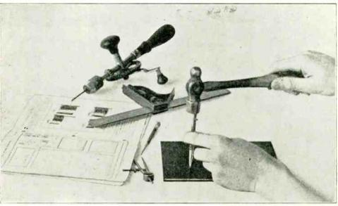
Photo: Radio and Model Engineering Centre punching the positions for the holes.
