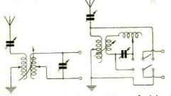
Fig. 2. A coupled circuit. Better selectivity is obtained by splitting the secondary coil. The coil which couples with the aerial circuit may be 3 ins. in diameter, with 10 turns. The other secondary coil may be 4 ins. in diameter and 3 ins. long of No. 22 D.C.C. with 10 taps.
