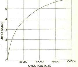
Fig. 57. Curve showing the amplification which may be expected when various anode resistances have various effective values.
