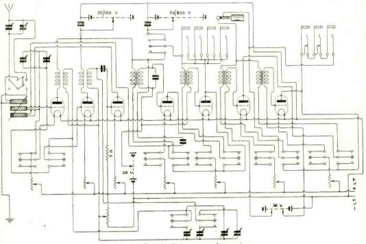
Fig. 4. Circuit of the seven-valve receiver.
