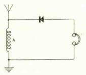
Fig. 2. A simple receiving circuit, which does not permit of selective tuning.
