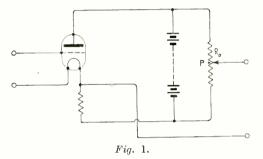
Referring to the circuit of Fig. 1, the principle will be seen. Instead of finding a point P with a resistance  $R_{in}$  at the same potential as the filament, we obtain it from a direct connection to the battery. In the case where a fraction of the voltage of a cell is required, this particular cell is shunted by a potentiometer of suitable value.
