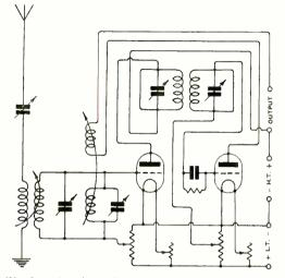
Fig. 12. Receiver with absorption circuit coupled to the reaction inductance for reducing interference.
