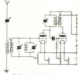
Fig. 13. Another circuit with rejector.
