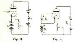
Under these circumstances the valve functions in a manner very similar to that of a non-return valve in a water-pipe system. Impulses applied in one direction are allowed to pass, whilst all those applied in the reverse direction are stopped.
