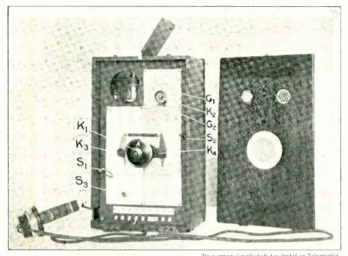
By courtesy Gesellschaft fur drahtlose Telegraphie. Fig. 2. The Tuner. It is adjusted to the correct wavelength when installed, though limited tuning is permitted and is effected by the single knob seen in the centre.
