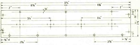
Dimensional drawing of panel for four-value holders.
