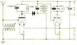
Fig. 6. "SIRKIT" (Lancs.). The first value operates as a H.F. amplifier, the crystal rectifies and the second value is a note magnifier.
