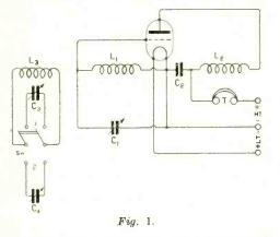
both the known condenser  $C_3$  and the new test condenser  $C_4$  are shown as variable condensers, since in this case the *known* condenser  $C_3$  is the variable condenser which has already been calibrated, and for which the calibration curve has already been plotted out. The test condenser  $C_4$  is now the new variable condenser, which it is desired to measure up so that a calibration curve can be plotted.
