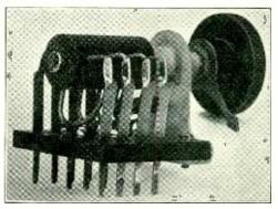
One of the many types of multi-contact switch suitable for varying the circuit arrangements of receivers.
