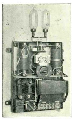
By courtesy, Gesellschaft für drahtlose Telegrarhie. Fig. 11. A pparatus for deriving L.T. and H.T. from direct current mains.
