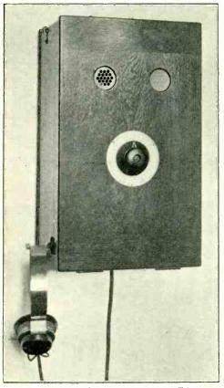
By courtesy Gesellschaft für drahtlose Telegraphic. Fig. 3. Removing the telephone from the switchhook throws the receiver into operation. One of the gratings can be removed so that the reaction coupling may be increased within limits for the reception of C.W. telegraphy.
