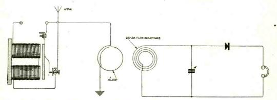
Fig. 13. Method of energising the aerial in order that the natural wavelength may be measured by the calibrated receiving circuit.
