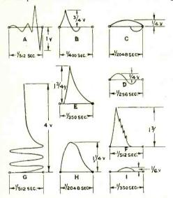
Fig. 2. Curves representing the wave shape of atmospherics.
