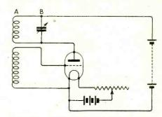
Fig. 11. Reacting value for reducing the effective resistance of the grid circuit.
