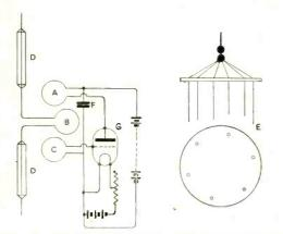
Fig. 2. Circuit of transmitter and arrangement of aerial.
