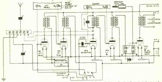
Fig. 1. Circuit diagram of the Receiver, which should be carefully studied in order that the principles may be thoroughly understood, before commencing to adjust and tune-in.
