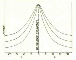
The figure illustrates a number of resonance curves showing how the selectivity of a circuit is improved with a high ratio of inductance to capacity. The upper curve corresponds with a low ratio of L to C, and the lower curve with a high ratio of L to C. It will be noticed, that for a given % change in the frequency, the amplitude of the current is reduced most in the lower curve—which corresponds with the circuit having the largest ratio of L to C.
