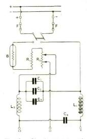
Fig. 12. Circuit arrangement for deriving H.T. and L.T. from D.C. mains.
