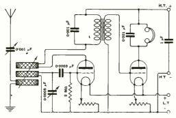
Fig. 2. " A.C.P.'' (Bruton). A two-valve receiver —rectifier and note magnifier.
