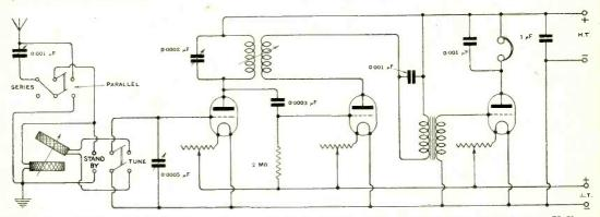
Fig. 6. "K.H." (S. Devon). This is a diagram of a three-value Broadcast receiver using one H.F., rectifier, and one L.F. values. All values are given. The reaction coil is coupled with the tunea ancde coil.
