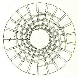
The accompanying sketch illustrates a novel method of winding a basket coil. As usual, an odd number of pegs or slots is used, but the wire is passed round two pegs at a time. The result is a basket coil of duolateral formation which possibly still further reduces the self-capacity. E.J.H.
