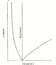
The curve shows the variation in current taken from the supply when the applied frequency is varied. At resonance the current is negligible, that is the circuit has a high impedance. To the left of the resonance point a larger portion of current flows through the inductance; to the right the condenser carries a larger current.
