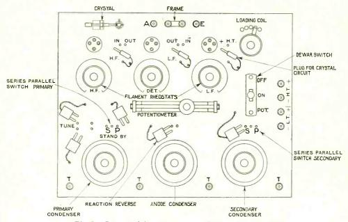
Fig. 3. Lay-out of the components on the face of the panel
