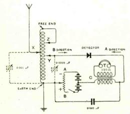
Fig. 15. Experimental Crystal Receiving Circuit.
