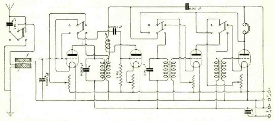
Fig. 5. "SIRKIT" (Lancs.). Connections of a four-valve receiver with H.F., rectifier and two note magnifiers. Switches are connected to cut out valves when required.
