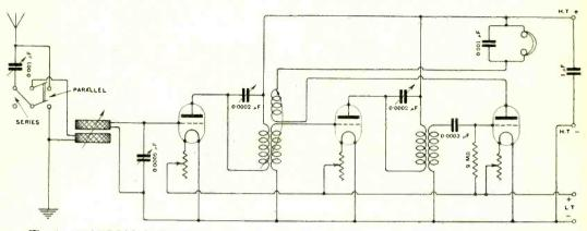
Fig. 3. "AERIAL" (Rugby). Diagram of a three-valve receiver suitable for the reception of broadcast transmissions. There are two H.F. transformer coupled valves and a rectifier. The reaction coil is coupled with the first H.F. transformer.
