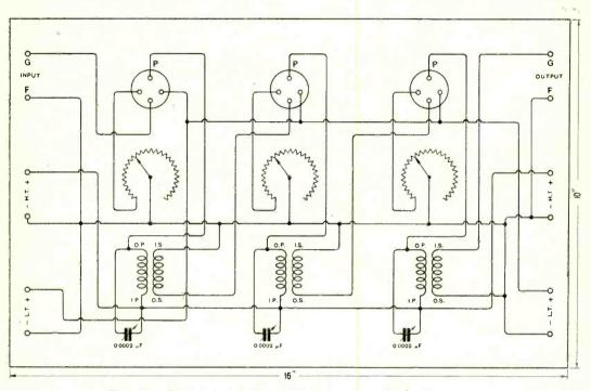
Fig. 5. " P.R.B." (Godalming). Panel with three H.F. valves.
