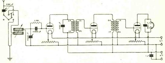
Fig. 2. "Nutty" (Sheffield). Here we have a three-value receiver—the first value operates as a rectifier, and the others as note magnifiers.
