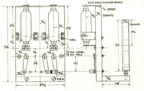
Fig. 10. Dimensions for setting out the H.F. valve punel.
