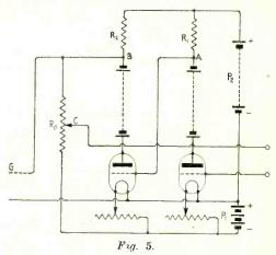
In order to eliminate the effect of selfinduction, it is well to introduce a further stage for the output; for example, in Fig. 5, G represents the grid of the output stage whose plate and filament circuits can also be supplied from the main batteries,  $P_1$  and  $P_2$ .
