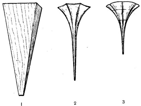
Fig. 2. Loud-speaker horns used for experimental comparison.
