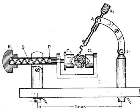
Fig. 1. Experimental Crystal Detector of French design.
