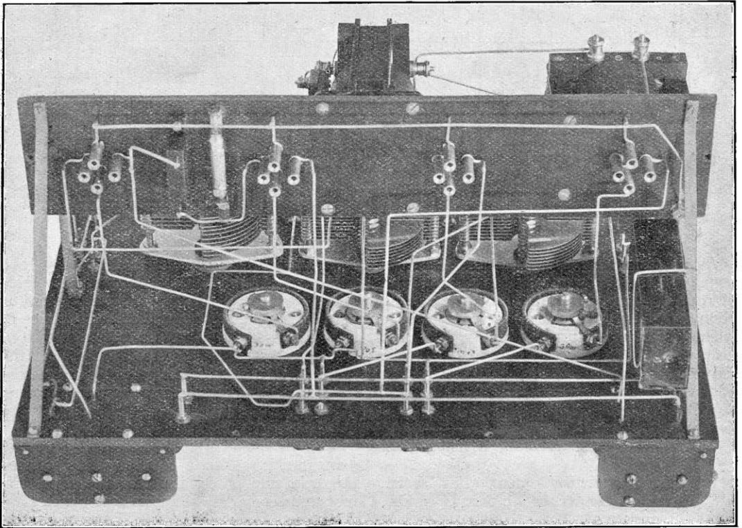
*Rear view of the panel showing the method of fixing the valve platform.*
