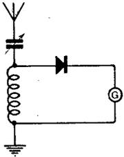
Fig. 1. This circuit gave 5° deflection on the galvanometer.
