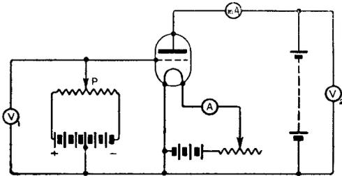
Fig. 1. Circuit for plotting grid voltage—*anode current characteristic. The potential applied to the grid is varied by means of the potentiometer P and indicated by the voltmeter  $V_1$  while the plate current is read off on the milliammeter mA. Filament current and plate voltage remain constant.*
