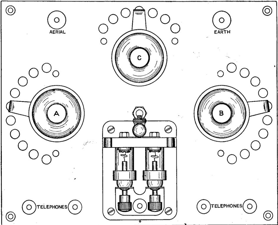
Fig. 1. Plan showing arrangement of components on top of panel.
