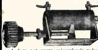
**PLUNGER RHEOSTAT ONE-HOLE FIXING.** A unique type of Rheostat and Potentiometer. The Rheostat is capable of exceedingly fine adjustment, contact is perfectly smooth, and does not cause microphonic noises, it occupies a very small space on panels. Finished, Nickel Plated.
