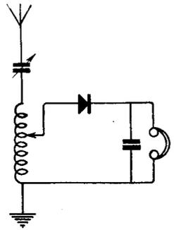
Fig. 5. A series condenser tuning circuit in which the load effect of the detector can be varied.
