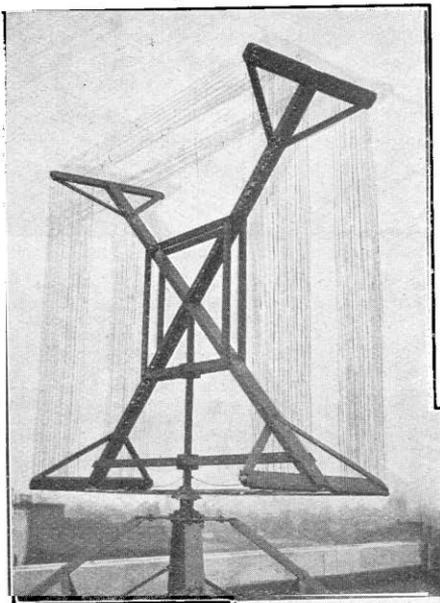
*The aerial can be rotated in any direction by a control wheel in the instrument room. The possibility of screening is entirely absent.*
