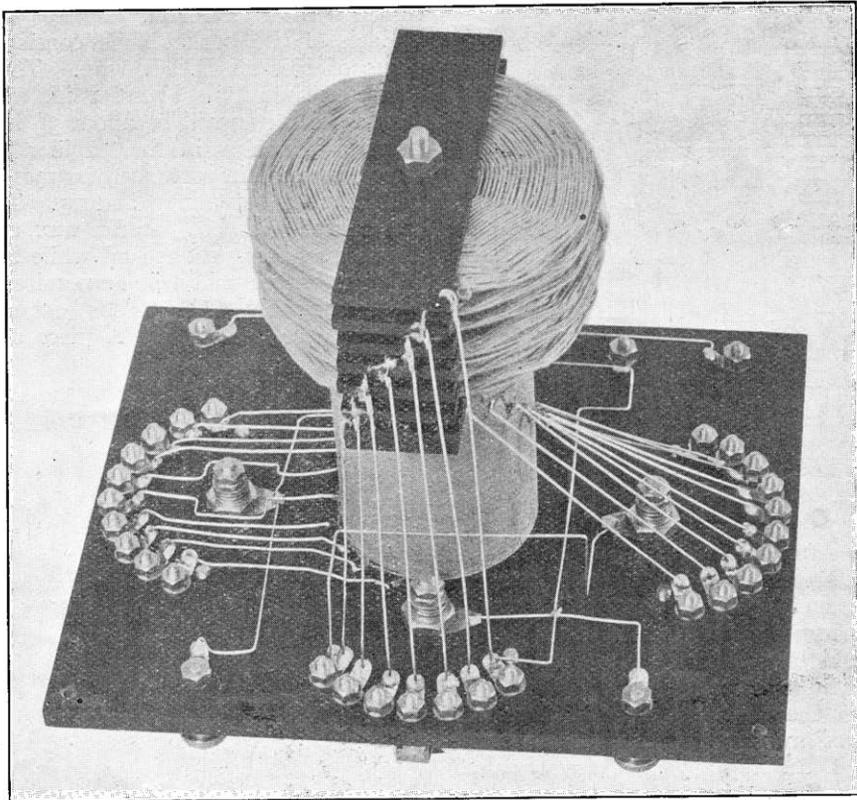
Fig. 5. View underneath the panel. Soldering tags are used under all terminals and switch contacts.
