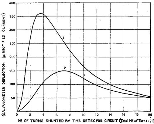
Fig. 4. Curve showing the reduction of the maximum signal intensity when the effective resistance of the aerial is increased.
