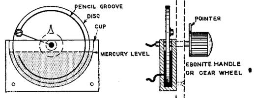
This groove is lightly rubbed round several times with a lead pencil. The centre of the disc works on an axis which is mounted in a bearing and allows the bottom of the disc to dip into a cup containing mercury. The necessary connections are taken from the mercury and from one end of the pencilled groove.
