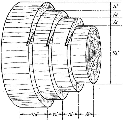
Former for shaping the turns for the several layers.
