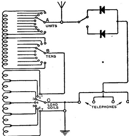
Fig. 3. The connections of the receiver.
