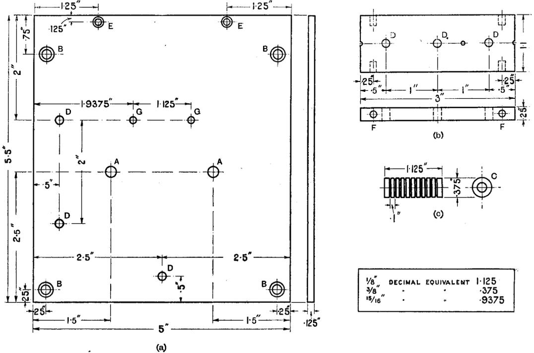
Fig. 1. Component parts of the inductance unit. Decimal dimensions are shown for uniformity and fractional equivalents are given. Sizes of holes : A, Drill 7/32" dia.; B, Drill 3/16" dia. and countersunk on topside for No. 3 B.A. screws ; C, Tapped No. 3 B.A. ; D, Drill 5/32" dia. ; E, Drill 1/8" dia. and countersunk on topside for No. 6 B.A. screws ; F, Tapped No. 6 B.A. x 3/16" deep ; G, Tapped No. 4 B.A.
