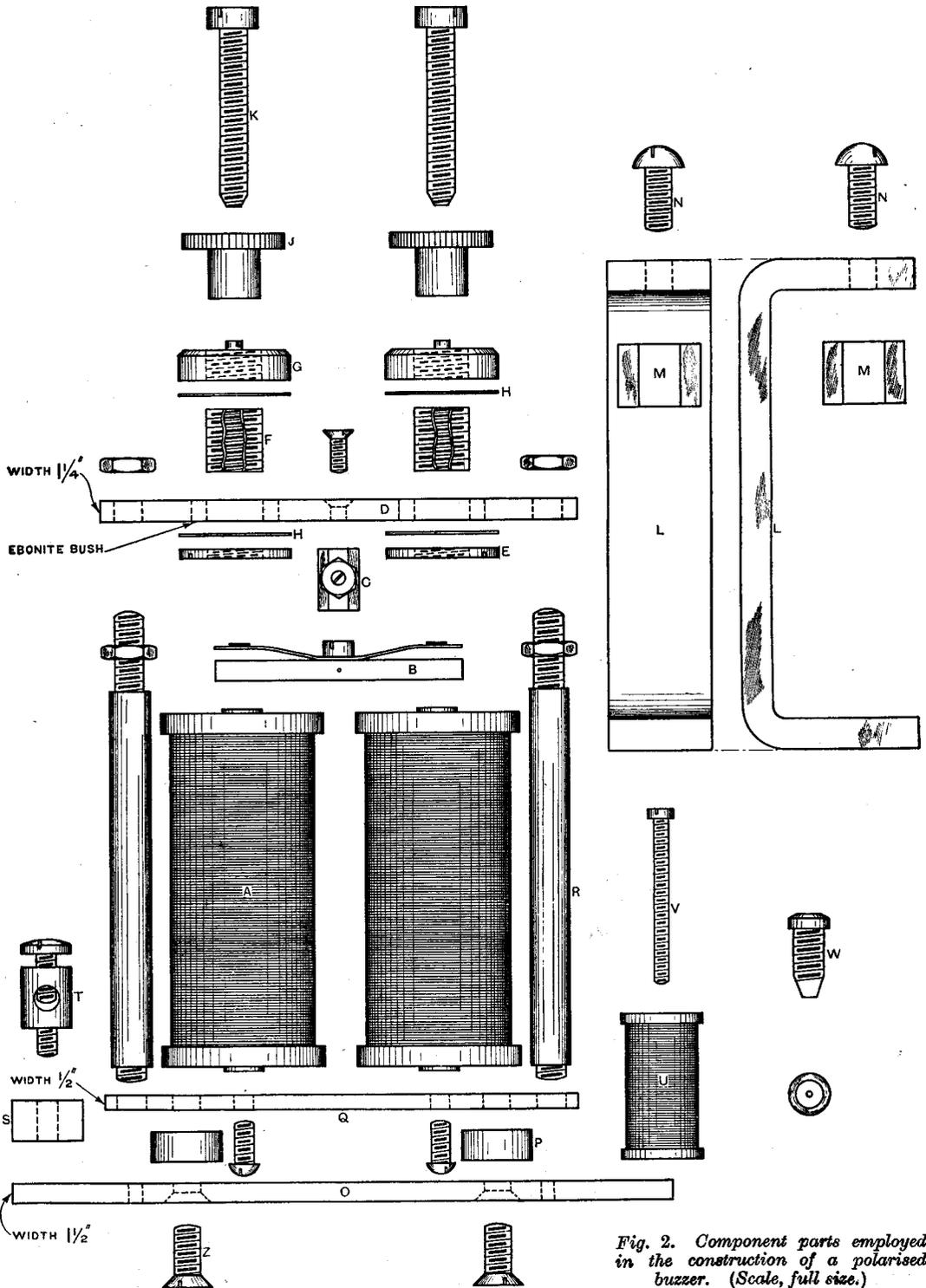
Fig. 2. Component parts employed in the construction of a polarised buzzer. (Scale, full size.)
