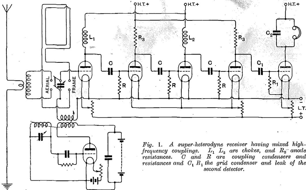
Fig. 1. A super-heterodyne receiver having mixed high-frequency couplings.  $L_1$   $L_2$  are chokes, and  $R_3$  anode resistances.  $C$  and  $R$  are coupling condensers and resistances and  $C_1$   $R_1$  the grid condenser and leak of the second detector.
