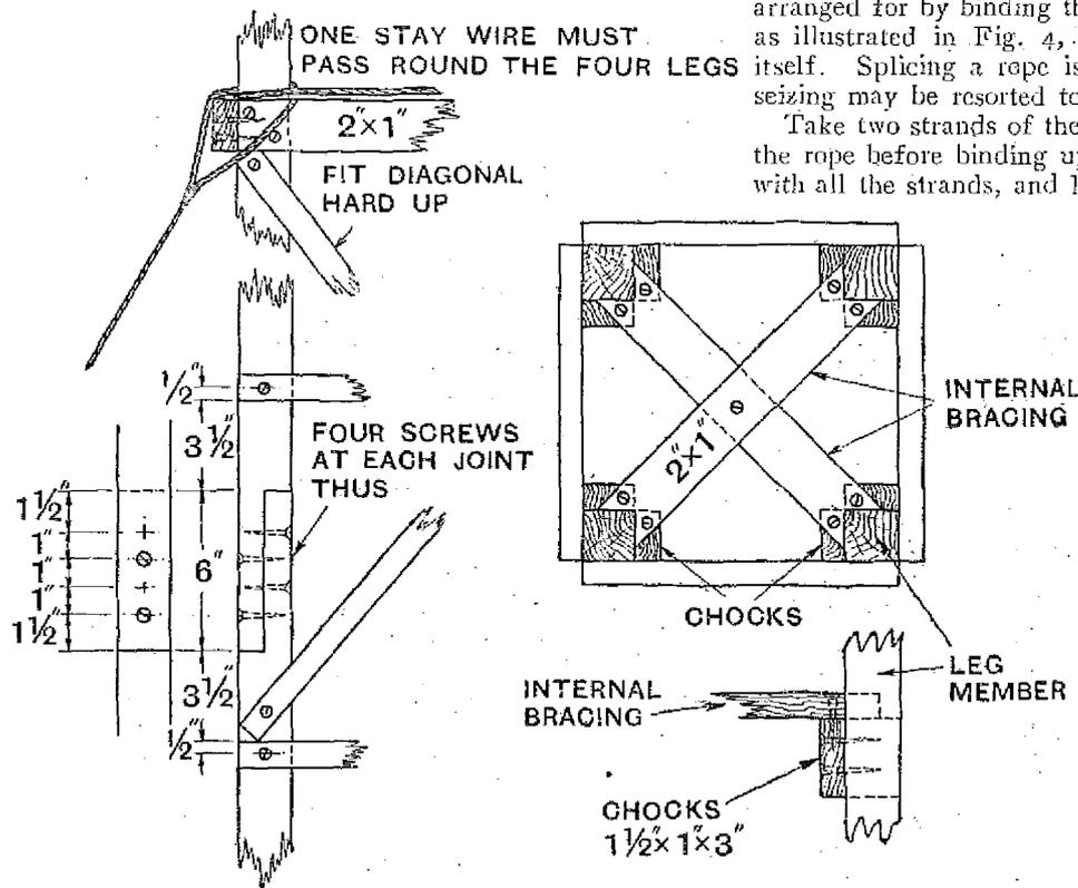
Fig. 4.—Details of the stay attachment.
