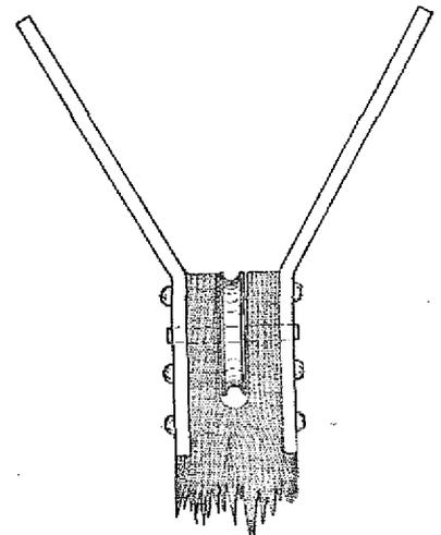
By terminating a mast in this manner, it is always a simple matter to restore a broken aerial halyard.
