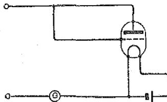
Fig. 1.—A valve rectifier and galvanometer.
