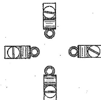
View showing the arrangement of the contacts on the underside of the panel.
