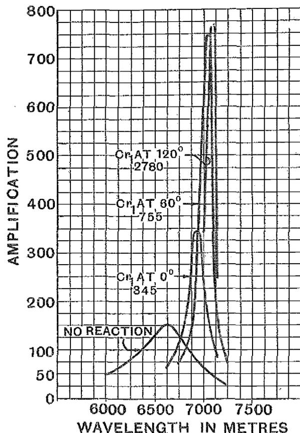
Fig. 7.—Effect of capacity reaction on two-stage H.F. amplifier. Note:  $C_2$  adjusted so that  $C_1$  at 180° just sets the valve in oscillation.
