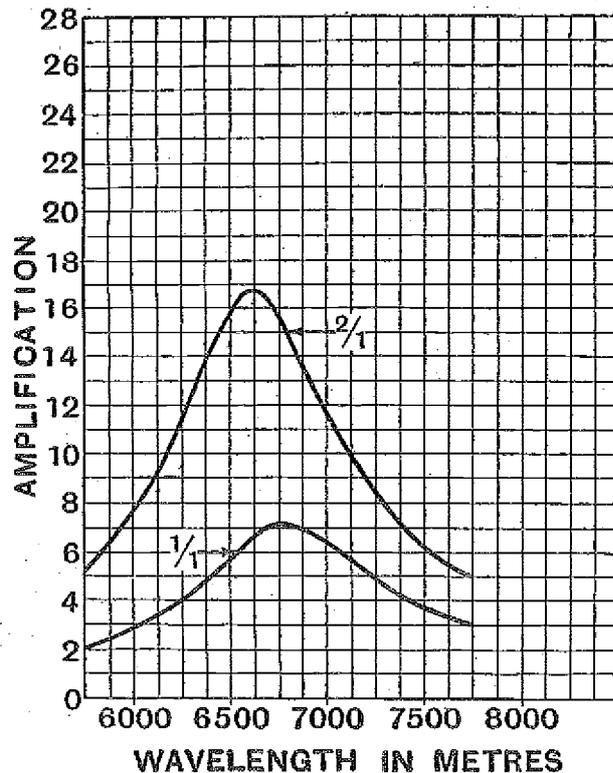
Fig. 4.—Comparison of transformers having ratios of 2/1 and 1/1.
