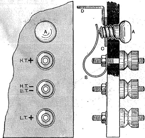
*A flash lamp connected in the high tension battery lead will prevent the valve filaments from being destroyed by accidental contact with the plate socket.*
