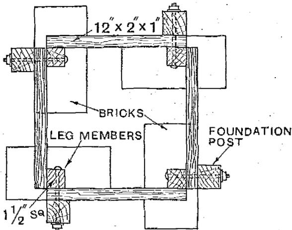
Fig. 3c.—Plan of the base.
