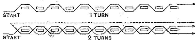
Fig. 4.—Winding of a simple basket coil having a pitch of 2.
