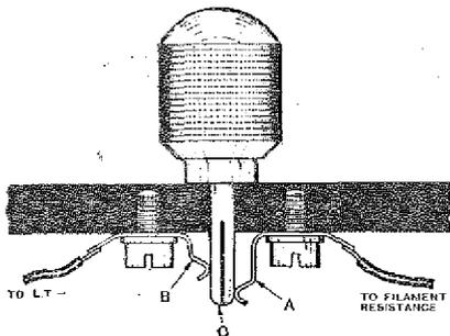
Using a plug to break the filament circuit. To be effective as a "lock" the contacts must be beneath the panel.
