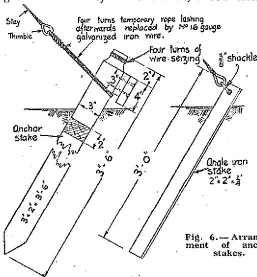
Fig. 6.—Arrangement of anchor stakes.
