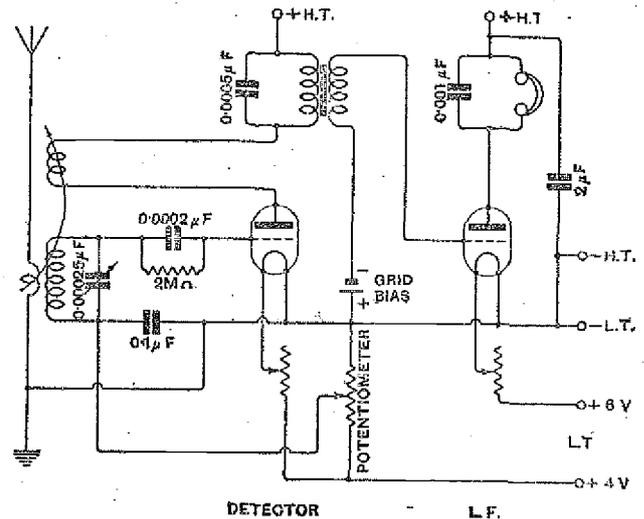
Fig. 1.—Schematic connections of the set.
