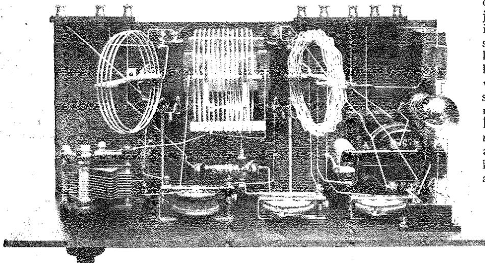
View of the set from above. On the panel may be seen the tuning condenser, potentiometer, two filament resistances and the telephone condenser. The centre coil is the removable closed circuit coil; on the left the aerial coil, and right, the reaction coil.
