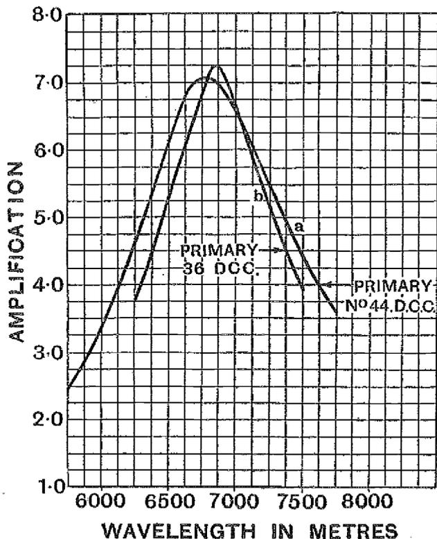
Fig. 3.—Effect of size of wire on amplification and selectivity.
