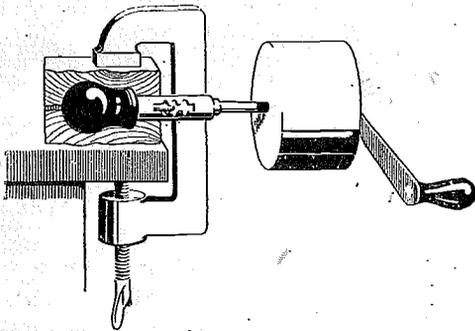
*A coil winder making use of a ratchet action screwdriver.*
