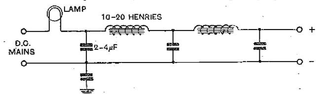
Fig. 4.—A filter for reducing commutator ripple and noises when using the mains for H.T. or filament supply.
