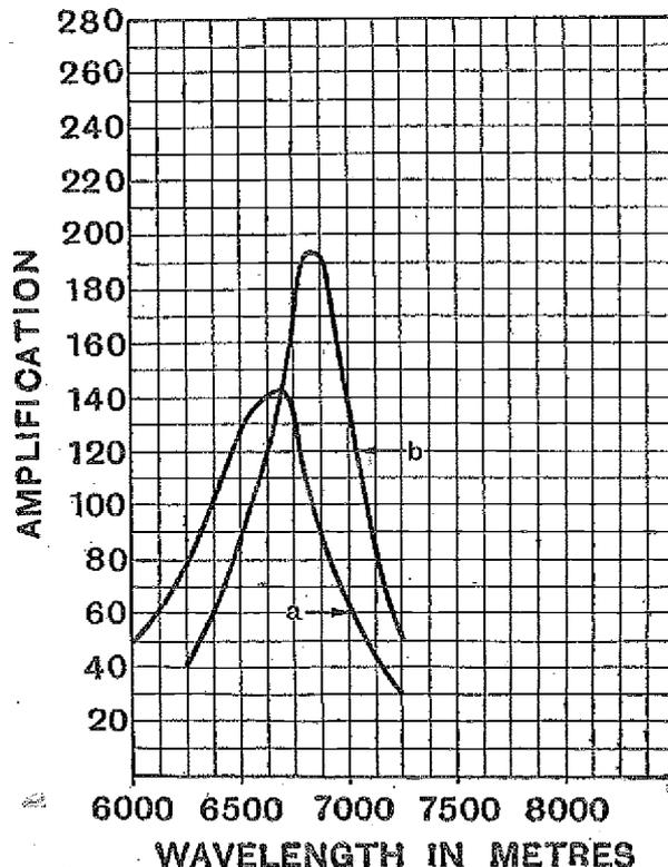
Fig. 5.—Amplification with a two-stage H.F. amplifier. The two transformers are here: (a) out of tune, and (b) carefully tuned.
