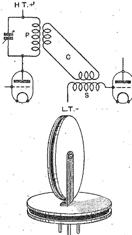
New form of construction for high frequency transformer.
