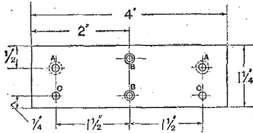
Fig. 8.—The ebonite base of the coil holder. Holes A are to take the pillars which support the movable portion, and should be drilled accordingly; holes B are for fixing screws, etc., for No. 4 B.A. screws. These screws hold connecting tags which are connected by flexible wires to the tags on the movable portion.
