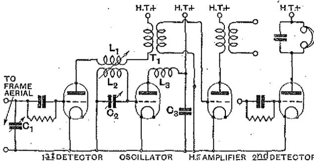
Fig. 1.—Arrangement of a super-heterodyne receiver in which the oscillator is coupled to the first H.F. transformer.
