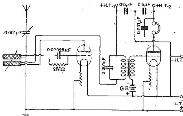
Fig. 1.—The theoretical connections of the set
