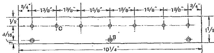
Fig. 11.—Details of the terminal strip.
