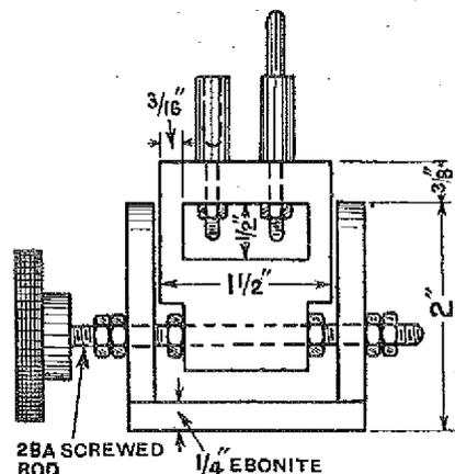
An easily constructed two-coil holder.
