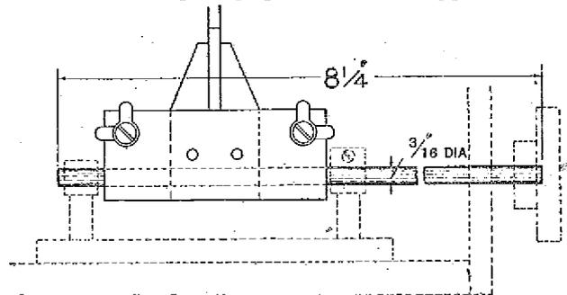
Fig. 7.—Layout of the movable coil holder for the reaction and aerial coils. Details of the base are given in Fig. 8, and of the movable pins in Fig. 9. The movable portion has a spindle passing through it which runs in two brass pillars as indicated. A knob is attached to the end of the spindle which passes through the panel.
