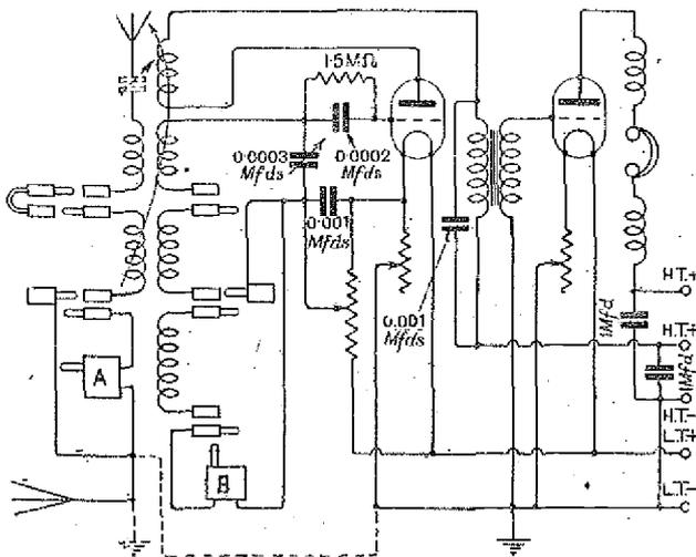
Fig. 1.—The circuit is a detector valve with reaction followed by a note magnifier. The short wave tuning inductances are shown while loading coils may be added at A and B or inserted into the plug and socket connectors in place of the "U" links.
