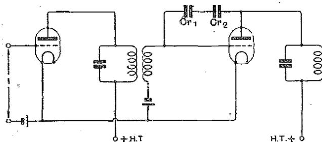
Fig. 6—Connections of the reaction condensers.
