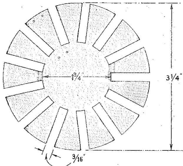
Fig. 7.—Drawing of the cardboard former of the basket coils which are used as H.F. chokes.
