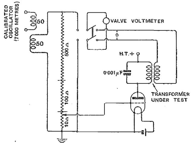
Fig. 2a.—The apparatus employed when testing the H.F. amplifier.
