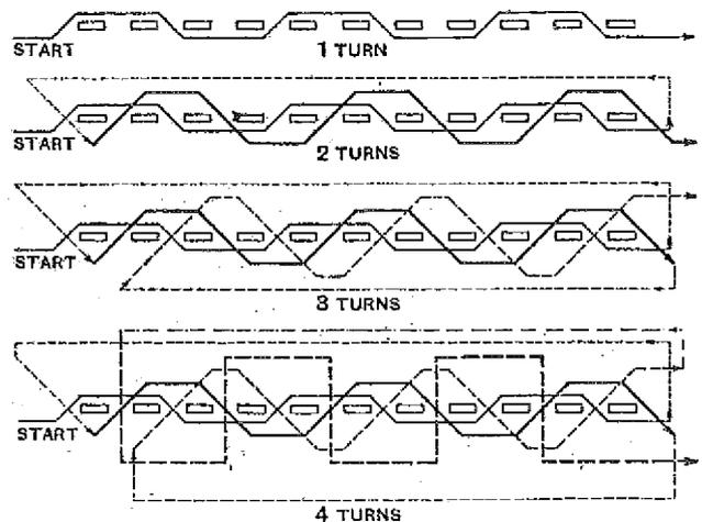
Fig. 2.—Method of winding the basket coil.
