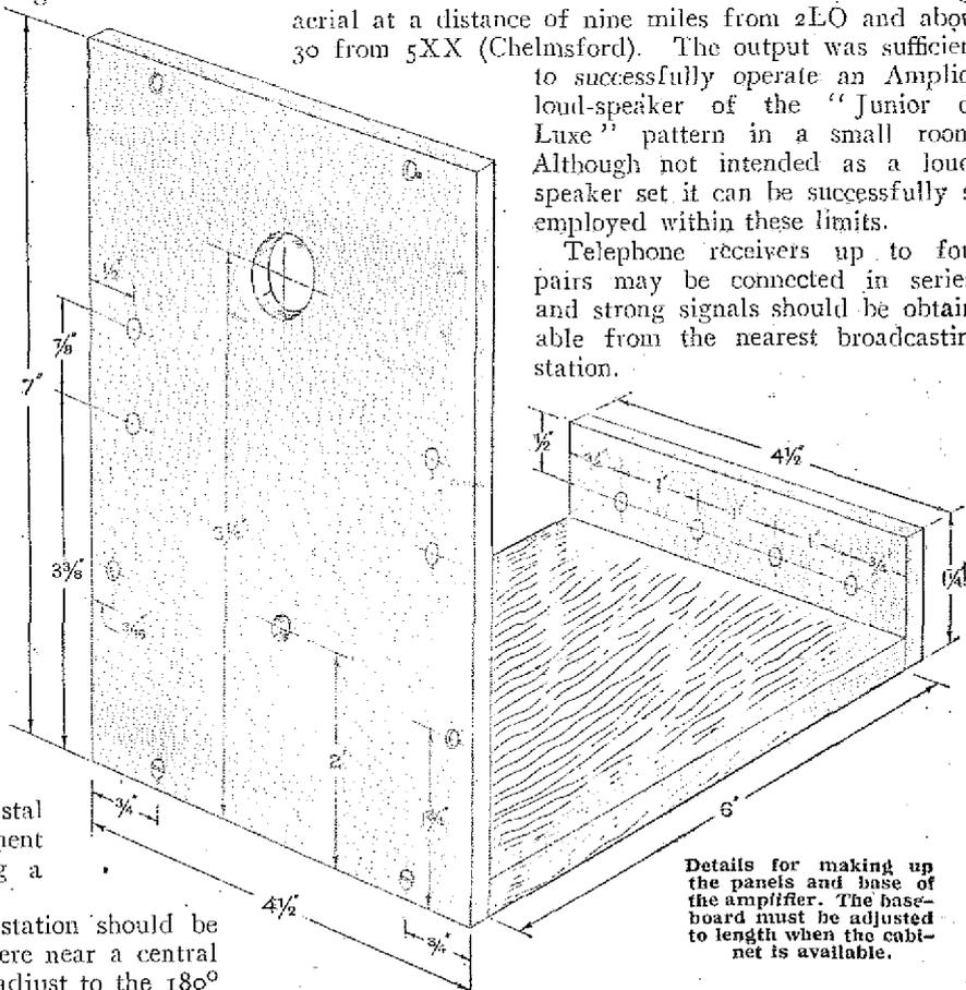
Details for making up the panels and base of the amplifier. The base-board must be adjusted to length when the cabinet is available.
