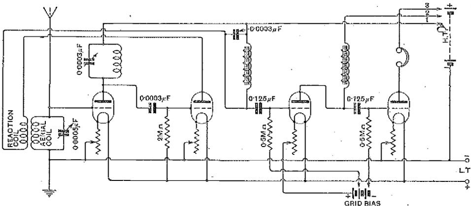
Connections of a four-valve receiver with one H.F. valve detector and two L.F. stages. The H.F. stage is tuned anode coupled, and the L.F. stages are choke coupled.
