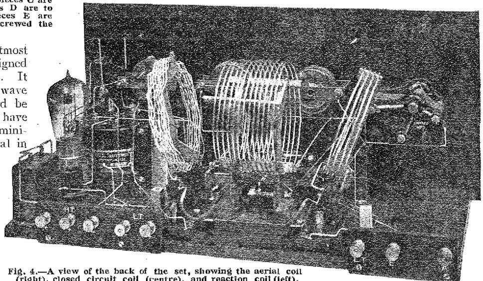
Fig. 4.—A view of the back of the set, showing the aerial coil (right), closed circuit coil (centre), and reaction coil (left).
