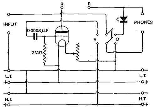
Fig. 1. The theoretical connections of the panel.
