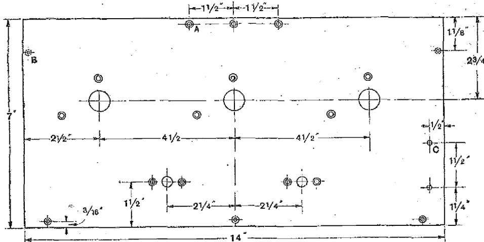
Fig. 3.—Drilling details of ebonite front panel. A = drill  $\frac{3}{16}$  in. and countersink. B = drill  $\frac{1}{4}$  in. and countersink. C = drill  $\frac{1}{2}$  in.
