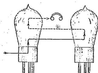
Fig. 1.—The reflex principle.
