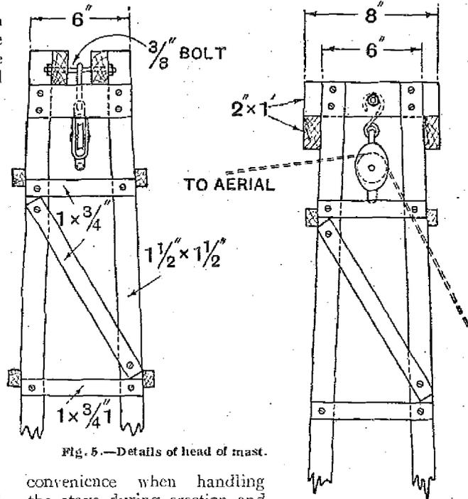
Fig. 5.—Details of head of mast.
