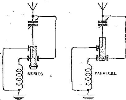
A plunger type series-parallel switch and the manner of connecting it in the tuning circuit.
