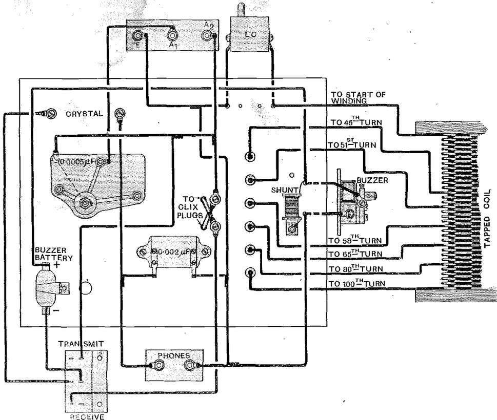
Fig. 6. The wiring diagram. The connection strips, loading coil socket, buzzer and tapped coil, are shown removed from the panel for clearness.
