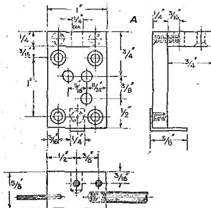
Details for making the plunger type series-parallel switch.
