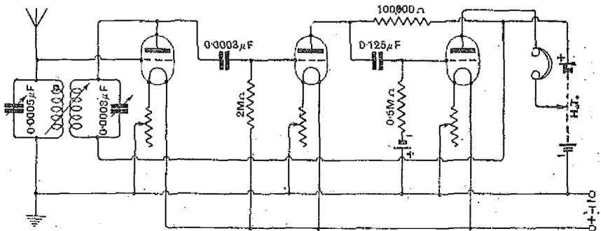
A three-valve receiver with one H.F. detector and one stage of resistance coupled L.F. Reaction is obtained by coupling the anode and aerial coils.
