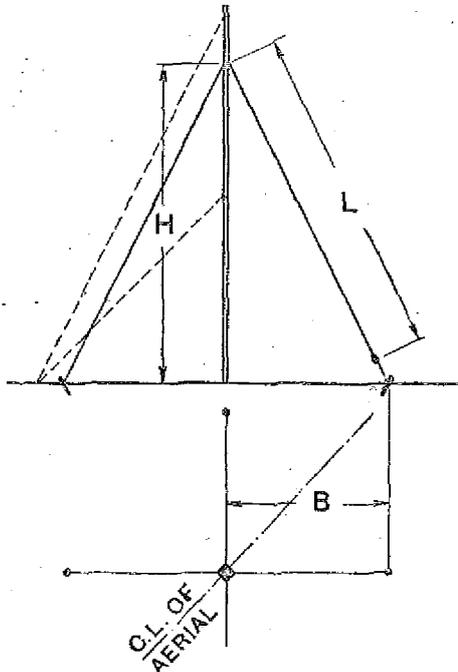
Fig. 1.—Layout of aerial. H=Height of stays; L=Length of stays; B=Length of base.
