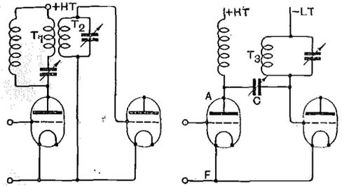
*Figs. 3 and 4. In Fig. 3 a tuned transformer is employed, and in Fig. 4 a tuned auto-transformer.*
