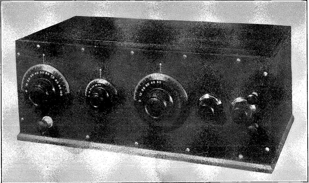
*A view of the set. On the left is the variable condenser tuning the closed circuit coil. The next knob, which is smaller, controls the coupling of the aerial and secondary coils, while the third knob is for adjusting the reaction coupling. There are two filament resistances, and the telephones are connected to the terminals on the right of the set.*
