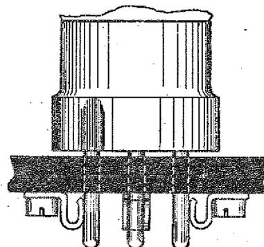
Design for a valve holder with contacts beneath the panel, and presenting very little stray capacity.
