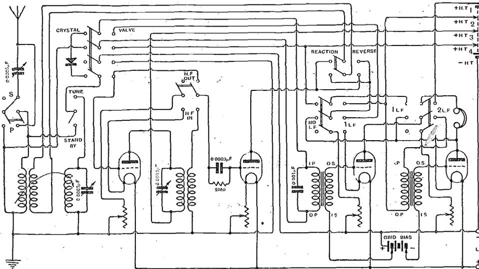
A four valve receiver with switches to enable valves to be put in or out of circuit, or a crystal to be employed as a detector instead of a valve.
