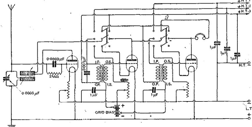
A three-valve receiver, in which the switches in the L.F. stages maintain the correct plate potentials.
