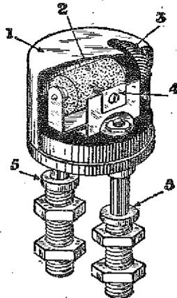
The internal construction of the Harlie detector
