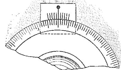
Fig. 5.—A vernier setting may be obtained by sticking a piece of paper, marked as shown here, above the scale of the dial.
