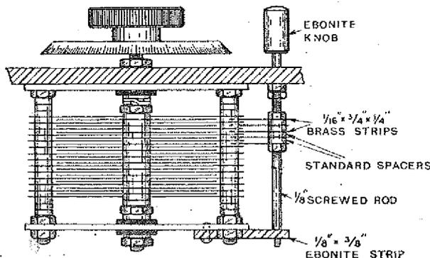
Fitting a vernier control to a variable condenser by means of a spindle carrying a few semi-circular plates, and engaging into the projections of the fixed plates.
