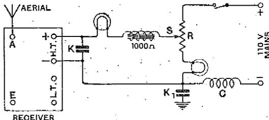
In order to avoid any eventual trouble of this kind, I have carried out further experiments, and find that an equally good H.T. supply can be obtained from the mains by the method shown in Fig. 1.
