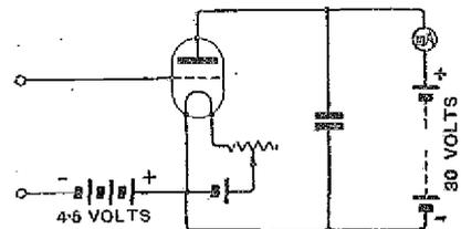
Fig. 2b.—Connections of the valve voltmeter employed in the circuit of fig. 2a.
