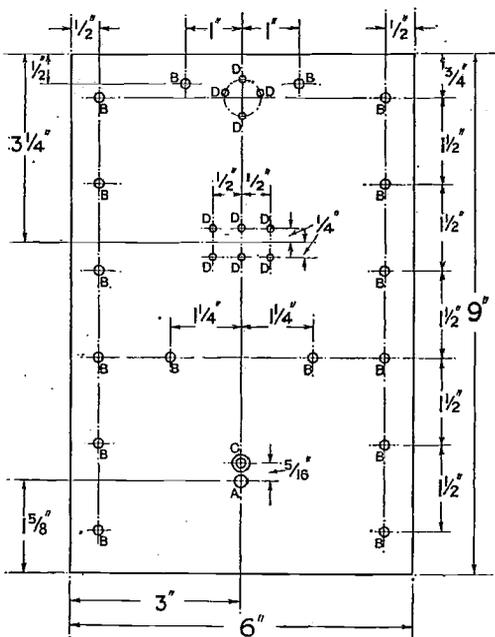
Fig. 2. Details of the panel. A, drill  $\frac{3}{16}$ " dia.; B, drill  $\frac{5}{32}$ " dia.; C, drill  $\frac{5}{32}$ " and countersink for No. 4 B.A. screws; D, drill  $\frac{1}{8}$ " dia.
