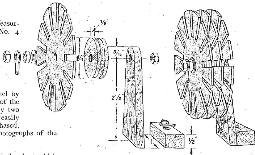
Fig. 8.—Arrangement of the H.F. chokes when they consist of three basket coils connected in series.
