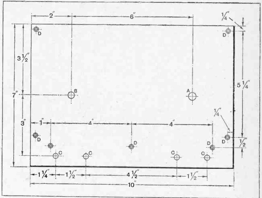
Fig. 2.—Drilling details of top panel. A, 3.8in. dia.; B, 5/16in. dia.; C, 1/4in. dia.; D, 1/8in. dia., countersunk for No. 4 wood screws.
