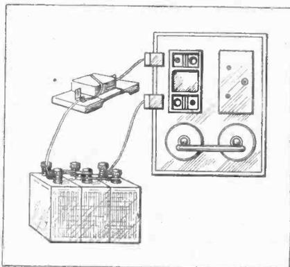
Fig. 1.—Charging batteries from the mains.
