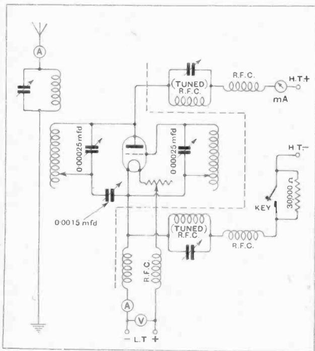
Fig. 1.—Complete circuit diagram of transmitter arranged for third harmonic excitation. The portion to the right of the dotted line is built as a separate unit.
