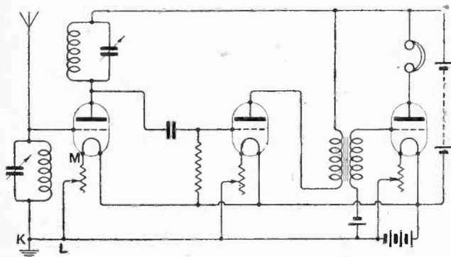
Fig. 3.—Typical three-valve receiving circuit.
