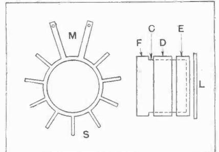
**Former for winding double-weave coils
