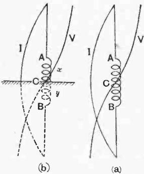
Fig. 1.—Distribution of current and potential (a) in half-wave oscillator and (b) in quarter-wave oscillator.
