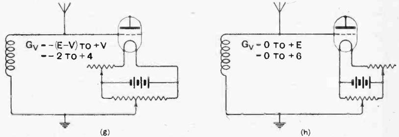
Fig. 2.—Range of voltages available with the addition of a potentiometer.
