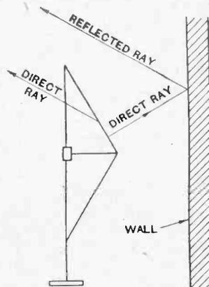
Fig. 2.—Direct and reflected waves from cone loud-speaker.
