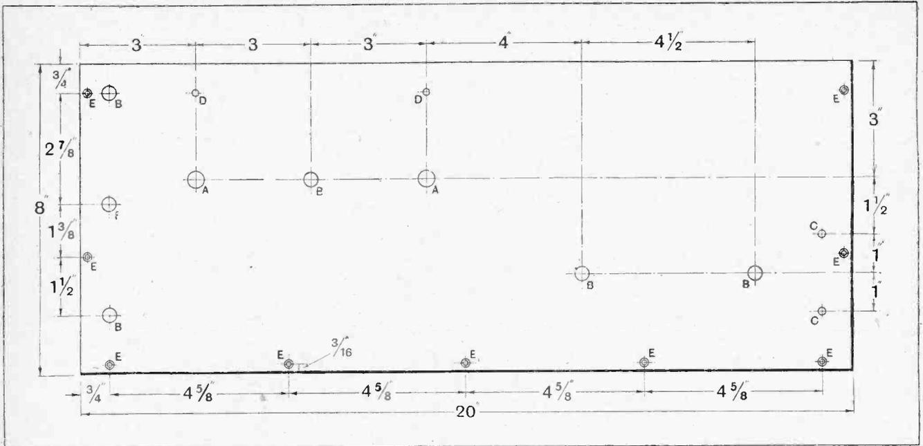
Fig. 2.—Dimensional details of the front panel. Drilling sizes are as follow: A, 7/16in. dia.; B, 3/8in. dia.; C, 3/16in. dia.; D, 5/32in. dia.; E, 1/8in. dia.; and countersunk for No. 4 wood screws.
