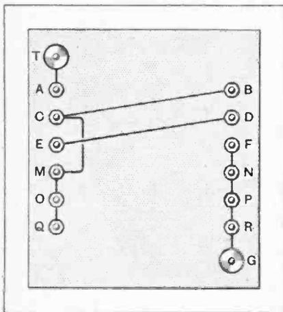
Wiring diagram of panel for obtaining various grid leak values from different combinations of a series of three fixed resistances.
