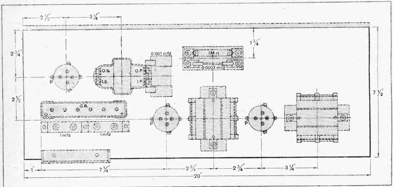
Fig. 3.—Details of the baseboard layout.
