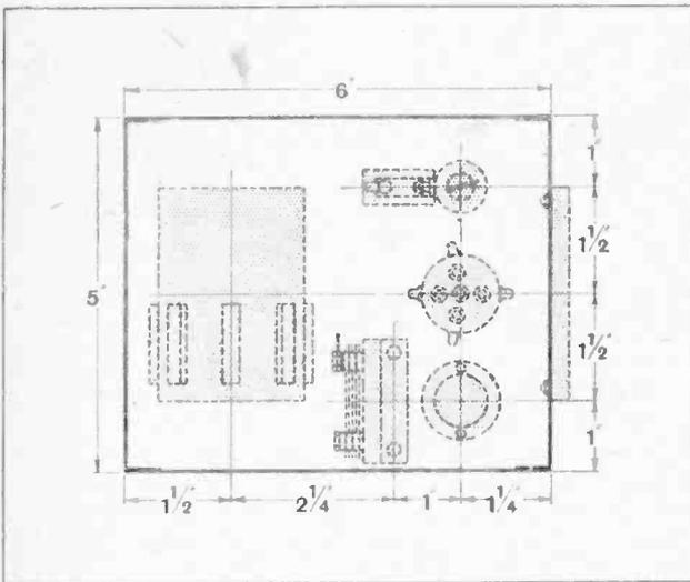
Fig. 3.—Layout of apparatus on baseboard of radio receiver.
