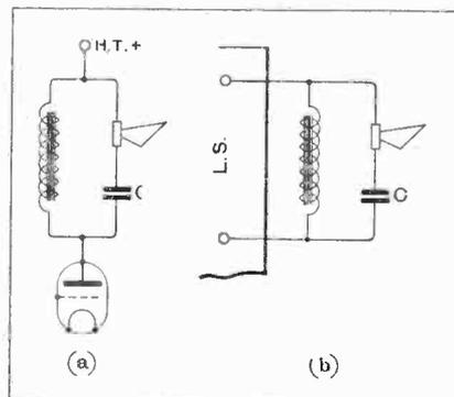
Fig. 1. — (a) A choke-capacity output circuit. At (b) its connections to the loud speaker terminals of an existing set are shown.
