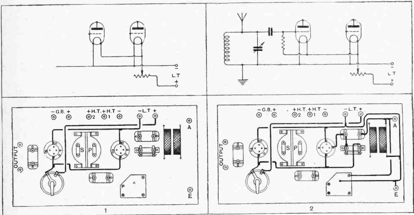
The filament circuits are wired in the usual manner. In this particular case a single rheostat is used to control both valves.
