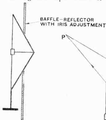
Fig. 3.— Loud-speaker with adjustable baffle-reflector.
