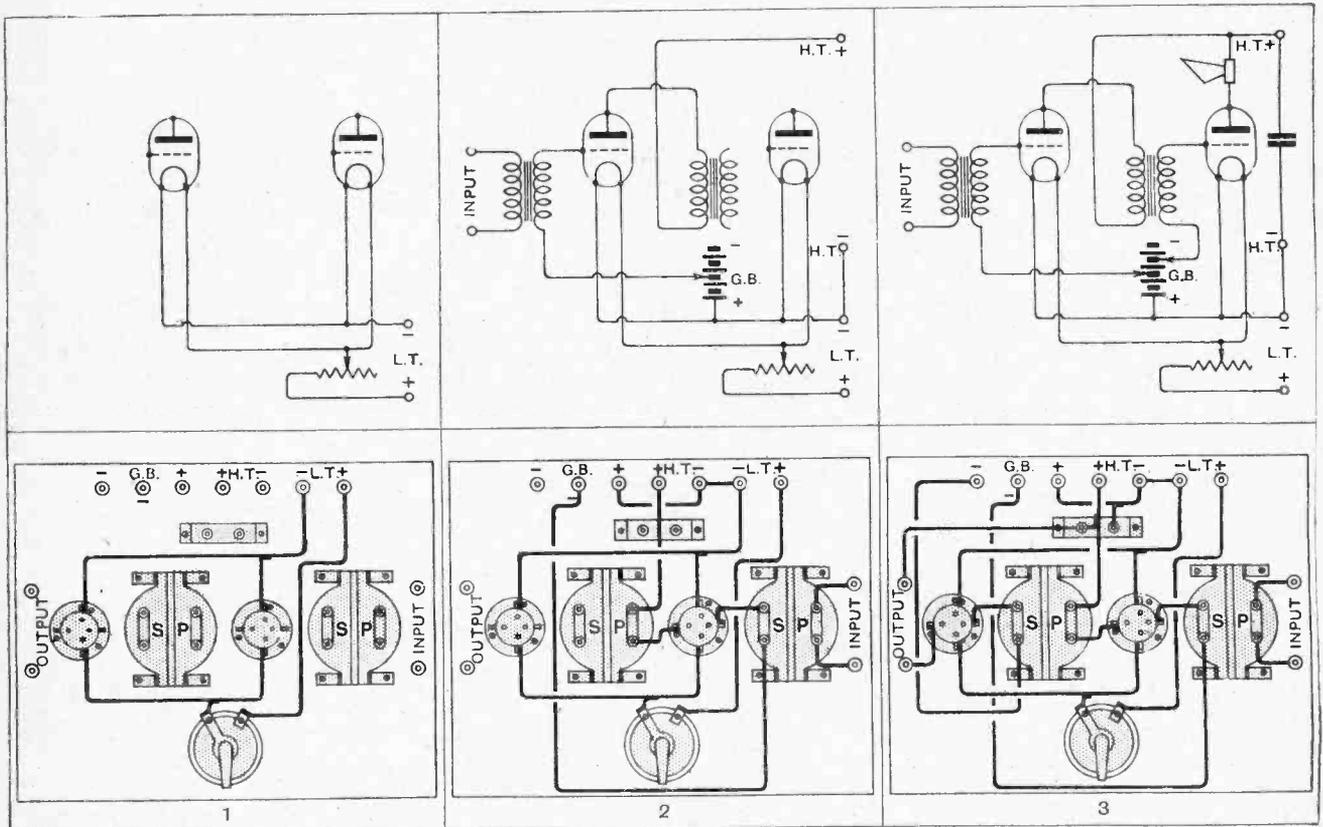
The filament circuits are wired in the conventional manner. A single rheostat, which controls both valves, is inserted in the L.T. positive lead as usual. Separate rheostats must be used if the two valves have different filament characteristics.
