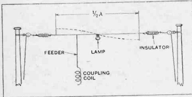
Fig. 2.—Half-wave Hertz aerial with single feeder. The dotted line indicates the voltage distribution.
