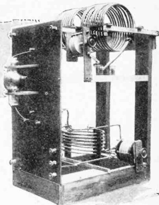
The circuit chosen, after many trials, is the tuned grid and plate arrangement, commonly known as the Armstrong circuit (Fig. 1).
