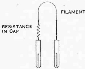
Fig. 4.—Special case of permanent resistance in series with the valve filament.
