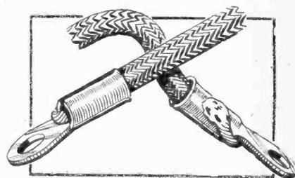
Fig. 2.—Finishing off connecting leads.
