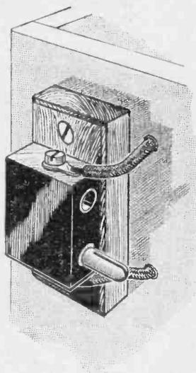
Fig. 5.—Mounting of the coil holder.
