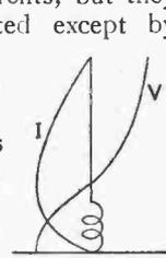
Fig. 2.—Current and potential distribution with "insulated earth."
