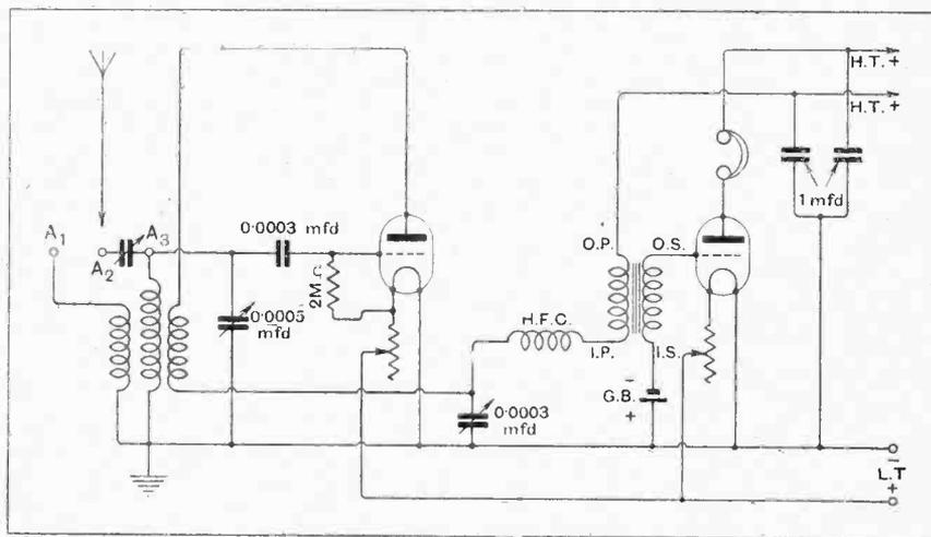
Fig. 1.—A sensitive arrangement of two valves.
