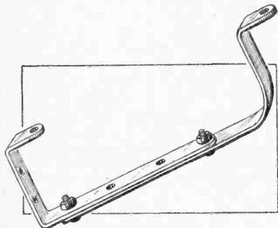
Adjustable bracket for securing the panel and baseboard and arranged to support an elevated platform.
