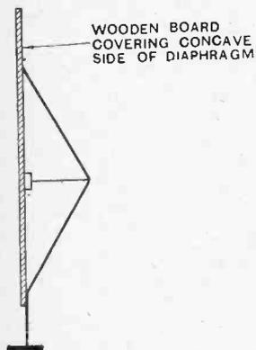
Fig. 6.—Experiment to show suppression of low tones by closing one side of diaphragm
