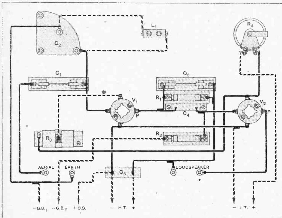
Fig. 4.—The practical wiring plan. Flexible connectors are shown in broken lines. The lettering of the components corresponds with that of the other diagrams.
