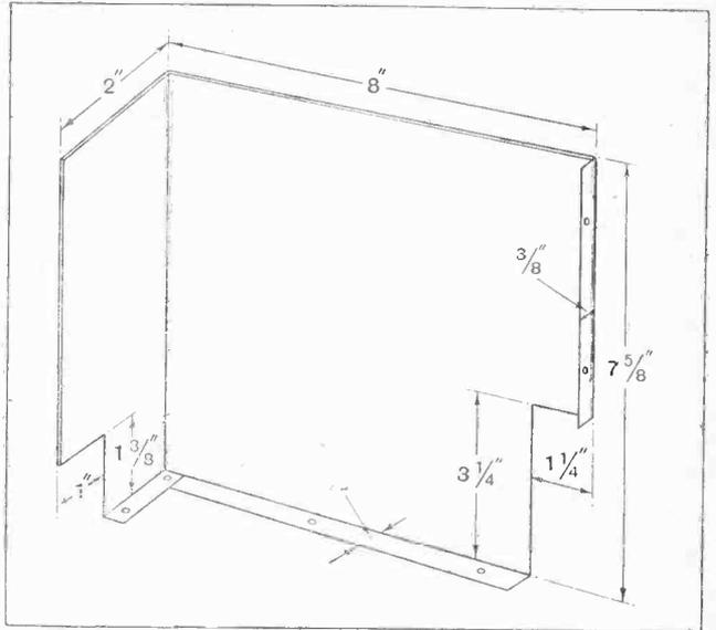
Fig. 4.—The copper or aluminium screen.
