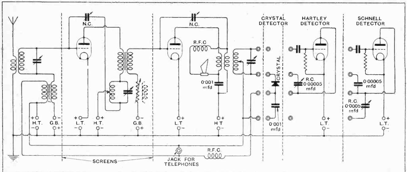
Fig. 6.—Schematic diagram showing how the crystal in Fig. 5 may be replaced by well-known reacting valve detectors.
