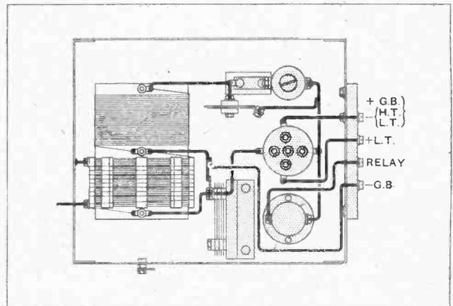
Fig. 6.—Wiring diagram for the radio receiver.
