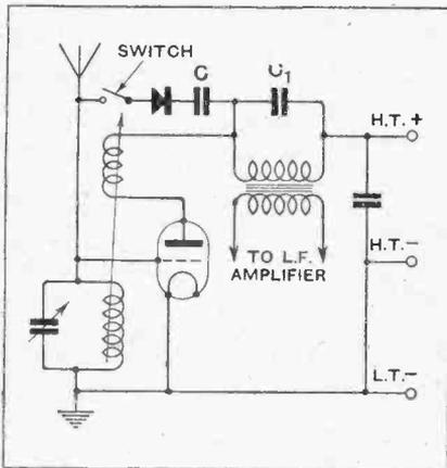
Fig. 1.—Changing from valve to crystal detection.
