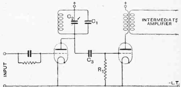
Fig. 1.—Connections of tuned-anode circuit with auxiliary condenser for changing the intermediate frequency.
