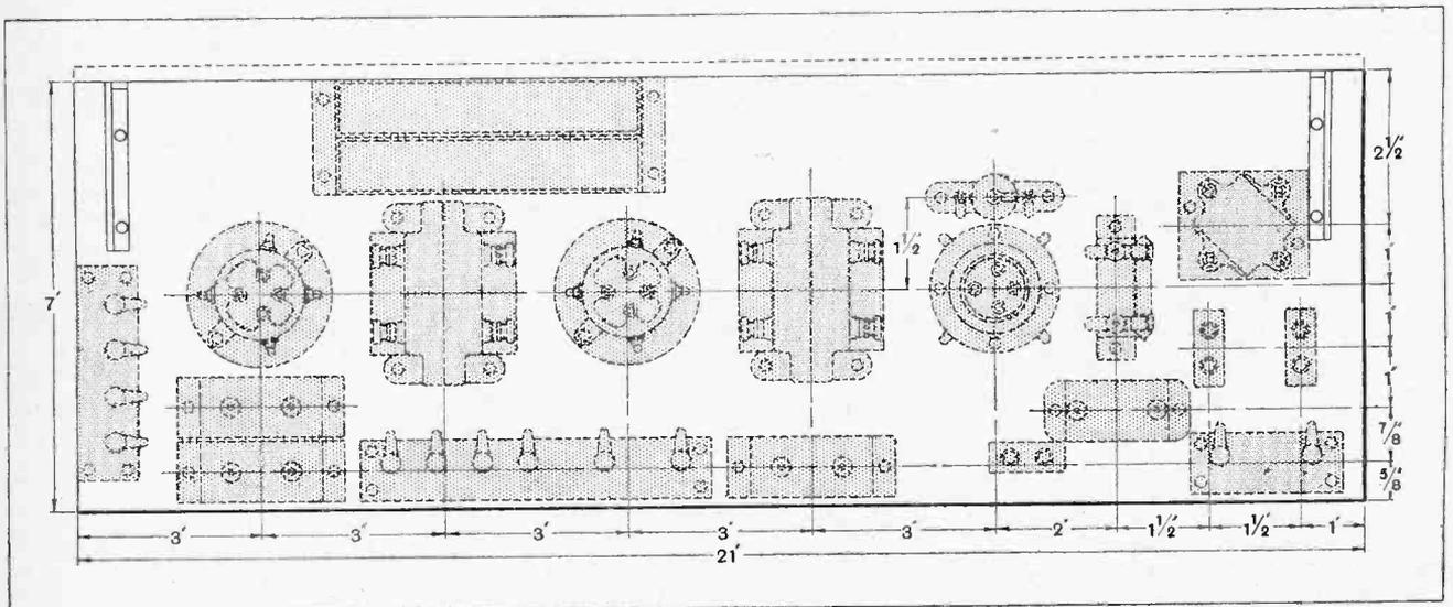
Fig. 3.—Layout of components on baseboard.
