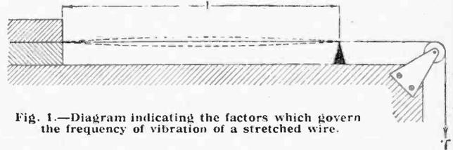
Fig. 1.—Diagram indicating the factors which govern the frequency of vibration of a stretched wire.
