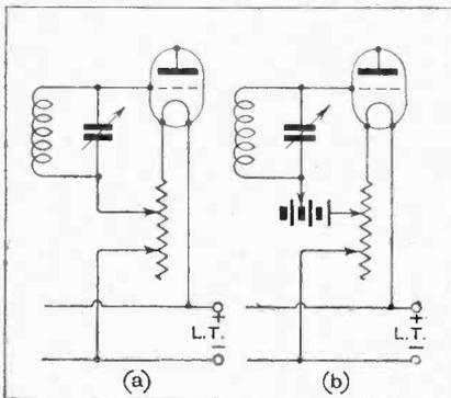
Fig. 1.—Connecting a filament rheostat to control grid bias.
