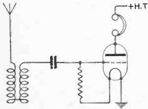
Fig. 5.—Connections of half-wave oscillator with potential rectification.
