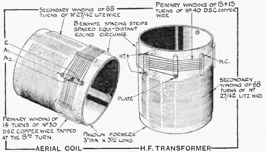
Fig. 2.—Details of the aerial-grid and intervalve high-frequency transformer windings.
