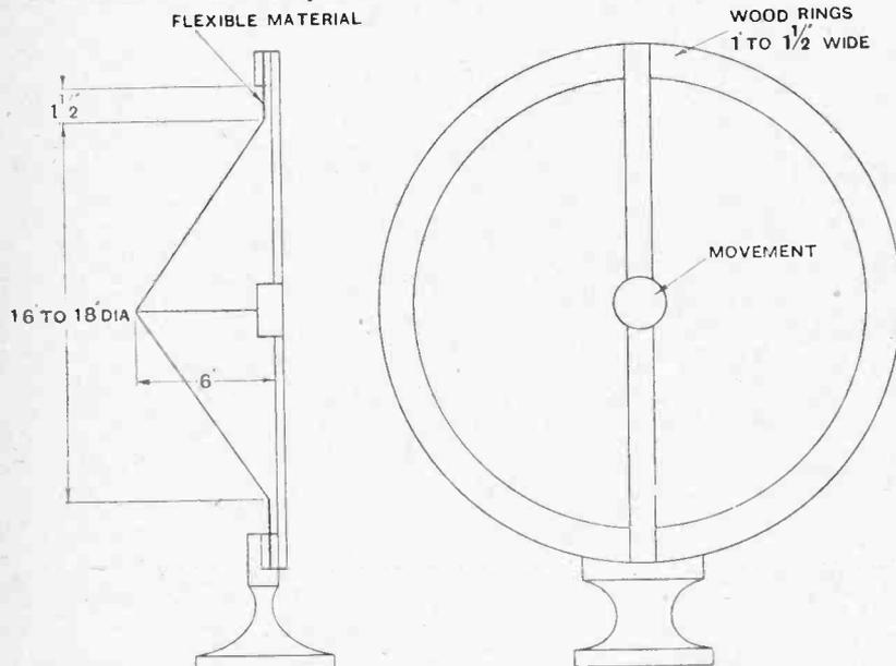
Fig. 1.—Details of experimental loud-speaker.
