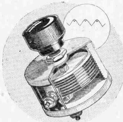
Totally enclosed rheostat in which the resistance wire is carried in a spiral groove so that maximum to minimum adjustment is spread out over seven complete turns of the knob.
