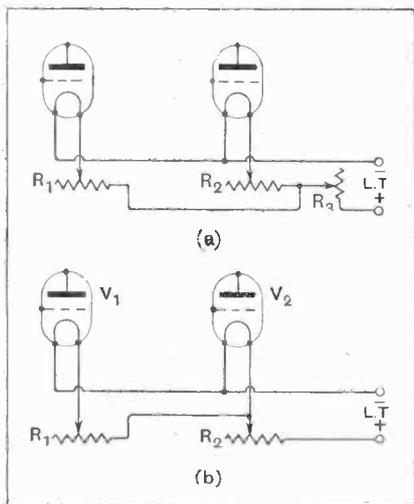
Fig. 1.—Methods of filament control.
