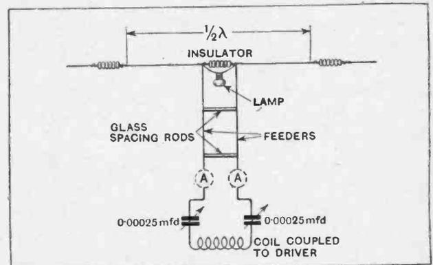
Fig. 3.—Hertz aerial with twin feeders. The lamp is removed and ammeters inserted in each feeder after wavelength adjustment.
