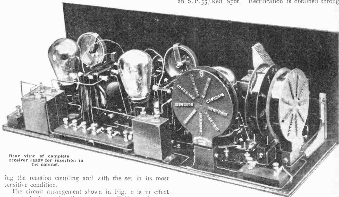
Rear view of complete receiver ready for insertion in the cabinet.
