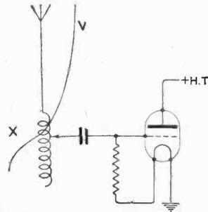
Fig. 6.—Method of exploring distribution of potential on half-wave oscillator.
