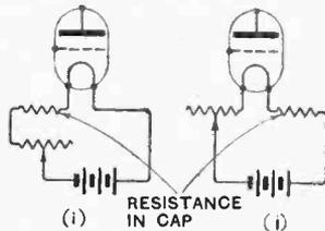
Fig. 5.—Alternative positions for external variable resistance relative to the fixed internal resistance.
