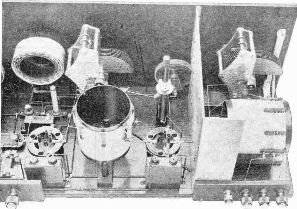
The high-frequency and detector circuits: on the right is the aerial coil, tuning condenser, connection strip and screen. Behind the right-hand valve-holder is the balancing condenser and volume control rheostat, while to the left can be seen the Daventry plug-in type coil.
