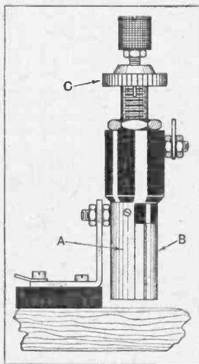
Fig. 4.—Showing details of reaction condenser mounting. A = fixed plate, B = moving plate, C = clamp.
