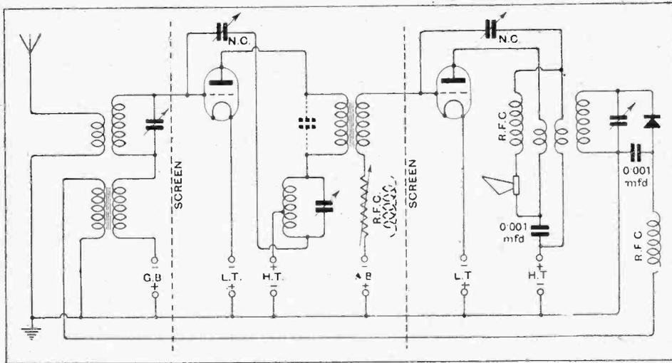
Fig. 5.—Schematic circuit diagram of a practical two-valve and crystal reflex receiver.
