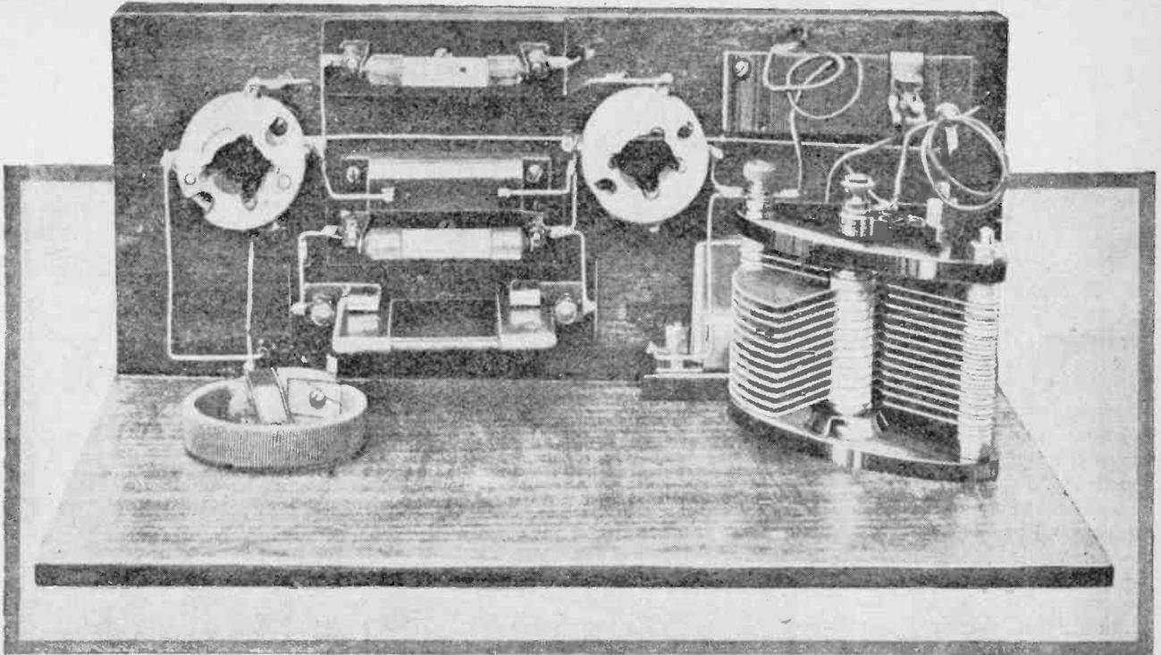
Another view showing the mounting of components. Note the flexible leads from the variable condenser terminals for joining to the external coil holder.
