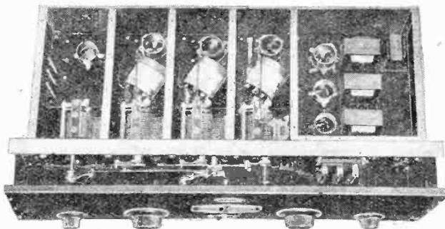
Seven valve "Howard" neutrodyne receiver with top shield removed. The condensers tuning the three H.F. stages are interconnected by a link motion between the front panel and screening box. The three L.F. stages are coupled by one 2 to 1 and two 1 to 1 ratio transformers.
