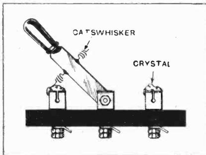
S.P.D.T. knife switch converted to a crystal detector.
