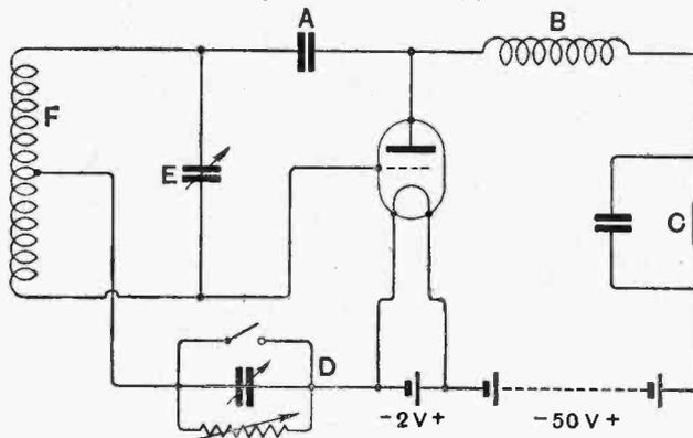
Fig. 1.—Circuit diagram of the wavemeter.
