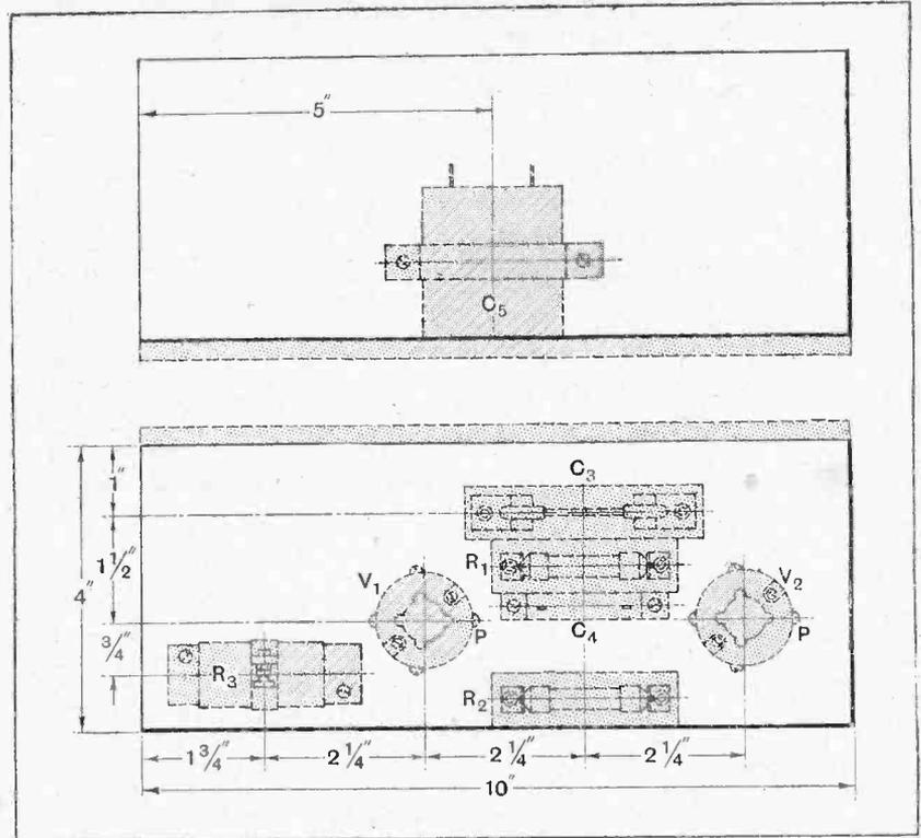
Fig. 3.—Mounting of condenser on back of sub-panel and (below) layout of components on the front of this panel.
