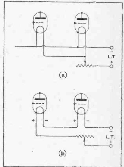
Fig. 2.—Valve filaments in parallel (a) and in series (b). In the latter arrangement the positive and negative ends of each filament are marked.
