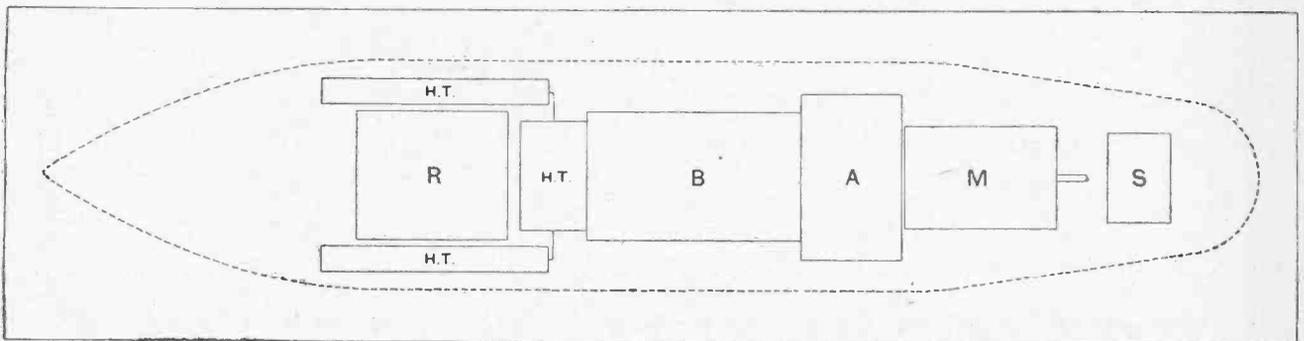
Fig. 1.—Outline sketch of boat. R=radio receiver; B=electric "brain"; A=accumulator; M=motor; S=steering gear.
