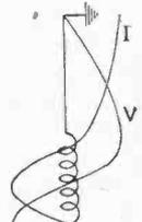
Fig. 7.—Three-quarter wave oscillator with remote end of aerial earthed.
