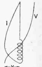
Fig. 4.—Distribution of current and potential for "end-loaded" half-wave oscillator.
