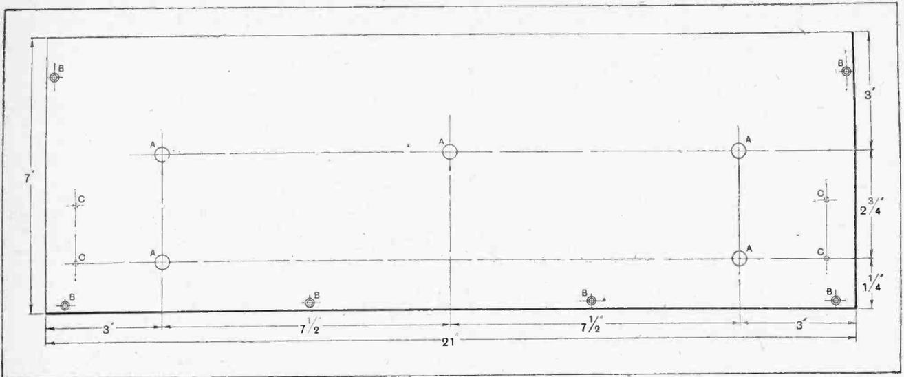
Fig. 2.—Drilling details of front panel. A, 3/8in. dia.; B, 1/8in. dia., countersunk for No. 4 wood screws; C, 7/64in. dia. for back, tapped No. 4 B.A.
