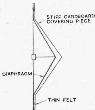
Fig. 7.—Alternative method of suppressing low tones in a diaphragm loud-speaker.
