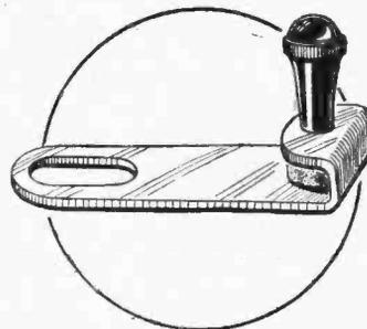
An inexpensive vernier control which is easily attached by clamping the bracket down under a one hole fixing nut.
