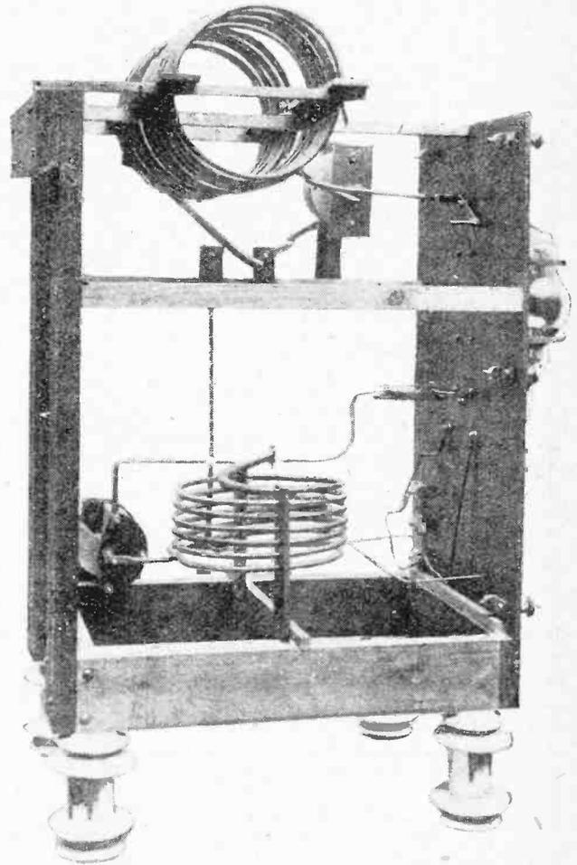
Side view of oscillator frame, showing aerial, grid and anode coils.
