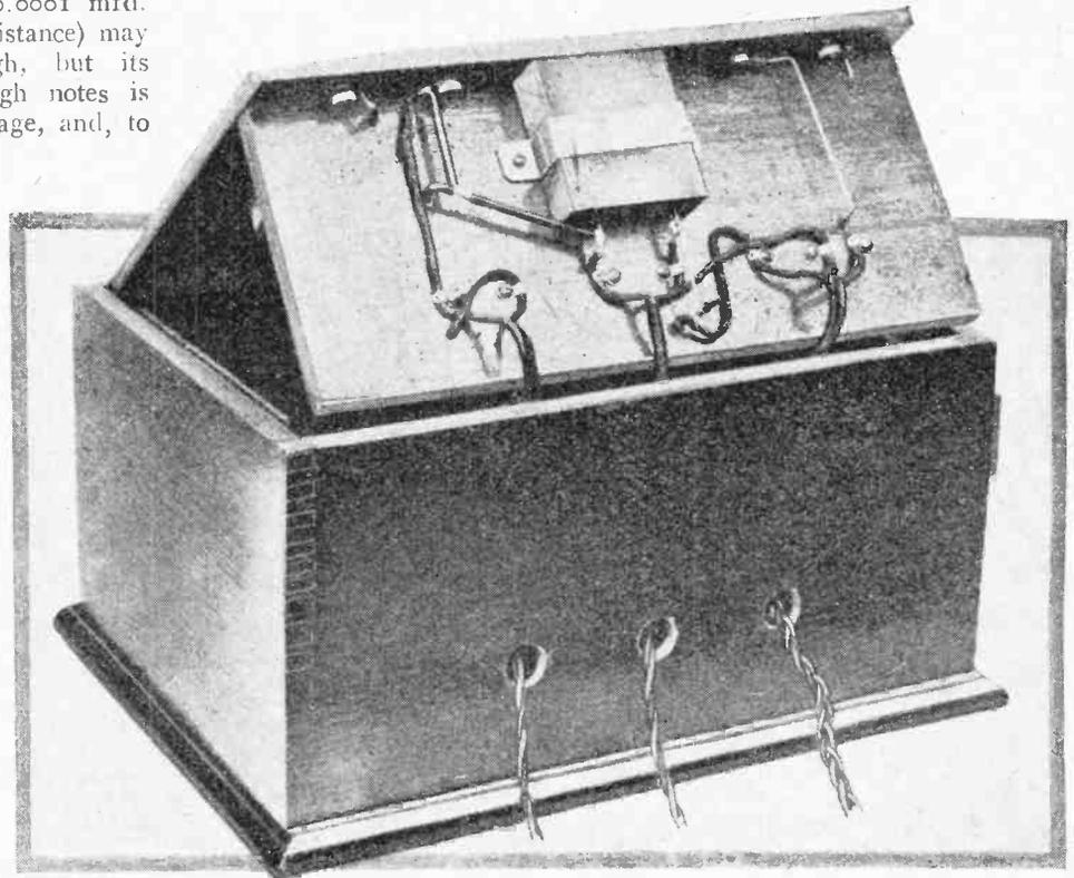
The set partly removed from the cabinet. The method of securing the flexible leads is clearly shown.
