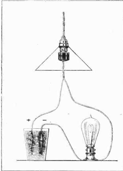
Fig. 2.—Testing mains for polarity.
