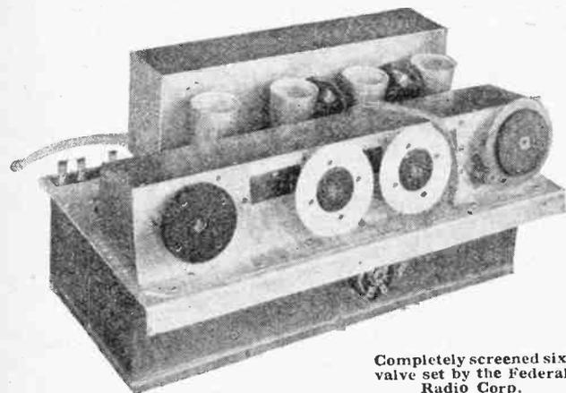
Completely screened six-valve set by the Federal Radio Corp.
