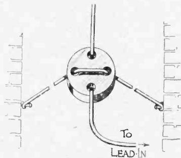
Method of bracing aerial down-lead.
