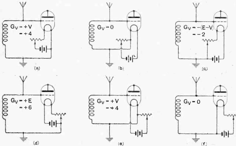
Fig. 1.—Six methods of connecting filament battery, filament resistance and grid return lead to obtain various values of grid bias. V=normal filament voltage=4; E=voltage of L.T. battery=6.
