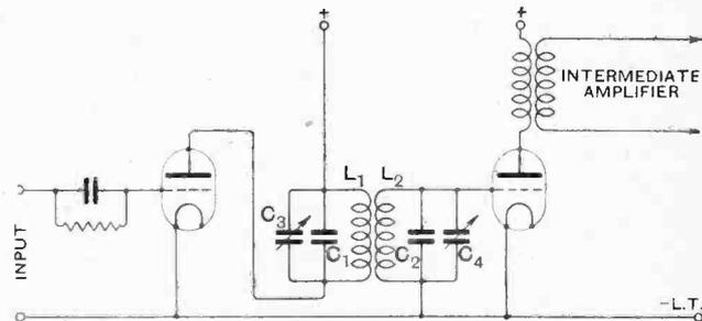
Fig 2.—Tuned transformer for coupling valves in the intermediate amplifier with auxiliary frequency changing condensers.
