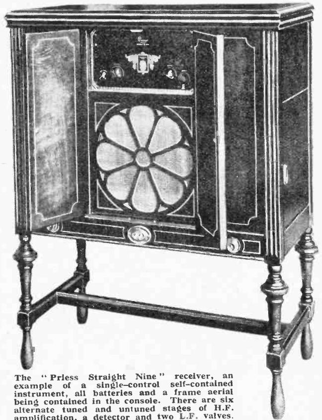
The "Priess Straight Nine" receiver, an example of a single-control self-contained instrument, all batteries and a frame aerial being contained in the console. There are six alternate tuned and untuned stages of H.F. amplification, a detector and two L.F. valves.
