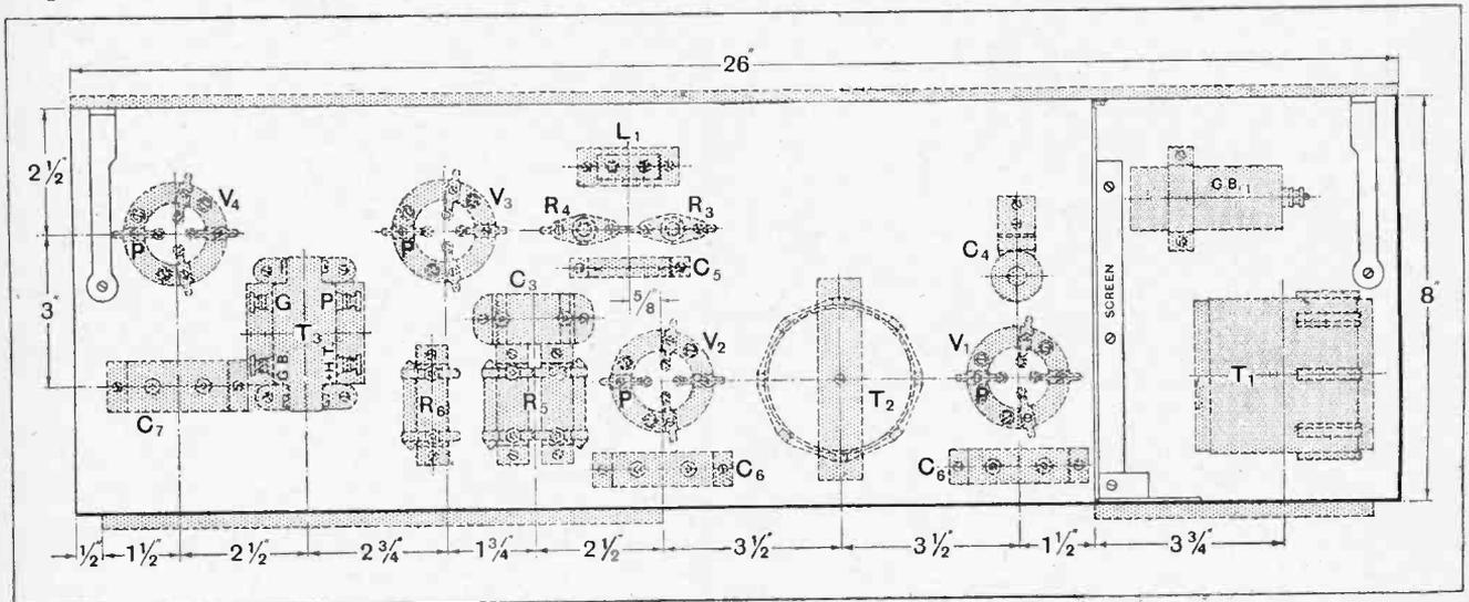
Fig. 6.—Arrangement of parts on baseboard. See Fig. 1 for values of parts.
