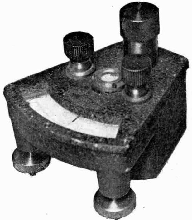
Fig. 5.—Pye suspension type moving-coil galvanometer with pointer and scale, in which readings as small as 0.25 microampere can be taken. This instrument is marketed at a very popular price.
