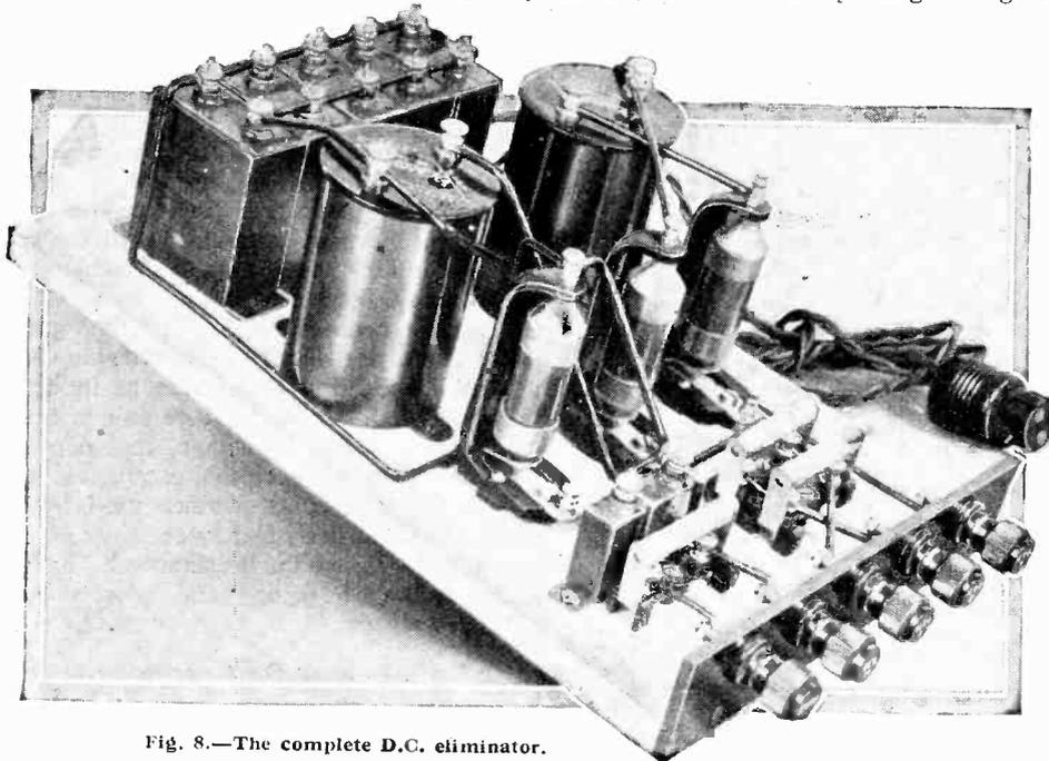
Fig. 8.—The complete D.C. eliminator.
