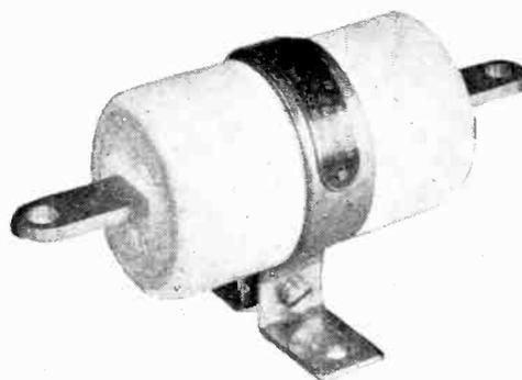
Fig. 8.—A 0.015 mfd. transmitting condenser selling at a popular price and made by the Dubilier Company. It is capable of passing 5 amps when used on 100 metre transmission.
