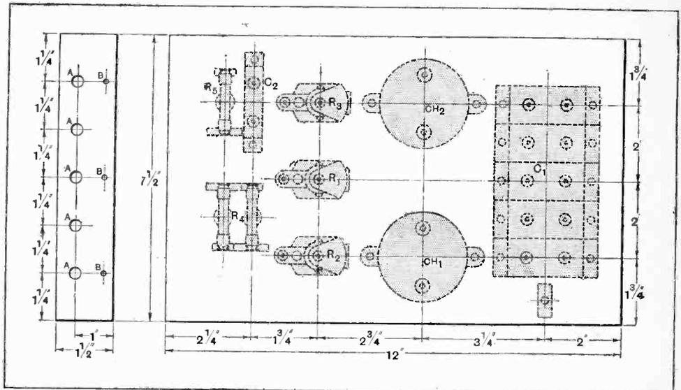
Fig. 7.—Layout of the parts of the D.C. eliminator and the terminal strip. The holes have the following diameters: A 5/16in. B 1/8in.
