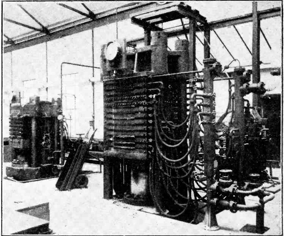
Fig. 5.—A steam-heated hydraulic press which exerts a pressure of 1/2 ton per square inch or an equivalent total weight of 800 tons. The treated paper sheets form a hard homogeneous substance which has excellent dielectric properties.
