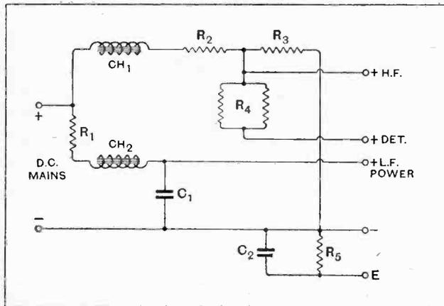
Fig. 3.—An eliminator for attachment to direct current mains for the "Everyman Four" receiver. Resistance  $R_1$  may be of 5000 ohms when the mains voltage is 240 and the full amount is not required across the L.F. and power valves. Values for resistances  $R_2$  and  $R_3$  are given in the text.  $R_4$  comprises two 0.5 megohm resistances in parallel, and  $R_5$  is of 0.25 megohm.
