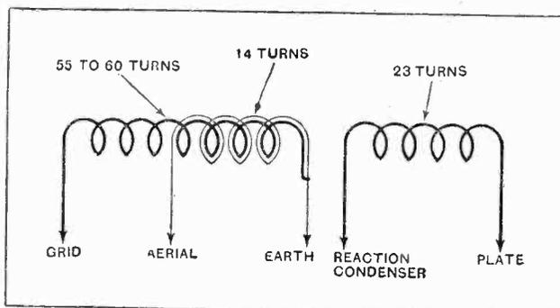
Fig. 5.—Particulars of the tuning coil windings which are supported on a "Becol" former 3in. in diameter and 6in. long.
