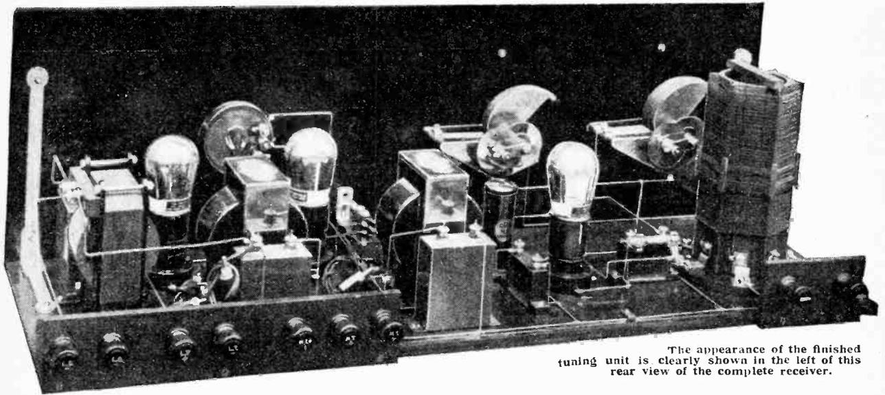
The appearance of the finished tuning unit is clearly shown in the left of this rear view of the complete receiver.
