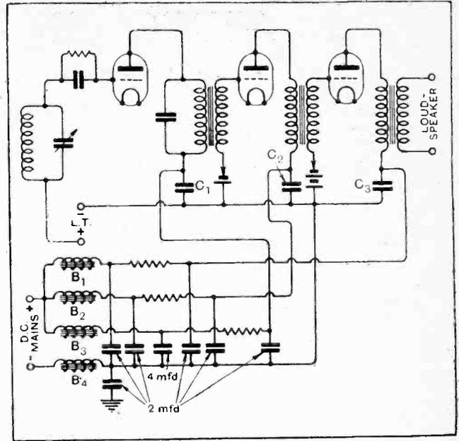
**Fig. 5.—The anode-feed resistance scheme as applied to a D.C. H.T. eliminator. The important claim is made that no "motor-boating" can occur and that the amplification curve is the same as in the ideal case where separate H.T. batteries are used for each anode**
