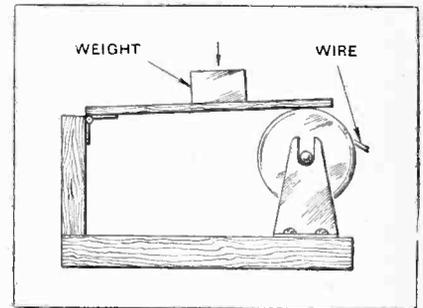
Friction device for coil winder.
