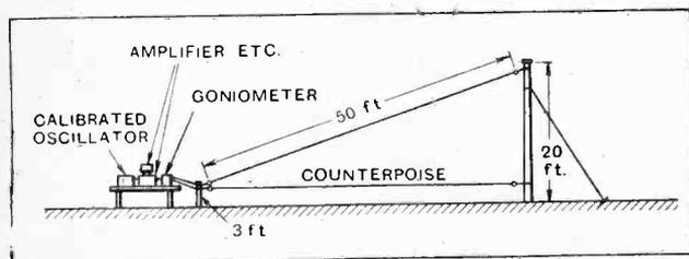
Fig. 3.—Dimensions of aerial and counterpoise system.
