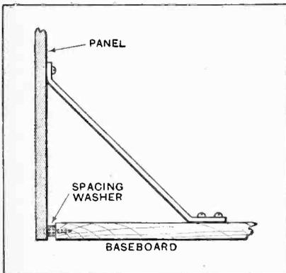
Panel spaced from baseboard to facilitate removal of surplus solder.
