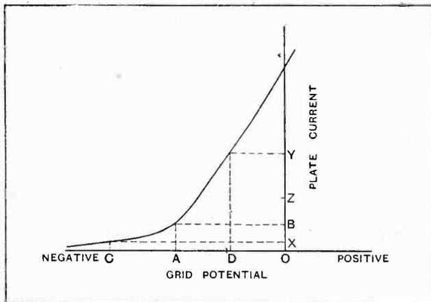
Fig. 1.—Rectification by anode bend. A positive displacement of grid potential at the bend in the curve increases the plate current more than an equal negative displacement decreases it, resulting in an increase in the mean anode current.
