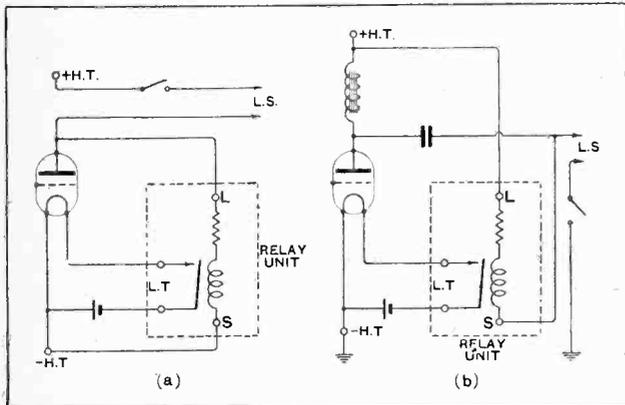
Fig. 3.—Circuit connections of the "Teletrol" system; (a) for loud-speakers connected directly in the anode circuit and (b) for choke-capacity output.
