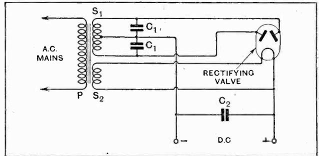
Fig. 5.—A rectifying unit. Condensers C<sub>1</sub> are of 0.1 mfd. each, and C<sub>2</sub> of 4 mfd.
