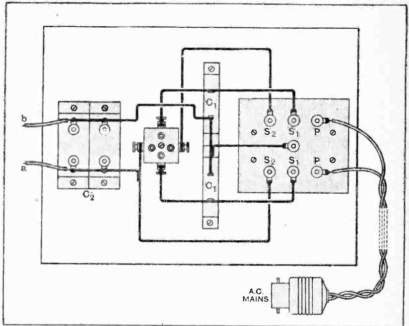
Fig. 11.—Wiring diagram. Wires a and b have to be connected to the input terminals a and b (fig. 9) of the D.C. eliminator.
