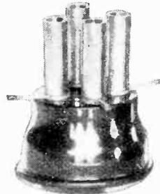
Valve base converted for use as a valve holder.
