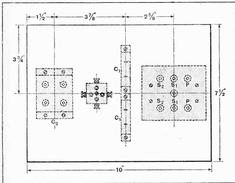
Fig. 10.—Layout of the parts for the rectifier.
