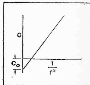
Fig. 2.—Graphical method of determining self-capacity.
