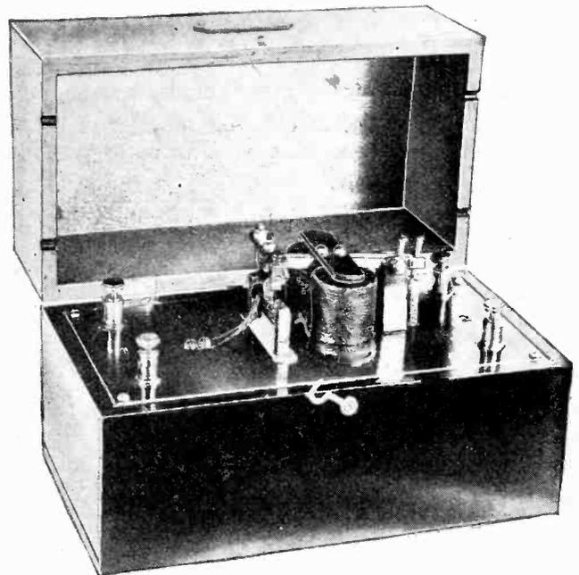
The "Gamage" relay has proved itself a reliable instrument for controlling L.T. current.
