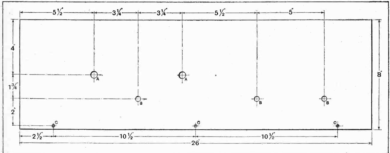
Fig. 6.—Dimensions of the panel. A, 1/2in. diameter; B, 3/8in. diameter; C, 1/8in. countersunk for No. 4 wood screws.
