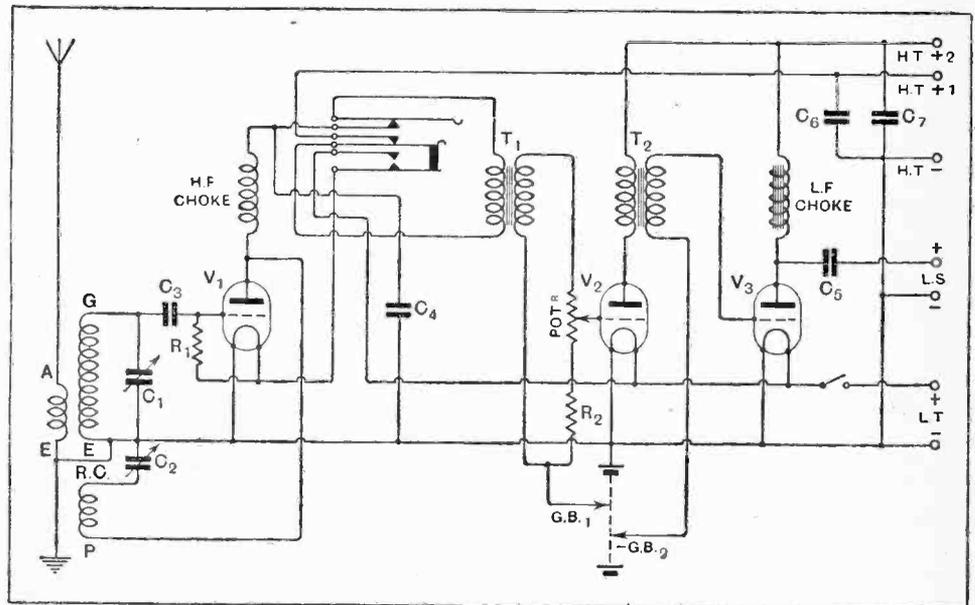
Fig. 1.—Complete circuit diagram.  $C_1=0.0005$  mfd.,  $C_2=0.0003$  mfd.,  $C_3, C_4=0.0003$  mfd.,  $C_5, C_6, C_7=2$  mfd.,  $R_1=2$  megohms,  $R_2=0.5$  megohm.
