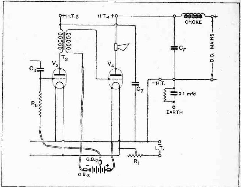
Fig. 2.—The last two valves of the "Everyman Four" with a filter showing how current may be supplied to the last valve from D.C. mains.
