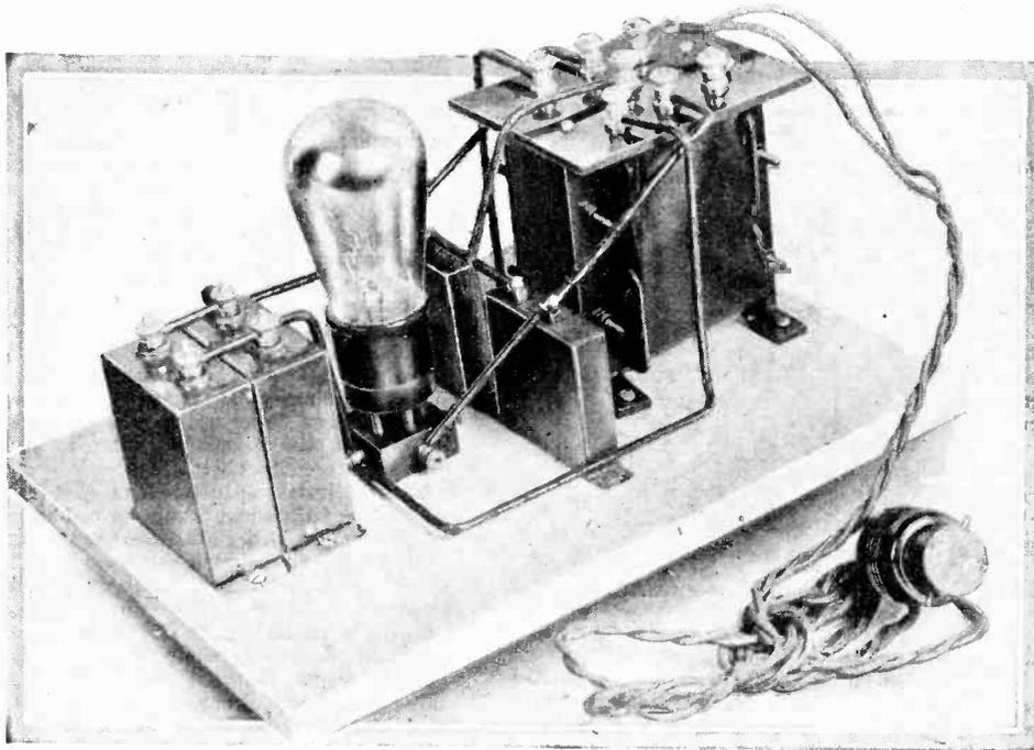
Fig. 12.—The completed rectifying unit with flex and adaptor.
