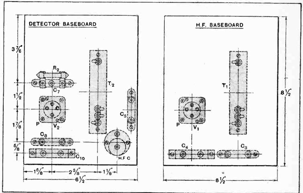
Fig. 4.—Arrangement of the parts in the two compartments of the copper box. These are fitted on wooden bases.
