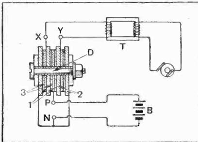
Section of dry contact rectifier and associated circuit. (No. 277,103.)
