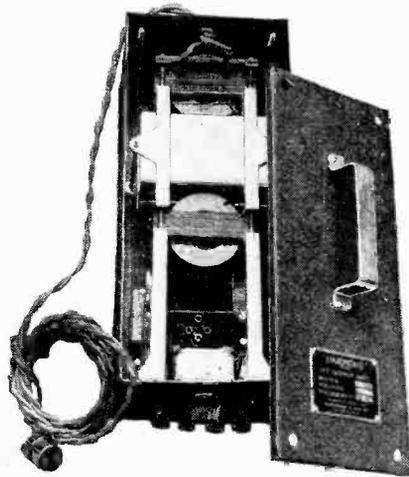
**Parmeko A.C. battery eliminator.** Its several components are supported in aluminium frames.
