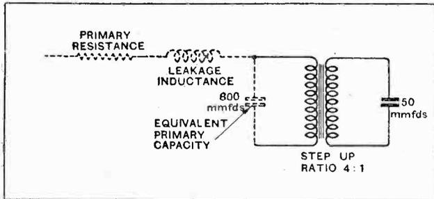
Fig. 6.—The equivalent primary capacity transferred from the secondary is increased as the square of the step-up ratio.
