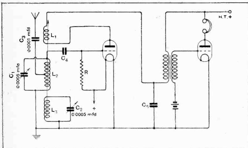
Fig. 2.—Rejector circuit for eliminating interference from the local station.
