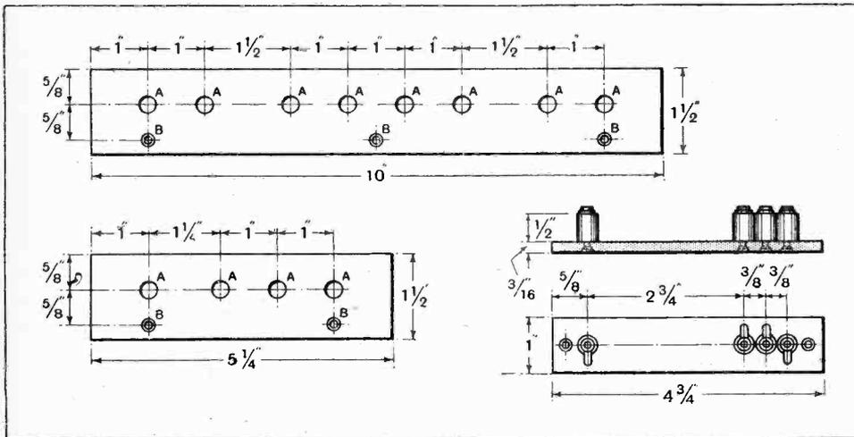
Fig. 3.—The terminal strips and coil base. A, 5/16in. diameter; B, 1/8in. countersunk for No. 4 wood screws. Two coil bases are required.
