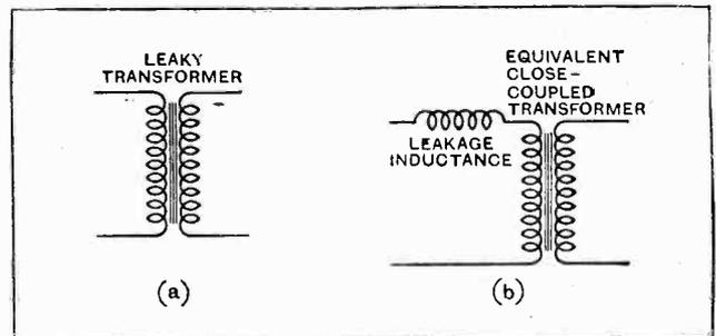
Fig. 5.—Transformer (a) with magnetic leakage, and (b), the equivalent circuit with leakage inductance referred to one winding.
