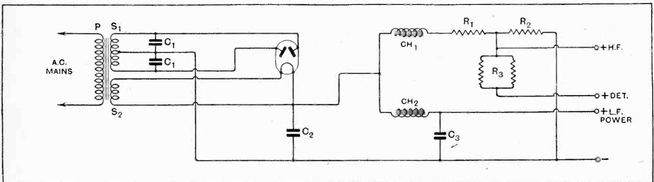
Fig. 6.—Connections of the complete eliminator for working off A.C. mains.
