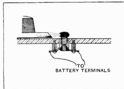
Method of fitting lamp socket for illuminating wavemeter dial.
