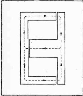
Fig. 4.—Iron core laminations of typical shape showing mean length of magnetic circuit.
