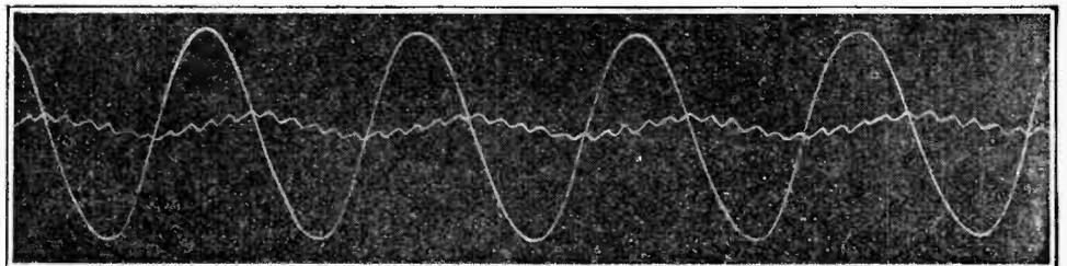
Fig. 4.—Oscillograph photograph of input and output waves of amplifier shown in Fig. 2 with common H.T. battery of 200 ohms D.C. resistance but without anode feed resistances. Note the reduced amplitude of output wave and the H.F. ripple superimposed.
