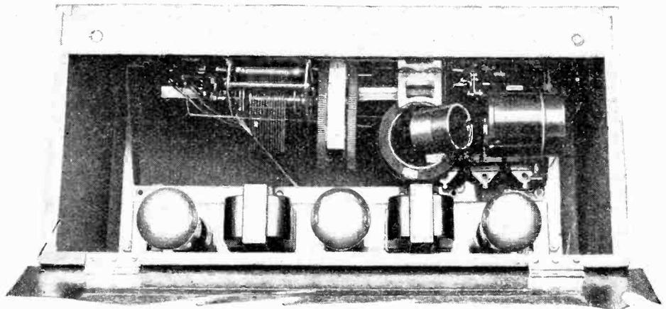
Plan view of interior from back of set; the tuning and reaction coils are assembled in the top right-hand corner.
