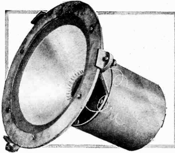
A completed loud-speaker. (The front projecting lugs are no longer provided as will be seen in the set of castings shown earlier.)
