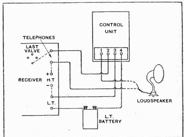
Fig. 4.—Connections of the Lissen "Telepathic" remote control relay.
