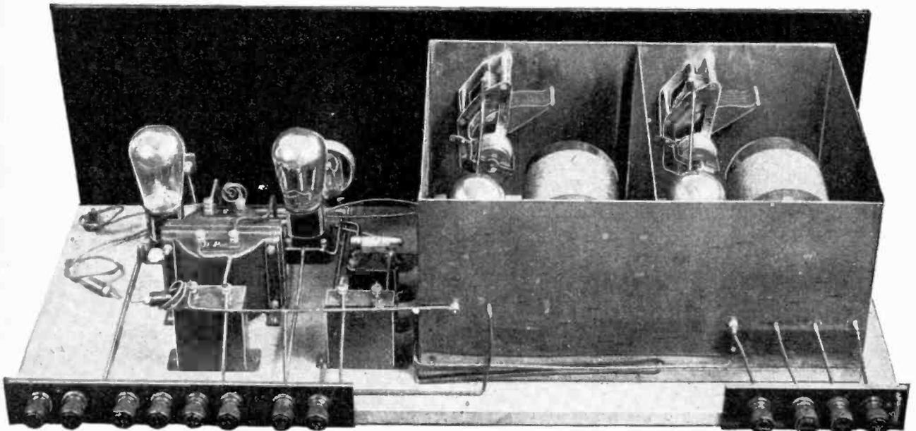
The finished set complete with coils and valves.
