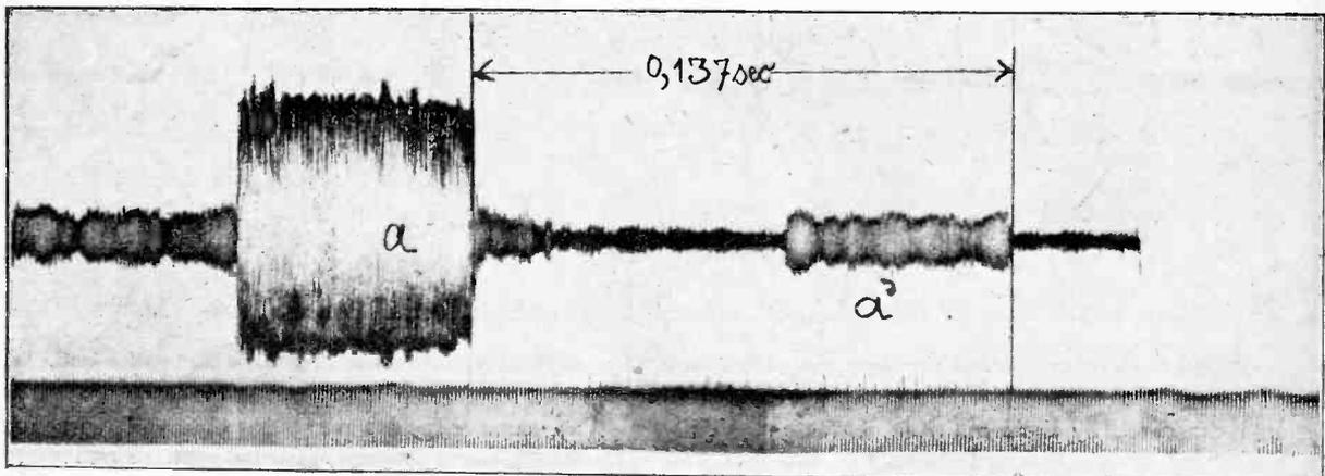
Fig. 1.—Oscillograph record of Morse "dot" sent from Rio de Janeiro on 15.66 metres and received at Geltow, Germany.
