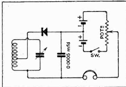
Fig. 2. Potentiometer connections giving positive or negative bias.
