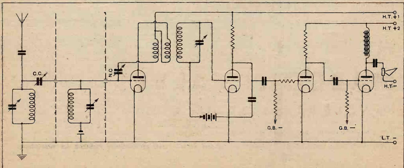
Fig. 2.—A "Wireless World Diary" circuit with two low-gain L.F. stages, modified by the addition of an H.F. amplifying valve.
