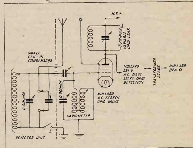
should be made of something like copper strip, and the condenser should have definitely low resistance connections, particularly to the rotor, and the leads to the inductance should be of heavy flex.
