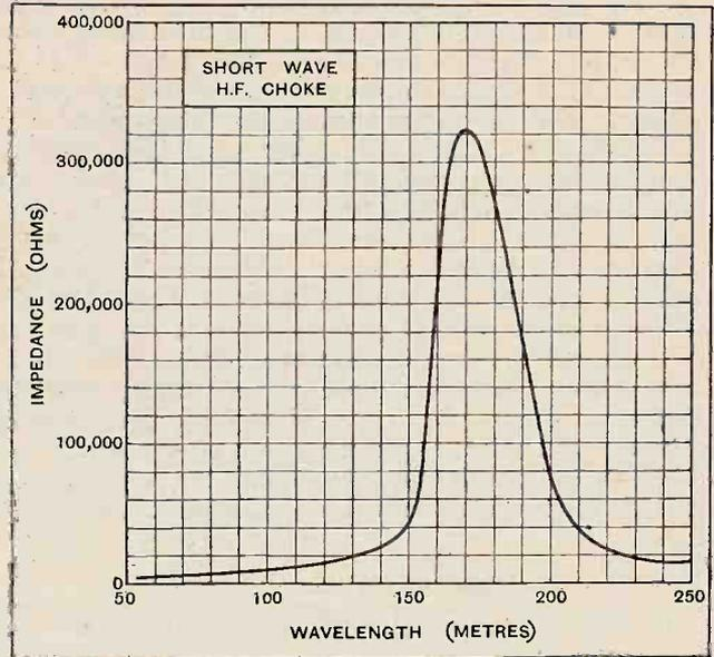
Fig. 2.—Impedance curve of a typical short-wave H.F. choke with a shunt capacity of 8  $\mu\mu\text{f}$ .
