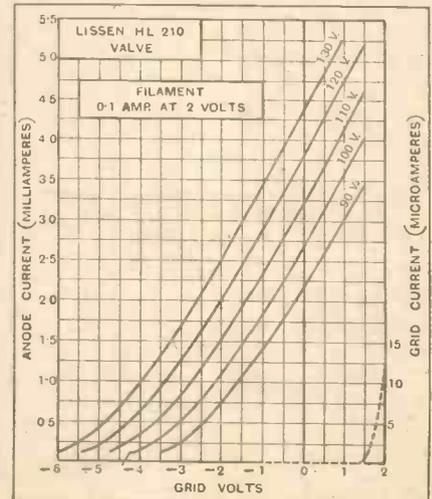
Average value under working conditions: A.C. resistance, 18,000 ohms; amplification factor, 16; mutual conductance, 0.9 mA/volt.
