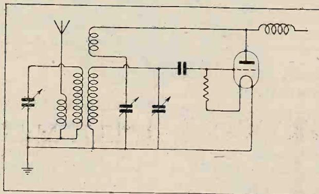
Fig. 1.—A filter circuit preceding a leaky-grid detector.
