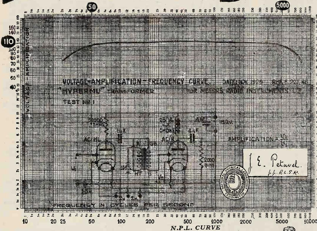
At the request of many interested users we are now publishing by the courtesy of the N.P.L. one of the latest "Hypermu" N.P.L. voltage amplification curves taken with the famous A.C.H.L. indirectly-heated Cosmos valves.
