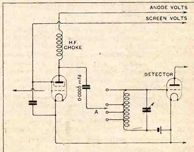
Fig. 4.—Tuned grid H.F. coupling, using tapped coil. By connecting the lead A to different tapplings, selectivity, amplification and stability can be varied until the best compromise is found.
