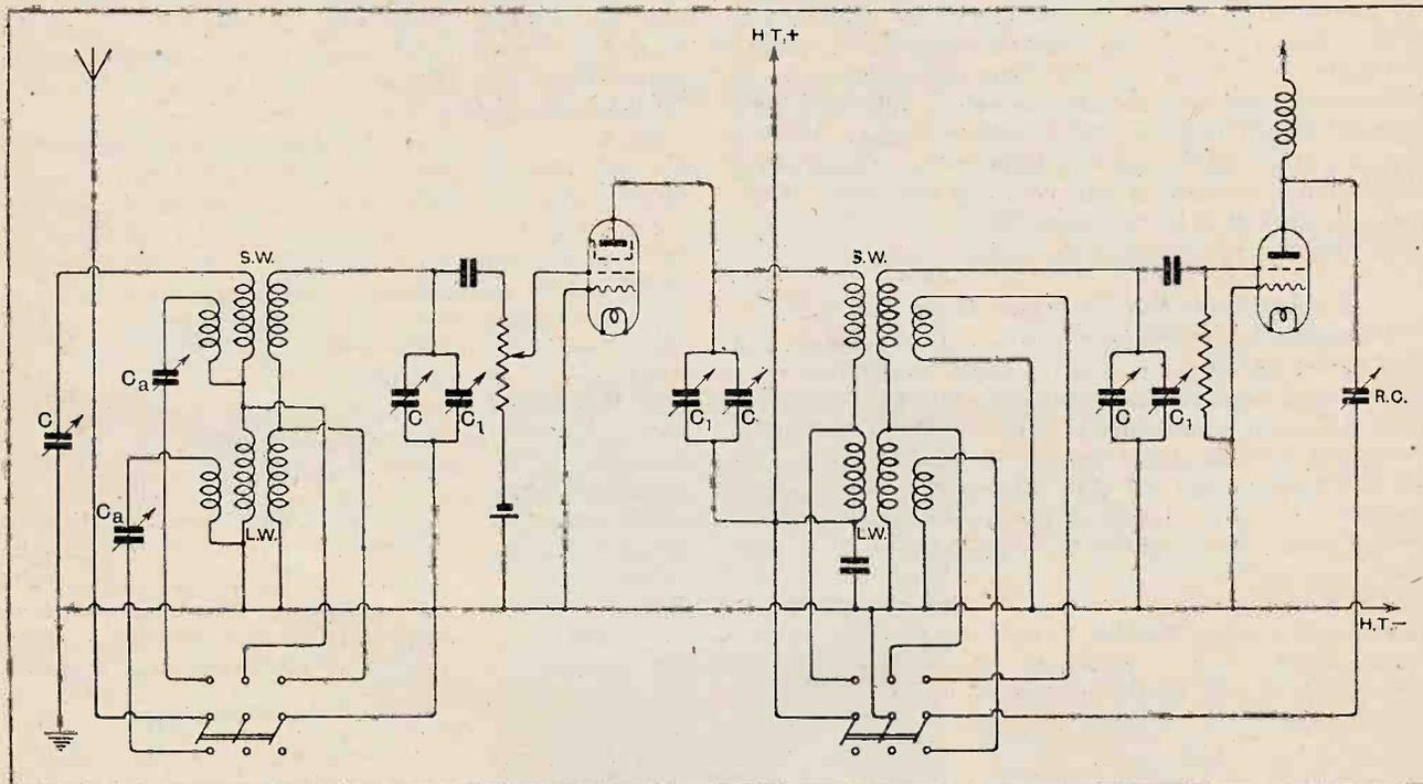
Fig. 7.—Circuit showing ganged filters, equalising condensers and a suggested method of waveband switching. C, ganged tuning condensers 0.00035 mfd.; C<sub>1</sub>, equalising condensers of 50 mmfd. and C<sub>a</sub> series aerial condensers.
