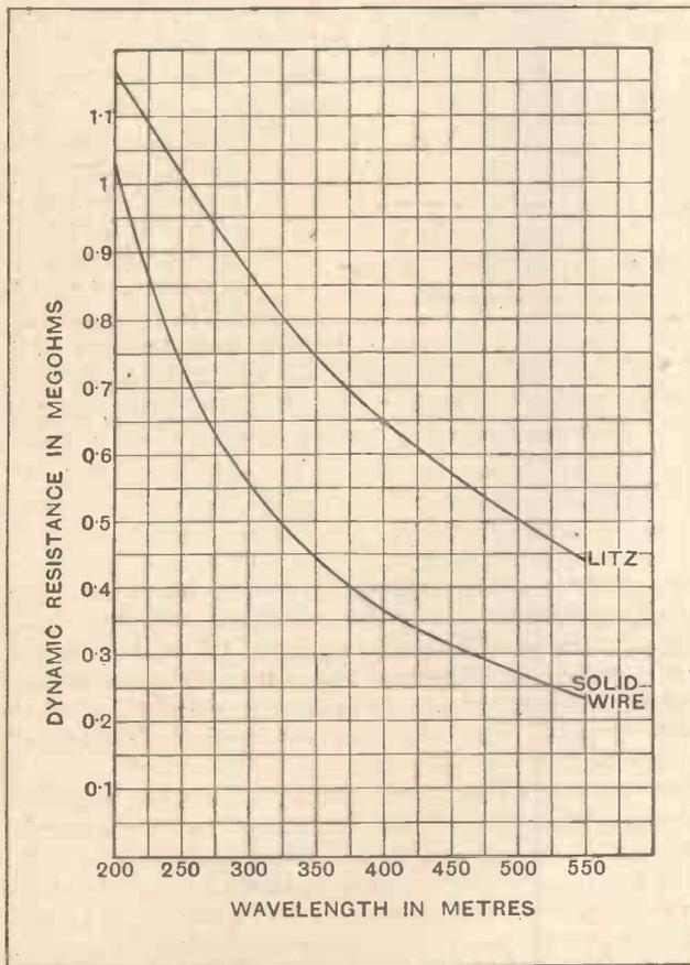
Fig. 2.—Theoretical dynamic resistance of tuned circuit, taking only the copper losses of the coil into consideration.
