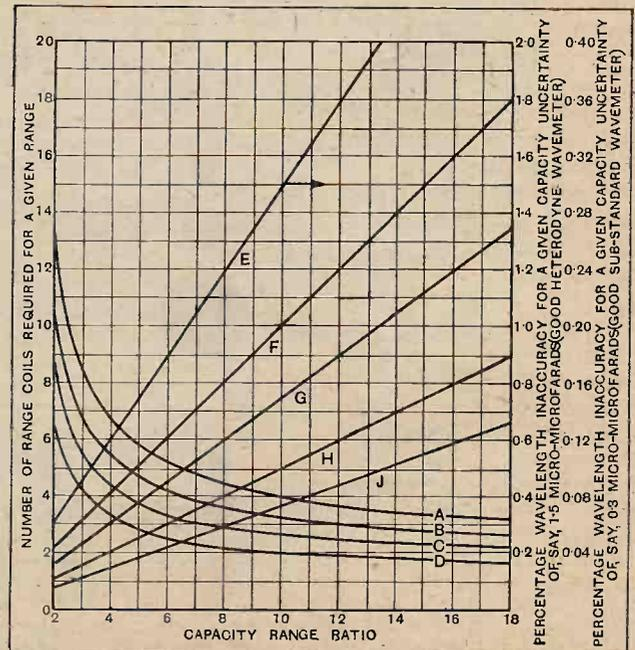
Fig. 3.—Showing the number of range coils and capacity ratio of condensers of wavemeters of various accuracies.
