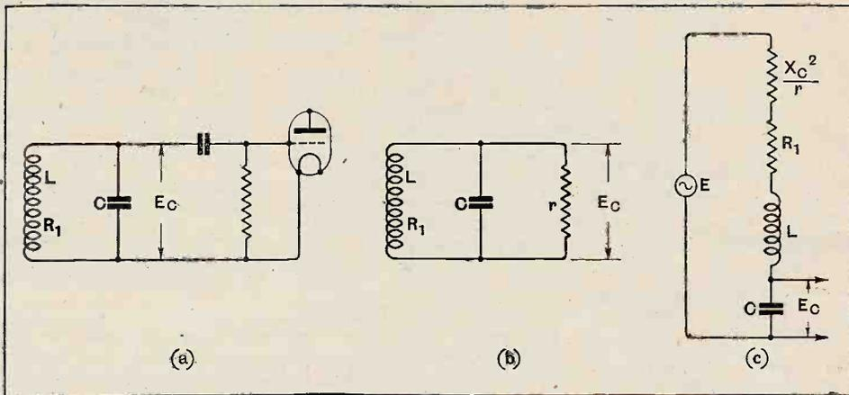
Fig. 3.—When a tuned high-frequency circuit feeds a leaky grid detector it is shunted by an equivalent resistance  $r$  as shown in (b). This in turn is equivalent to adding an extra resistance  $\frac{X_c^2}{r}$  in the tuned circuit itself.
