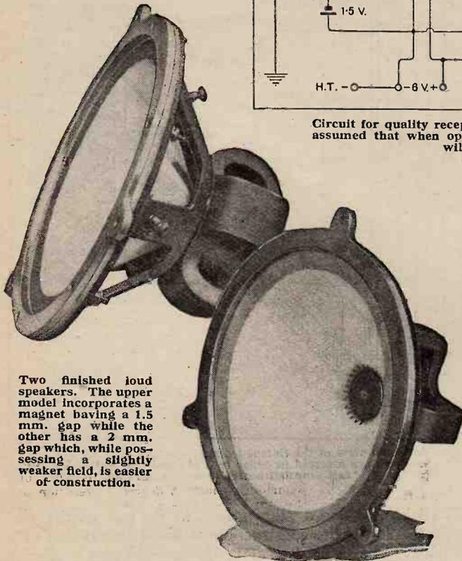
Two finished loud speakers. The upper model incorporates a magnet having a 1.5 mm. gap while the other has a 2 mm. gap which, while possessing a slightly weaker field, is easier of construction.
