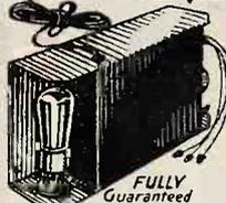
Designed for use with Portables, or Sets with outside aeriars. Variable Detector Tapping adjustable to any set. Full wave rectification with Philips type 1801 valve, giving output of 25 M.A. at 120 volts. This output is greater than that of most eliminators on the market. Saving at least £3 per year in high tension batteries—Coates' Eliminator is a sound investment and ensures consistently good reproduction with wider range and greater volume. Specially made and very neatly finished in blue.
