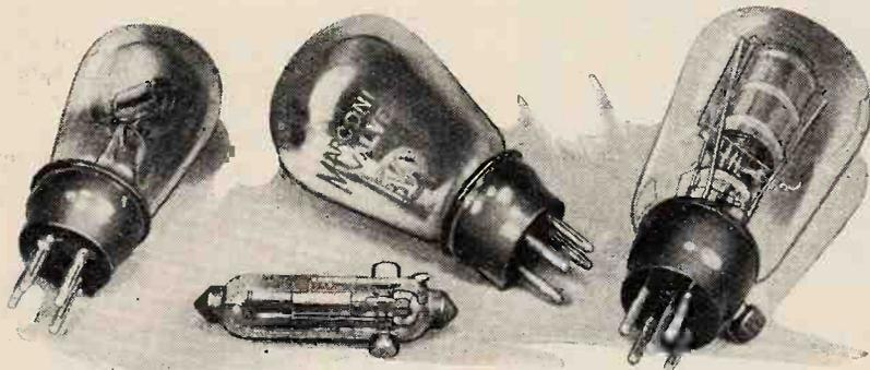
The Marconi-Osram QX, seen in the foreground, was one of the earliest special detector valves designed for anode rectification, and is shown in contrast with the Mazda A.C./Pen., a recently developed valve suitable for super power-grid detection. The DER and DE5B valves, also shown in the illustration, were other very popular types used for rectification.
