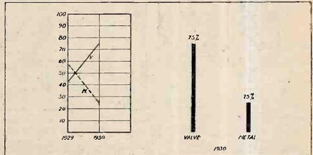
The valve is now the most favoured form of rectifier in A.C. power supply units.
