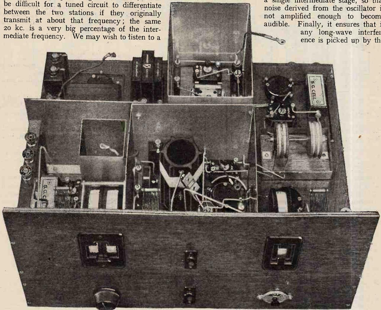
Three-quarter plan view with covers of screening boxes removed. Note the method of mounting the I.F. band-pass transformer.
