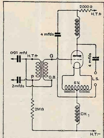
Fig. 1.—"The Wireless World Four" output stage with a triode in place of the original pentode.
