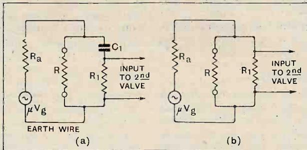
Fig. 2.—A.C. circuits equivalent to the interval circuit of Fig. 1 at low frequencies (a) when the reactance of the coupling condenser  $C_1$  is comparable with  $R_1$  and (b) when the reactance of  $C_1$  is negligibly small compared with the grid leak resistance  $R_1$ .
