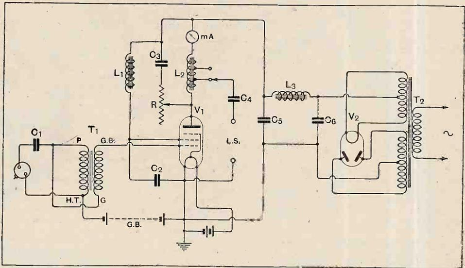
One-valve gramophone amplifier circuit on the lines of the Regional-One receiver.  $C_1$ , 0.05 mfd.;  $C_3$ , 0.01 mfd.;  $R$ , 30,000 ohms;  $C_2$ , 8 mfd.; G.B., 22 volts negative;  $V_1$ , PM24A and  $V_2$ , U5.
