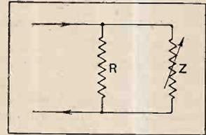
Fig. 3.—In this simplified diagram Z stands for the varying impedance of a moving-iron loud speaker while R is a compensating resistance.
