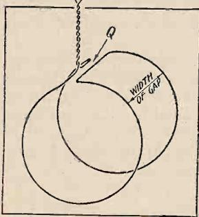
Fig. 4(b).—Alternative form of single turn differential coil. The space Q is left merely to show the construction of the coil.
