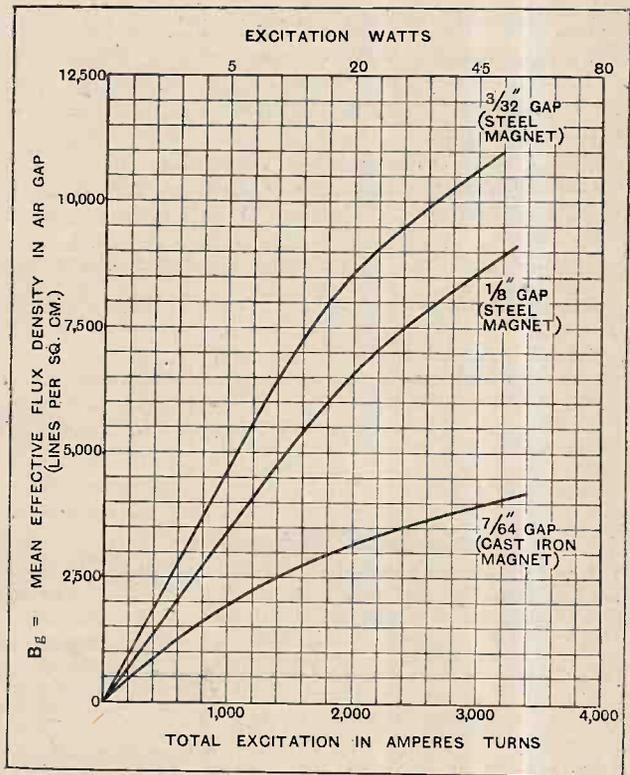
Fig. 7.—The effective flux density obtained in the air gap plotted against the excitation in ampere turns showing how the flux density varies with reduction in the length of the gap. Remanence has been neglected.
