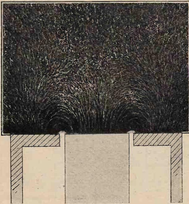
Fig. 2.—Photograph showing the external leakage and flux distribution of the magnet given in Fig. 1. The gap is 1/16 in. and the field distribution obtained is that which results before applying excitation.
