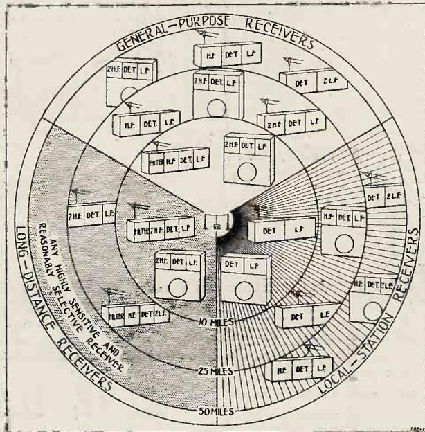
Sets for various localities and requirements. The effects of poor receiving conditions are taken into account by allowing an ample margin of sensitivity.
