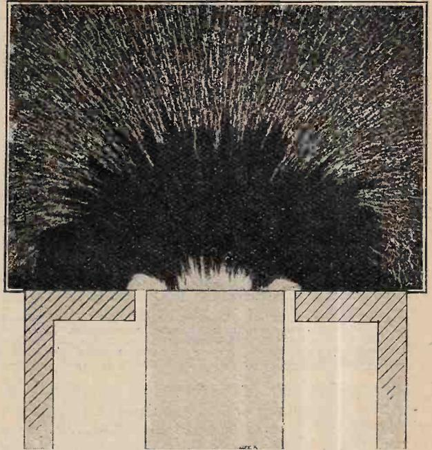
Fig. 3.—External leakage flux distribution with full excitation.
