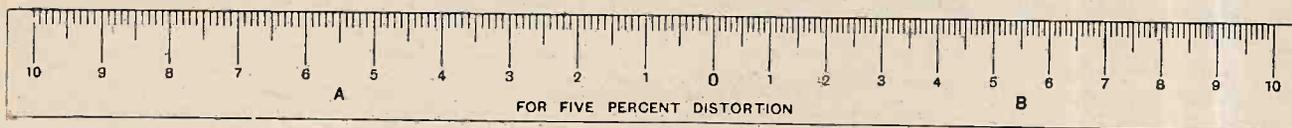
Fig. 1.—The five per cent. distortion scale in which the divisions on the right of zero are 9/11th of those on the left.
