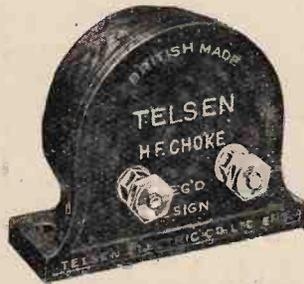
**TELSER H.F. CHOKES.** Designed to cover the whole wave-band range from 18 to 4,000 metres, extremely low self-capacity, shrouded in genuine Bakelite. Inductance 150,000 micro-henries. Resistance 400 ohms. Price 2/6 each.
