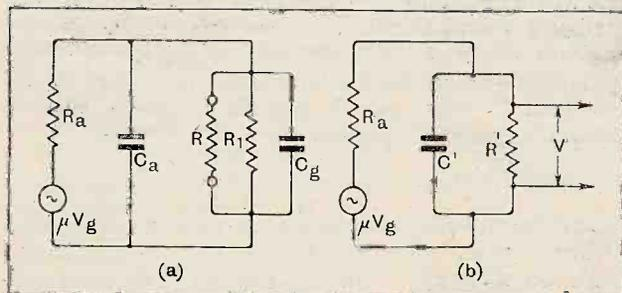
Fig. 3.—A.C. circuits equivalent to the intervalve circuit of Fig. 1 at high frequencies, showing the effect of the internal valve capacities. In (b)  $C'$  stands for  $C_a$  and  $C_g$  in parallel and  $R'$  for  $R$  and  $R_1$  in parallel.
