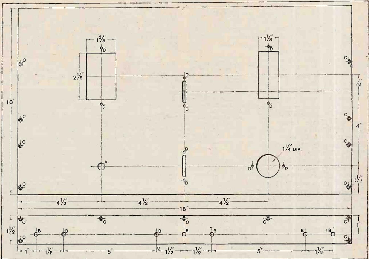
Drilling details of the front panel and the terminal strip. Sizes of holes are as follows: A, 1/4 in. dia.; B, 7/32 in. dia.; C, 1/8 in. dia.; countersunk for No. 4 wood screws; D, 1/8 in. dia.
