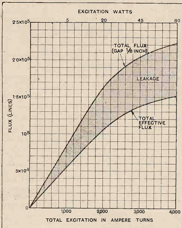
Fig. 6.—Total useful flux compared with the total flux plotted against excitation in ampere turns.
