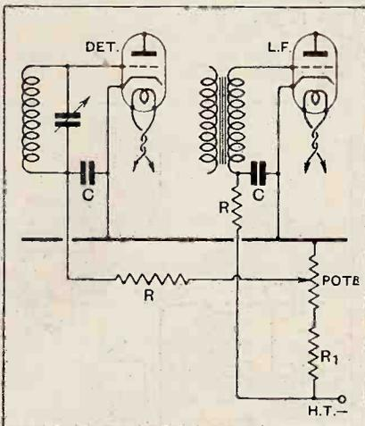
Fig. 1.—Variable "automatic" bias for an anode bend detector.
