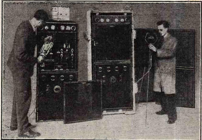
A COMPACT AMPLIFIER. Testing a Philips 500-watt amplifier which gives an output of  $1\frac{1}{2}$  kW. The engineer on the left is inserting a valve which takes a plate voltage of 4,000. The microphone on the right is similar to those in use at Hilversum and PCJ.
