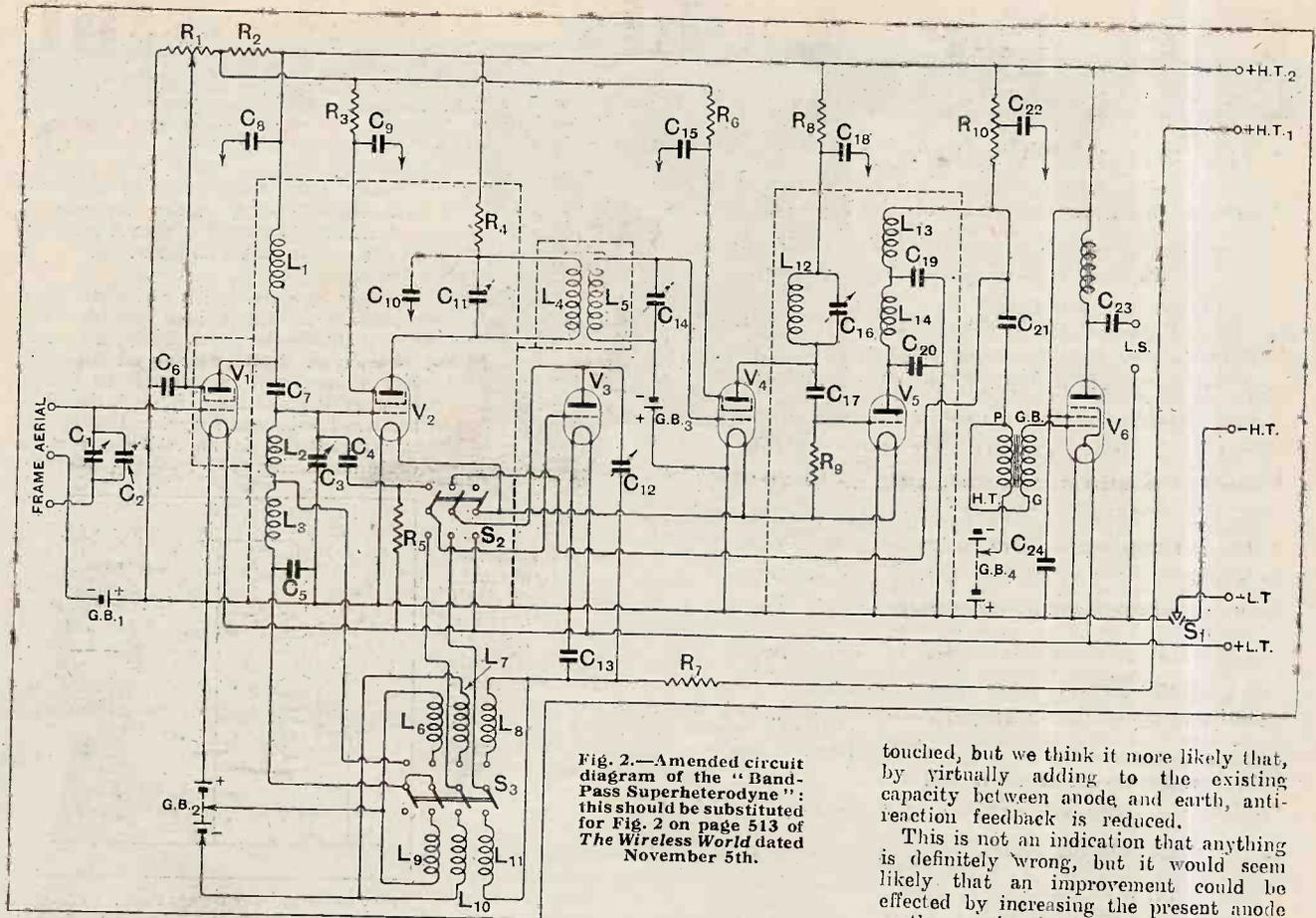
Fig. 2.—Amended circuit diagram of the "Band-Pass Superheterodyne": this should be substituted for Fig. 2 on page 513 of *The Wireless World* dated November 5th.
