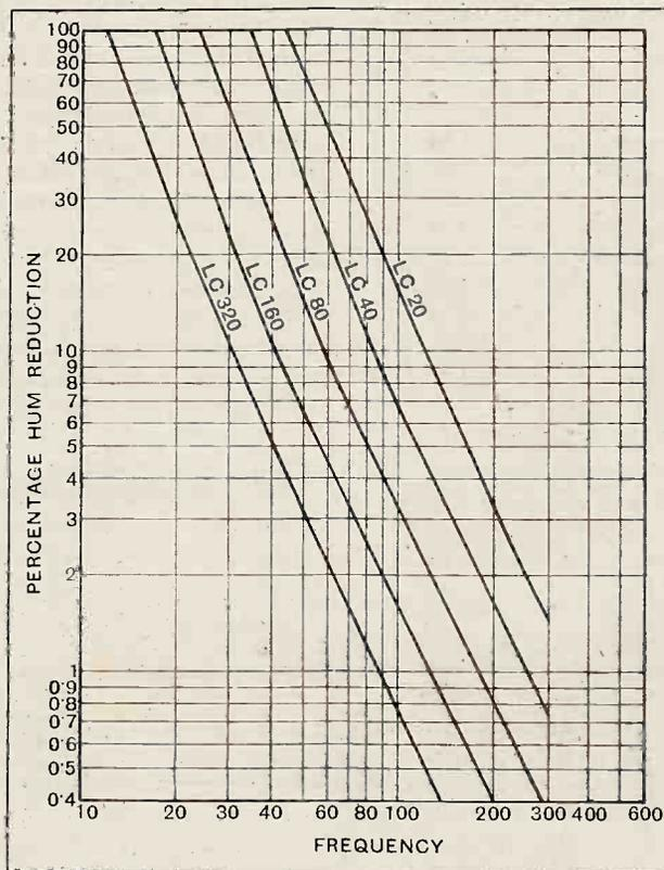
Fig. 3.—The approximate smoothing obtainable with any combination of inductance and capacity can be read off from these curves; the figures marked against each curve refer to the product of inductance in henrys and capacity in microfarads for that curve.
