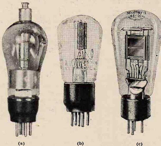
Typical H.F., detector and power output valves. (a) Mazda AC/SG with low interelectrode capacity, medium A.C. resistance and comparatively large grid swing acceptance which minimises cross-modulation. (b) Marconi and Osram MH4—an excellent power-grid detector giving less than 2 per cent. harmonic distortion. (c) The Mullard ACO44 directly heated A.C. power valve with 4.0 volt 1.0 amp. filament and an A.C. output of over 1 watt.
