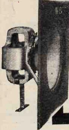
The new W.B. Permanent Magnet Moving Coil Speaker employs a Sheffield-made Cobalt Steel Magnet weighing 10½ lbs. Guaranteed for five years, it needs no energising from the mains, so that mains hum due to field windings cannot occur.
