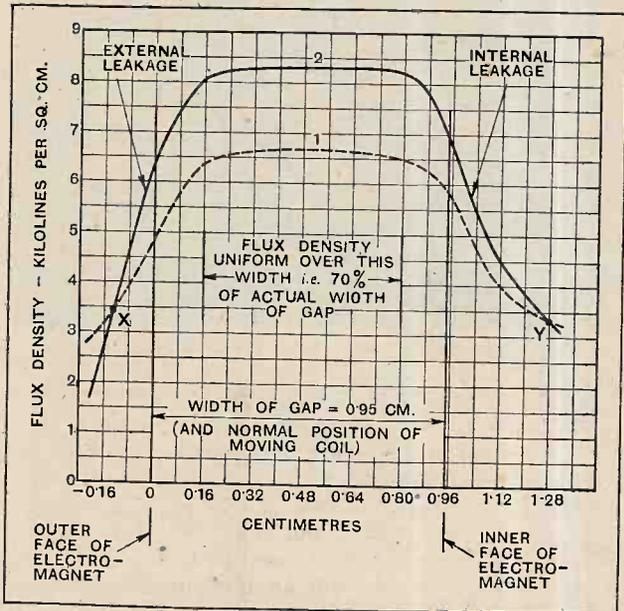
Fig. 5.—Diagram showing actual distribution of flux in air gap of electromagnet of Fig. 1. Curve 1 is for a gap of 1/8 in. (0.32cm.) and curve 2 for a gap of 3/32 in. (0.24cm.). It should be observed that the leakage with the smaller gap falls below that for the larger gap at the points XY.
