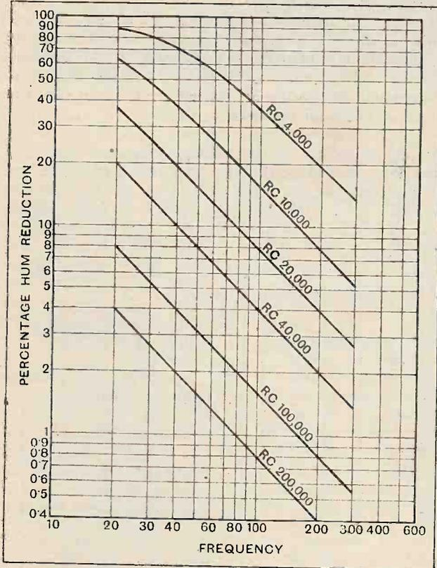
Fig. 4.—The smoothing given by a resistance-capacity circuit can be seen from these curves; the figures marked against each curve refer to the product of resistance in ohms and capacity in microfarads for that curve. The relative efficacy of various decoupling circuits can also be seen.
