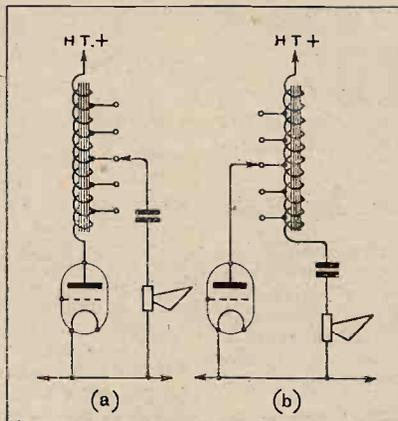
Fig. 1.—A tapped choke may be arranged as (a) a step-down or (b) a step-up coupling between the output valve and the loud speaker.
