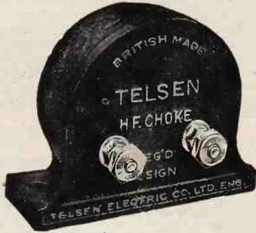
**TELSEN H.F. CHOKES**, designed to cover the whole waveband range from 18 to 4,000 metres. Extremely low self capacity, shrouded in genuine Bakelite. Inductance 150,000 microhenries, resistance 400 ohms.
