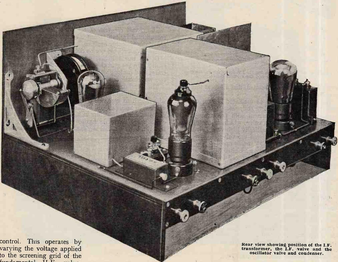
Rear view showing position of the I.F. transformer, the I.F. valve and the oscillator valve and condenser.
