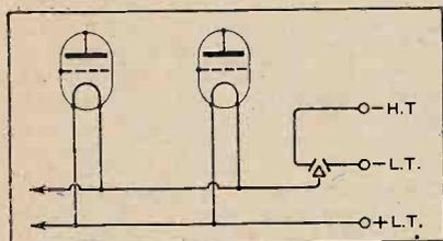
Fig. 1.—Connections of a three-point switch: both H.T. and L.T. battery circuits may be interrupted.
