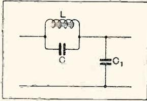
Fig. 6.—A special tuned smoothing circuit; the parallel tuned circuit L and C has a very high impedance at resonance, and at this frequency the smoothing is exceptionally good.
