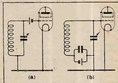
Fig. 2.—Methods of biasing an H.F. valve.
