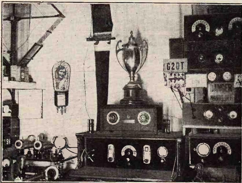
G2DT, owned and operated by Mr. E. T. Somerset at Dorking, Surrey. In the centre is the 7, 14 and 28 MC receiver with Reinartz-Grebe circuit and a screen-grid detector. On the receiver stands the frequency-monitor supporting the Wortley-Talbot challenge cup awarded by the R.S.G.B. in 1929-30 for early work on 5 metres. The transmitters comprise one for 56 MC, one TP.TG for 14 MC, and on the right is seen the 7 MC Hartley transmitter and a 28 MC 1-V-1 receiver.
