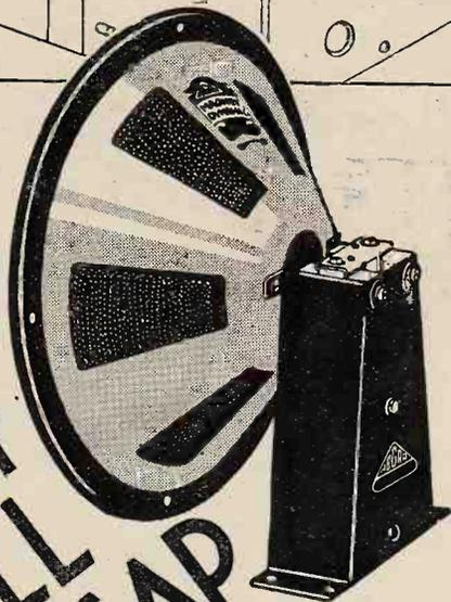
THE special design of the magnet system in the new Hegra Magnet-Dynamic Speaker, enables a very small uniform air gap to be employed. This, together with pole shoes specially shaped to give a compensated field, ensures uniformity of armature response. At the same time, it is impossible for the armature to come into contact with the pole-pieces.
