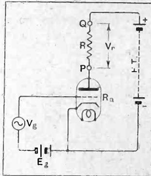
Fig. 1.—When a non-inductive resistance  $R$  is connected in the anode circuit of a valve, the theoretical value of the voltage amplification obtained is  $\mu \frac{R}{R + R_a}$  where  $\mu$  is the amplification factor of the valve and  $R_a$  is its A.C. resistance.
