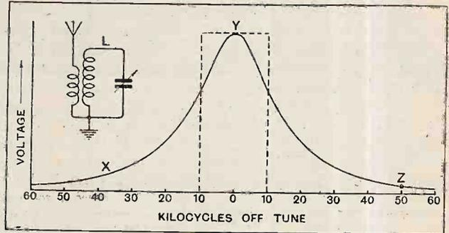
Fig. 2.—The voltage developed on the grid of the S.G. valve by Z, a station 50 kilocycles away from resonance may be sufficient to cause cross-modulation when the response curve of the input circuit is like XYZ. If the pre-H.F. volume control is adjusted until all traces of cross-modulation disappear it is possible that the voltage developed by the desired station will have become excessively small.
