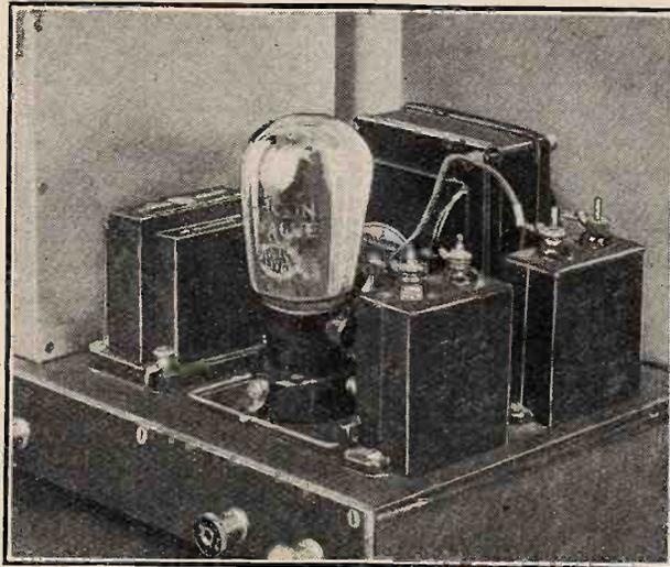
Showing the pentode output arrangement of "The Wireless World" Band-Pass Superheterodyne, a set recently described in this journal.
