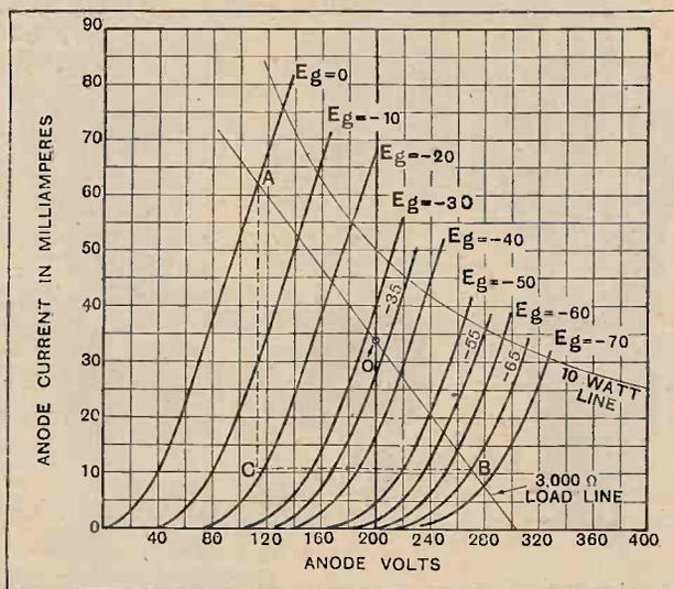
Fig. 2.—Anode volts-anode current curve of a typical power output triode where the watts dissipation limit is 10. If the zero of the distortion scale is placed on 0 (–32½ grid volts) the same reading in the scale is obtained at zero and –65 grid volts. From the points A, B and C, the optimum load and undistorted output can easily be calculated.
