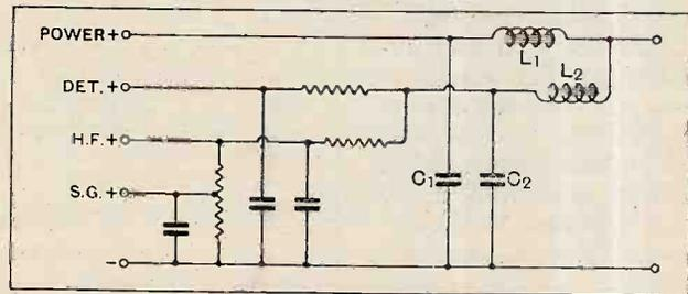
Fig. 5.—A form of smoothing circuit which introduces less feed-back than other types, but which may require more apparatus than the circuit of Fig. 2.
