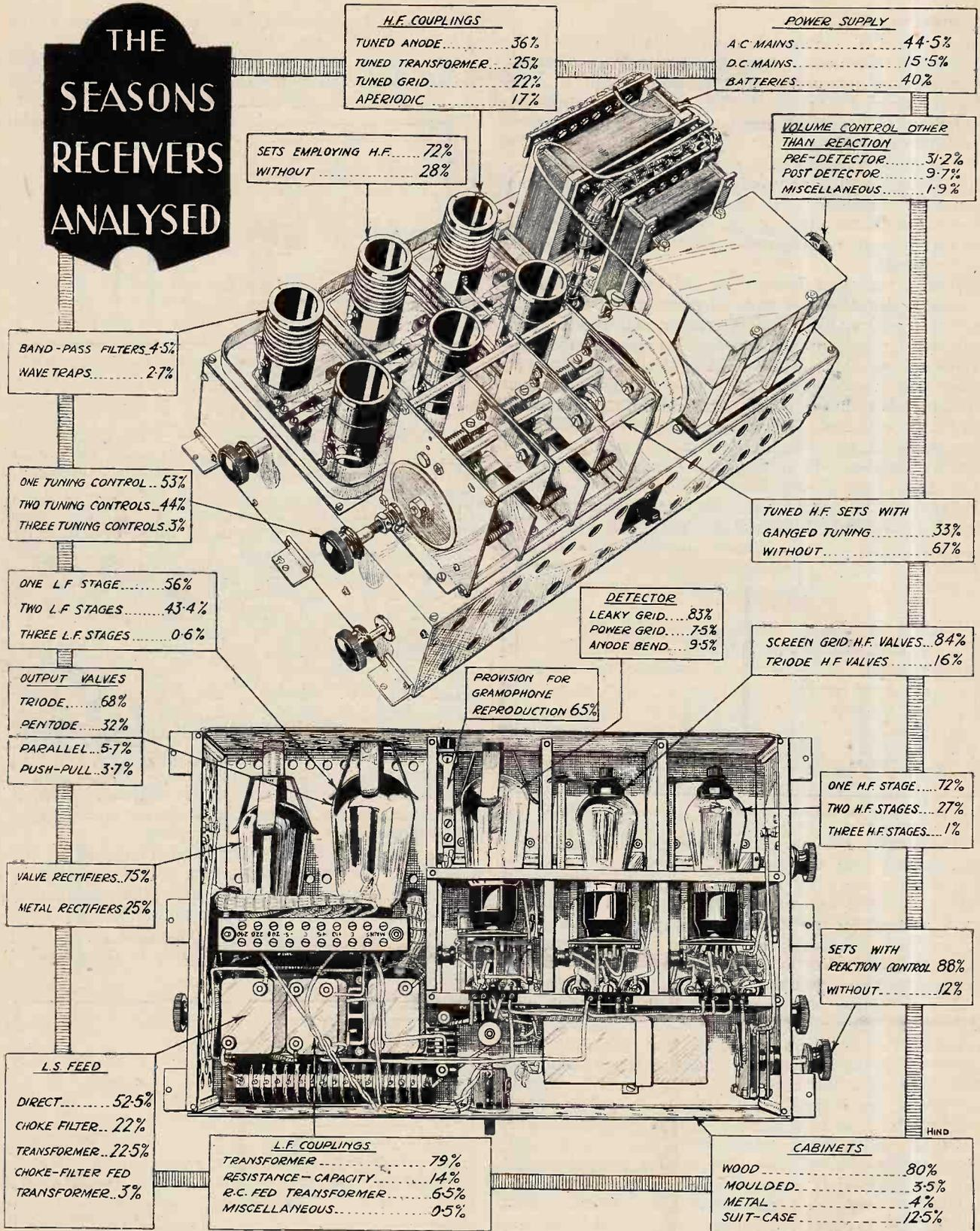
A typical 1930-31 receiver chassis showing the details of specification most favoured by modern practice. [The chassis reproduced above is the Gecophone All Mains Four.]
