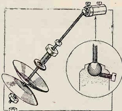
Weedon's "Self-centre," fitted with adjustable spindle for use on linen diaphragms.
