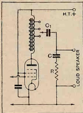
Fig. 4.— Output circuit (tapped choke) for pentode with moving-iron speaker.  $C_1 = 2$  mfd.,  $R = 10,000$  ohms,  $C = 0.01$  mfd. These last two values are subject to considerable variation to suit the speaker.
