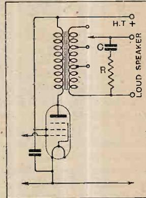
Fig. 5.— An equivalent circuit to that of Fig. 4, using a multi-ratio transformer in place of a tapped choke.
