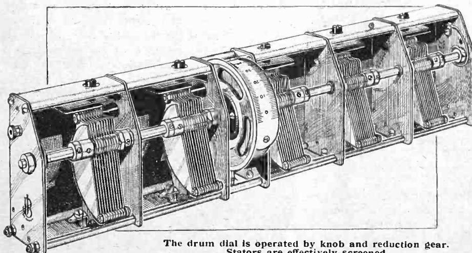
The drum dial is operated by knob and reduction gear. Stators are effectively screened.
