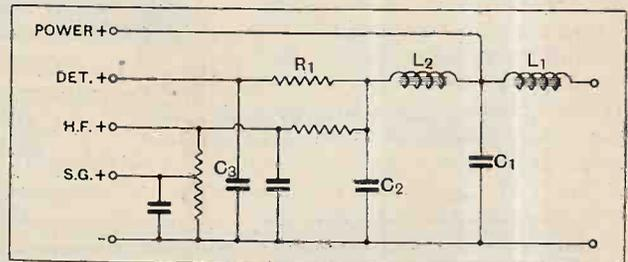
Fig. 2.—A series proportional smoothing circuit; with high amplification  $R_1, C_1$  must be large to avoid feed-back, but if push-pull be used  $R_1$  and  $C_3$  can be omitted.
