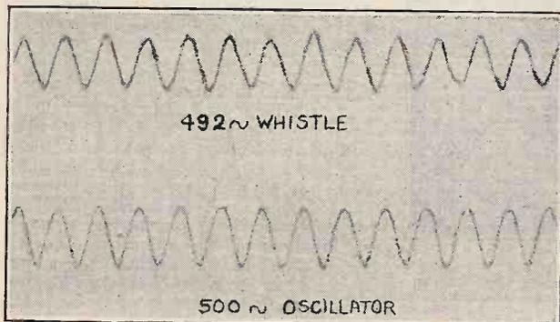
Oscillogram showing frequency and wave form of lowest whistled note obtained by G. A. V. Sowter, B.Sc., A.M.I.E.E.
