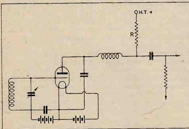
Fig. 1.—The anode detector has the merit of needing only a small anode current, and there is also little risk of hum. It does not give the best quality, however.
