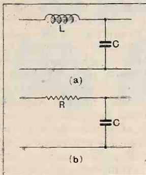
Fig. 1.—The simplest choke-capacity smoothing circuit (a). A resistance-capacity smoothing circuit, more usually known as a decoupling circuit, is given in (b).
