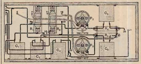
Note that the wires carrying raw A.C. are twisted together.
