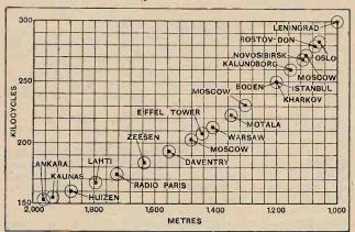
The above diagram has been prepared to illustrate the letter from the Chief Engineer of the B.B.C. The positions of most of the principal long-wave stations are indicated with their kilocycle separation. The circles drawn round each station are intended to indicate the spread, the width on either side of the carrier being taken as 5 kc.
