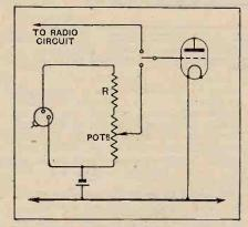
Fig. 1.—By connecting a fixed resistance in series with the controlling potentiometer, the maximum value of gramophone reproduction may be reduced to any desired extent.
