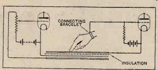
Fig. 3.-Volume control by the resistance of the human body.
