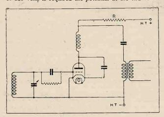
Fig. 1.—The usual resistance - transformer coupled power detector circuit. With an AC/HL valve, the best value for R is 20,000 ohms.
