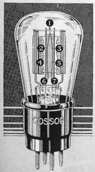
Cossor 210 DET., 2 volts, .1 amp. Impedance 13,000. Amplification Factor 15. Mutual Conductance 1.15 m.a./v. Normal working Anode Voltage 90-150.
