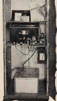
Fig. 4.—Arrangement of the central receiving station (experimental model). In the screened cupboard; short-wave band filter, broadcast receiver, and (below) high-frequency power amplifier.
