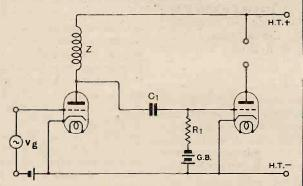
Fig. 1.—Connections for choke-capacity coupling.
