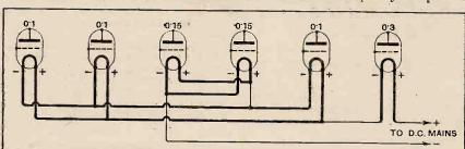
Fig. 2.—Series-parallel filaments. Each group (connections shown in heavy lines) consumes 0.3 amp. Polarity and current consumption of individual valves are indicated.
