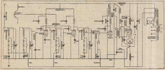
The circuit of The Wireless World Four. Even with a weak signal rectification occurs in the H.F. stages to a sufficient extent to produce L.F. oscillation unless L.F. decouplings are introduced into the anode circuits. The I megohm biasing feed resistances increase the negative bias as soon as the S.G. valves and the consequent cross modulation of carriers that gives rise to an apparant flatness of tuning met with when using screen grid H.F. stages without an ærial filter.
