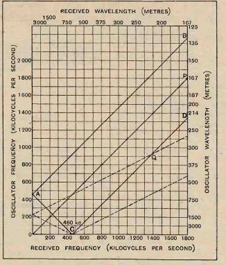
Fig. 2.—Relationship between received and oscillator frequencies for a superheterodyne using an intermediate frequency of 460 kc. (Kramolin.)
