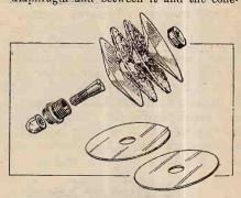
Tonax cone adaptor with felt fixing washers.
