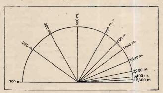
Fig. 4.—How the wavelengths fall on the oscillator tuning dial of a superheterodyne receiver of the "Infradyne" type. The whole tuning range is covered on a single swing of the condenser and the tuning is true "kilocycle tuning." At all points two stations removed by 9 kc. in frequency are separated by a shade over one degree on the dial.
