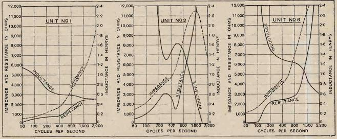
Fig. 9.—Graphs showing the variations in the effective values of resistance and inductance for the units numbered (1), (2) and (6) in Fig. 8.
