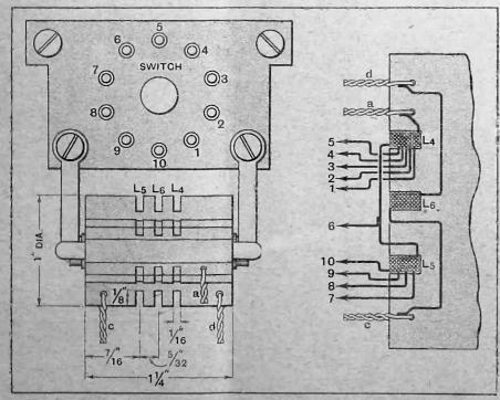
Fig. 3.—Construction and mounting of the coupling and reaction coils. The enlarged sectional diagram shows how the coils are wound; tappings are joined to similarly numbered switch studs, and terminal points bear reference lettering corresponding to the other diagrams.
