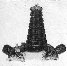
Tunewell H.F. choke, in which the sections are wound in alternate wide and narrow slots, and examples of new type push-pull switches. These components are made by Messrs. Turner and Co., Station Road, Old Southgate, London, N.11; the H.F. choke is priced at 6s. 6d., and the two- and three-point switches cost 1s. and 1s. 3d. respectively.
