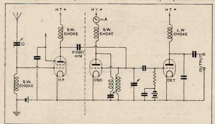
Fig. 2.—An aperiodic H.F. stage for the "Superheterodyne Short-wave Adaptor." Extra apparatus is shown on the left-hand side of the dotted line.
