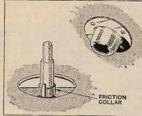
Friction collar on the turntable spindle of the B.T.H. motor.
