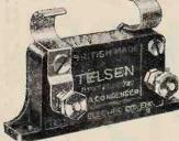
TELSEN FIXED (MICA) CONDENSERS, Shrouded in genuine Bakelite, made in capacities up to .002 m.f. Pro. Pat. No. .20287/30. .003 supplied complete with patent Grid Leak Clips to facilitate series or parallel connection. Can be mounted upright or flat. Tested on 500 volts. Price I/- each
