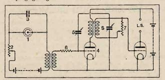
Fig. 1.—An experimental arrangement in which changes of frequency can be made in the Neon circuit and in the circuit marked S.
