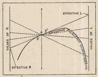
Fig. 7.—Alignment method of deriving effective values of L and R by means of the tangent to the impedence-frequency characteristic. The vertical line for frequency f is alone shown passing through P, the rest of the network heing omitted.
