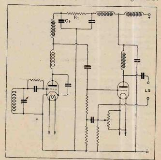
Fig. 4.—A satisfactory circuit with a single output valve; owing to the low amplification, feed-back effects are very small. The resistance R<sub>1</sub> should have a value of 8,600 ohms, with a 200 volts H.T. supply, and the condenser C<sub>1</sub> a capacity of frem 2 mfd, to 4 mfd.
