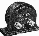
FELSEN H.F. CHOKE. Designed to cover the whole wave-band range, from 18 to 4,000 metres. Extremely low self-capacity, shrouded in Genuine Bakelite. Inductance 150,000 microhenries, resistance 400 ohns.
