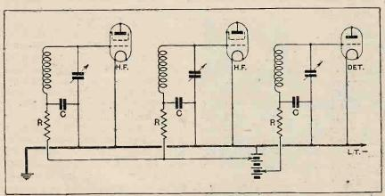
Fig. 1.—Grid bias system for 2 H.F. stages followed by an anode bend detector. The condenser rotors may be earthed, and the first by-pass condenser (C) may be the coupling condenser of a filter. Decoupling resistances are marked R.
