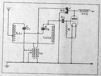
Fig. 1.—Simplified diagram of the tuning circuits and detector. References correspond with those of the complete diagram.
