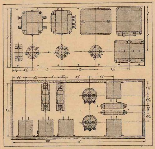
Fig. 4.—Layouts of the upper- and under-side of the baseboard.
