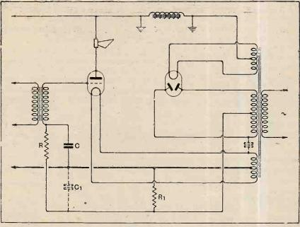
Fig. 2.—How A.C. voltages may be transferred to an output valve grid circuit through capacity leakages between power transformer windings.
