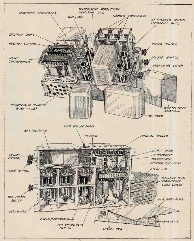
Chassis details of the Gecophone All-electric Four-valve Receiver.
