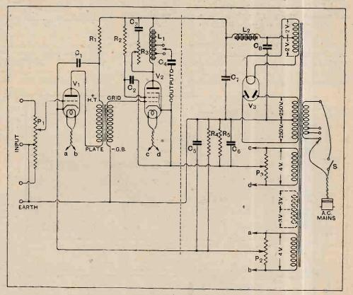
Fig. 1.—The theoretical circuit diagram. Values are as follows:  $P_1$ , 1 megohm;  $P_2$  and  $P_3$ , 50 ohms;  $R_1$ , 20,000 ohms;  $R_2$ , 10,000 ohms;  $R_3$ , 25,000 ohms;  $R_4$ , 750 ohms;  $R_5$ , 250 ohms;  $C_1$ ,  $C_2$ ,  $C_4$ ,  $C_5$ , and  $C_6$ , 2 mfds.;  $C_3$ , 0.01 mfd.;  $C_7$ , and  $C_8$ , 4 mfds.
