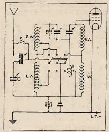
Fig. 2.—A band-pass filter with variable inductive coupling; the differential aerial input control may be short-circuited by the switch S. C. aerial capacity balancing condenser; L, coupling inductance; S.W., short-wave coils; L.W., long-wave coils.
