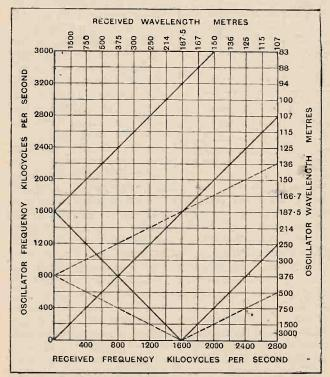
Fig. 3.—Relationship between received and oscillator frequencies for a superheterodyne of "Infradyne" type, using an intermediate frequency of 1,600 k.c.
