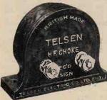
TELSEN H.F. CHOKES. Designed to cover the whole wave-band range from 18 to 4,000 metres, extremely low self-capacity, shrouded in gennine Bakelite. Inductance 150,000 micro-henries. Resistance 400 ohms. Price 2/6 each.
