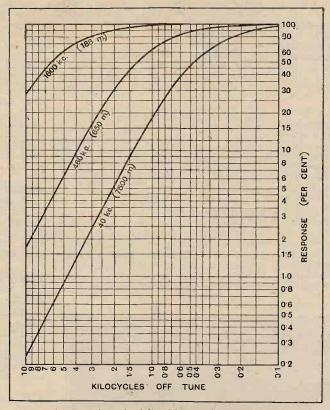
Fig. 5.—Comparative selectivity of intermediate amplifiers working at different frequencies. The very high selectivity associated with the superheterodyne method of reception is due entirely to the use of a very long wave for intermediate amplification.
