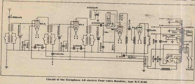
in its filament-heating circuit. Pre-H.F. volume control is provided by a series aerial condenser which serves also as a control of selectivity. In preparing the set for test one finds that the transformer is not only tapped to suit 200-, 220- and 240-volt supplies, but, in addition, there are three more terminals marked 10, 5 and -5 volts. By this means all mains potentials from 195 to 250 can be accommodated to the nearest 5 volts.
