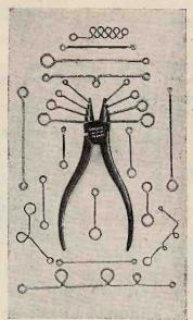
Entirely British in design and manufacture, they are invaluable to everyone associated with the Wireless, Electrical, and kindred trades. Made of the best tool steel, hardened and tempered in oil. Eight gauges on one tool, ensuring neat and accurate loops in one operation, in a fraction of a minute. Wire cropper incorporated in circular joint.
