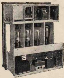
The Westinghouse Metal Rectifier is shown in the lower left-hand corner of this interior view of the set.
