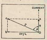
Fig. 2.—Voltage vectors for an inductive coil when the current is 1 ampere.
