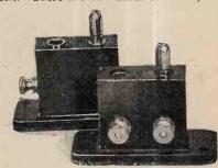
Two types of bakelite coil mounts made by Franklin and Freeman, Ltd.
