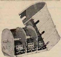
Polar "Tub" three-gang screened condenser with disc drive.
