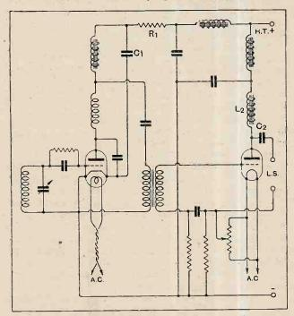
Fig. 2.—The complete choke transformer coupled circuit with a single output valve. As explained in the text, this circuit is not entirely satisfactory. With a 200 volts H.T. supply,  $R_1$  must be 8,600 ohms, and  $C_1$  about 8 mfd., while the choke  $L_2$  must have an inductance of 50 henrys when  $C_2$  is 4 mfd.
