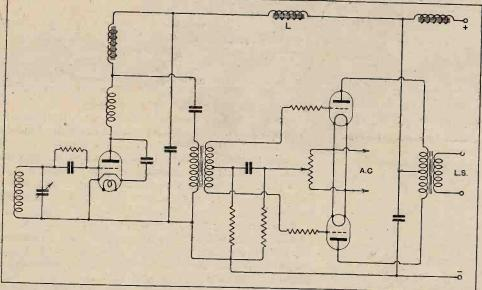
Fig. 3.—An economical and satisfactory choke-transformer coupled circuit. The H.T. supply needs no decoupling, and a proportional smoothing circuit can be used.
