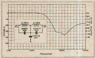
Filter with modified values of inductance giving a filter peaking at about 10,000 cycles.
