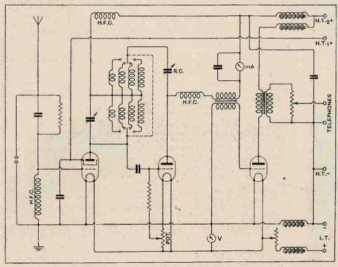
Complete circuit diagram. Valves are Marconi S.215, H.L.210, and L.210.
