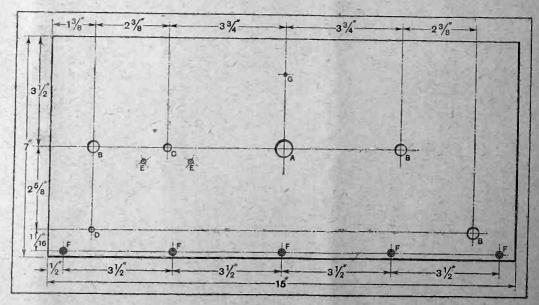
Fig. 5.—Drilling details of the front panel, which is of plywood, 1/4ln. thick. A, 9/16ln. dia. B, 3/8ln. dia.; C, 1/4ln. dia.; D, 3/16ln. dia.; E, 5/32ln. dia.; F, 1/8ln. dia., countersunk; G, 3/32ln. dia.
