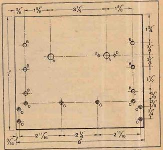
Fig. 3.—The panel layout. Drilling details are as follows: A, §in. dia.; B, 7/32in. dla.; C, §in. dia., countersunk for No. 4 wood screws; D, §in. dia.
