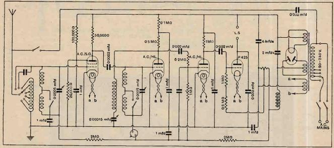
Circuit of the Wates All-Electric Four, compiled from details furnished by the manufacturers (The Standard Battery Company).
