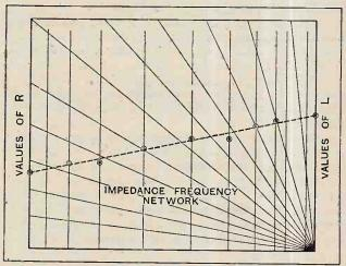
Fig. 5.—Schematic diagram showing method of deriving values of L and R from experimentally related values of z and f. The network of impedance and frequency lines shown here and in Fig. 6 is not accurately drawn, and the lines are not, therefore, numbered. The correct positions of the network lines are given in Fig. 8.
