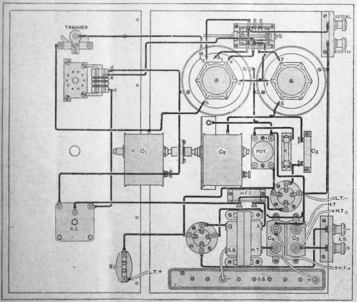
Fig. 7.—Practical wiring plan. Connection is made between the coupling control switch spindle and the point marked d. Note that the coll screen bases and the condenser shield are earthed.
