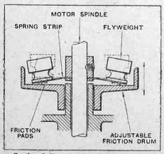
Sectional diagram showing principle of the Diebl governor mechanism.
