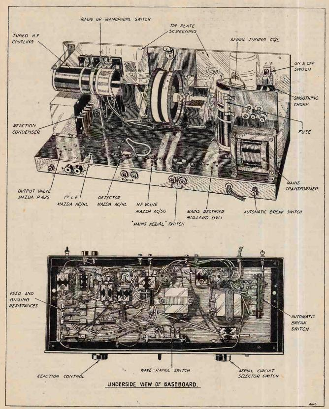
WATES ALL-ELECTRIC FOUR.—Back and underside views of the chassis.
