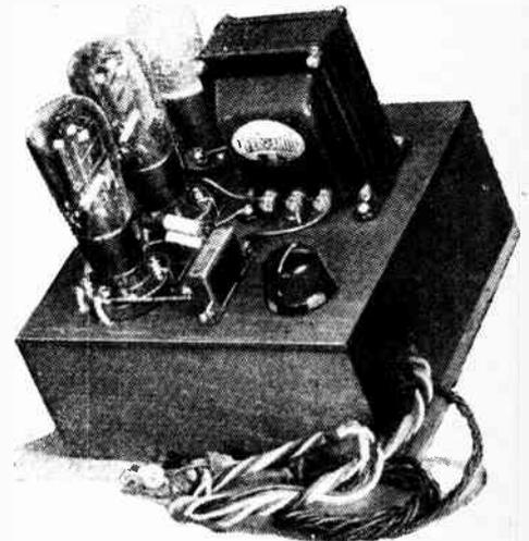
Three-quarter plan view of battery model. In the lower right-hand corner is the control knob of the grid bias potentiometer.
