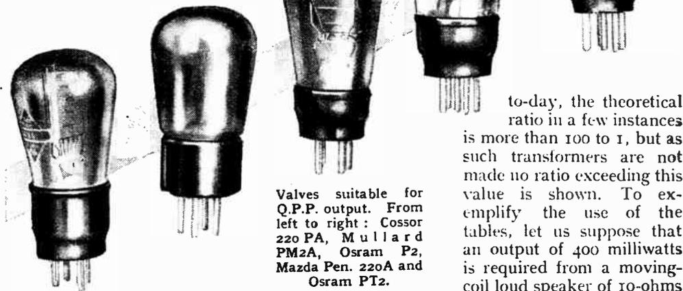
Valves suitable for Q.P.P. output. From left to right: Cossor 220 PA, Mullard PM2A, Osram P2, Mazda Pen. 220A and Osram PT2.
