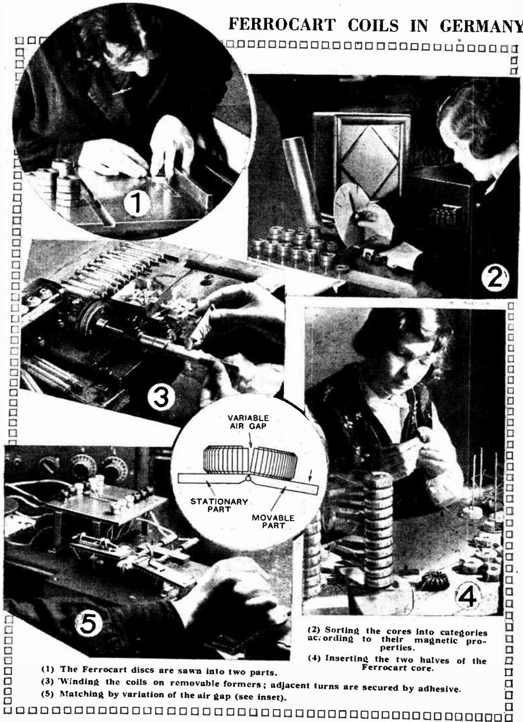
(1) The Ferrocart discs are sawn into two parts.
