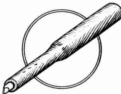
A simple form of insulated screwdriver, for adjusting trimming condensers. It is supplied with certain H.M.V. radio-gramophones.
