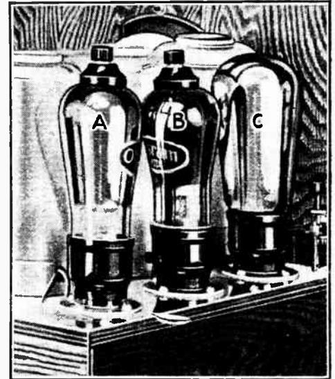
The first detector (B) is here shown mounted between the H.F. valve (A) and the oscillator (C).
