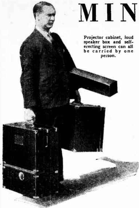
Projector cabinet, loud speaker box and self-erecting screen can all be carried by one person.
