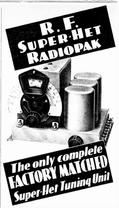
THE unit comprises CONSTANT, AERIAL COUP-LING coil, R.F. inter-valve coil and oscillator coil, special super-het aganged condenserthe oscillator tuning section having "shaped" tracking vanes ensuring matching over the whole wave-band. The R.F. Super Radiopak is matched within ½ of 1 per cent. before despatch. One has only to balance out the stray circuit capacities with the aid of the trimmers conveniently provided at the top of the Unit to ensure permanent MATCHED PERFECTION.
