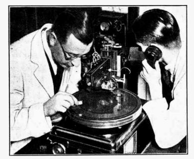
RECORDING THE KING'S MESSAGE. By special permission of His Majesty, an H.M.V. record was made of the broadcast message on Christmas Day. The engineers are shown superintending the recording on the wax blank, one checking the volume while his companion examines the sound track through a magnifying glass.
