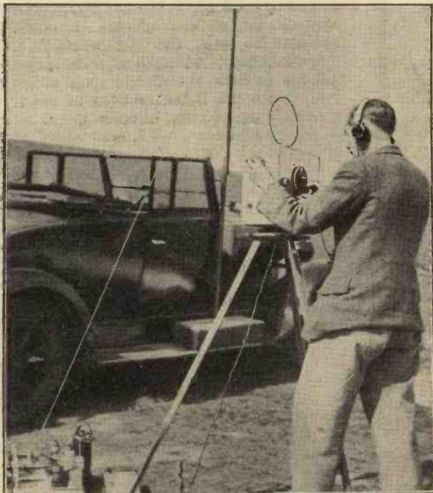
Initial tuning adjustments being made within sight of the transmitter. A superheterodyne for open aerial use is seen on the ground.
