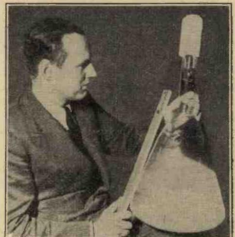
Fig. 5.—Von Ardenne with one of his high-power cathode-ray tubes.
