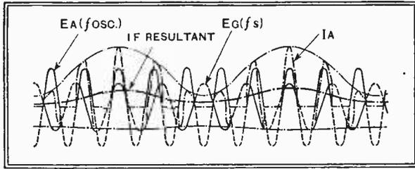
Fig. 5.—Showing additive mixing in "Ultra-dyne" circuit.
