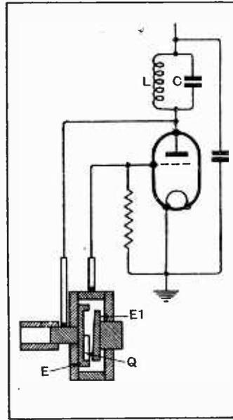
Method of mounting a piezo-electric crystal to "wobble" the frequency of a master oscillator stage.
