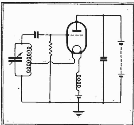
Fig. 8.—Earthing the anode end of the tuned circuit.
