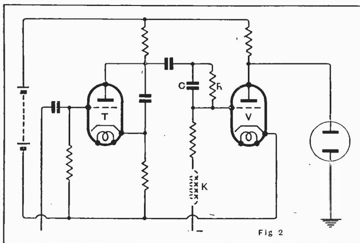
Fig. 2.—Frequency compensated amplifier for television scanning circuit.
