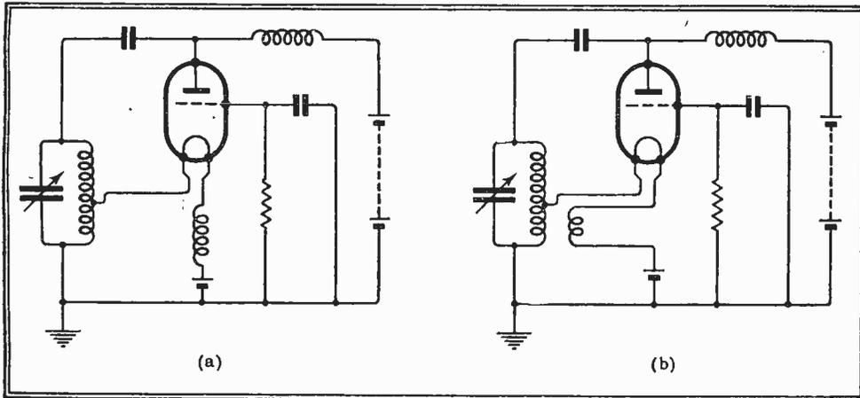
Fig. 7.—Arrangements permitting the grid end of the tuned circuit to be earthed. The filament-circuit coil in diagram (b) must be closely wound with the tuned winding.
