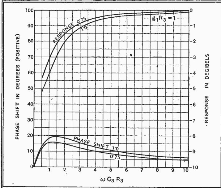
Fig. 30.—These curves show the effect of the bias resistance  $R_3$  and its by-pass condenser  $C_3$ .
