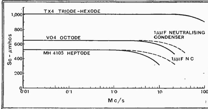
be substantially reduced. If the  $I_a/EG_4$  curve is a perfect exponential curve (so-called anti-cross curve) this trouble can be even further reduced. With the progress of valve-making technique generally, even the relative inefficiency of the early multiplicative mixers could have been overcome, and it really appeared that one or
