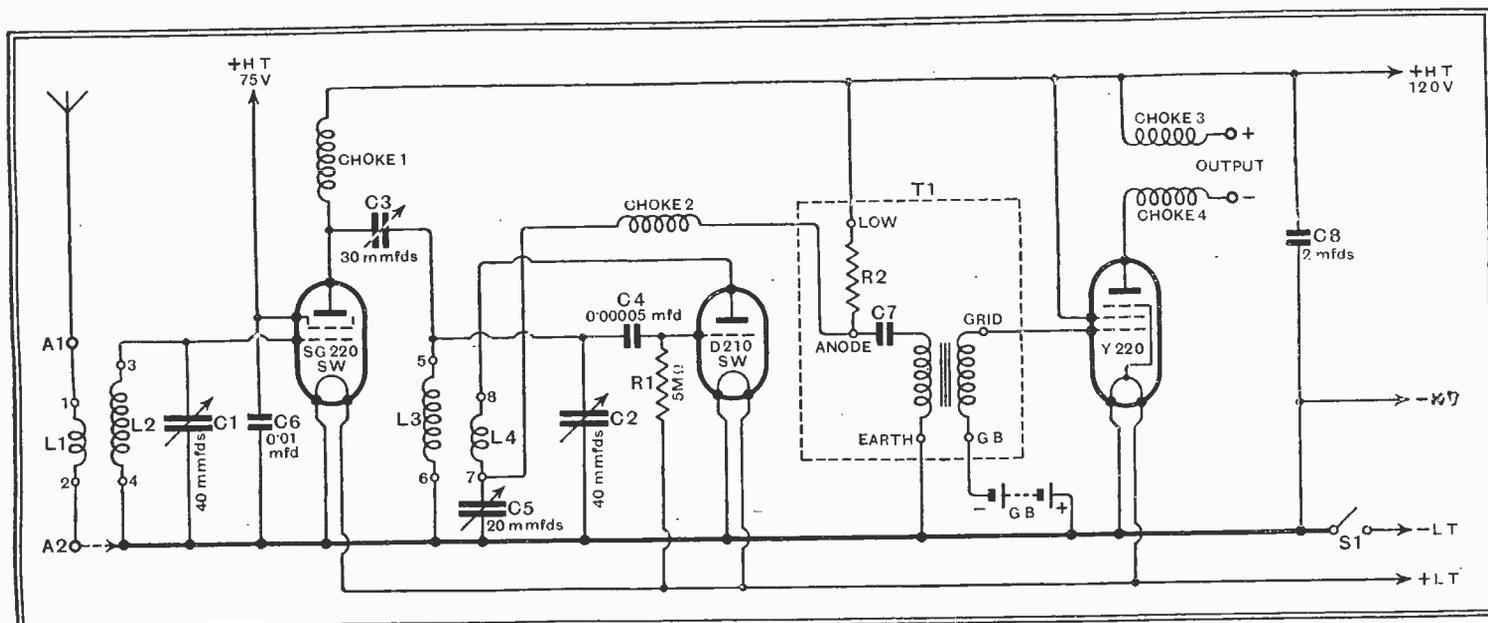
Fig. 1.—Theoretical circuit diagram of the ultra-short wave receiver.
