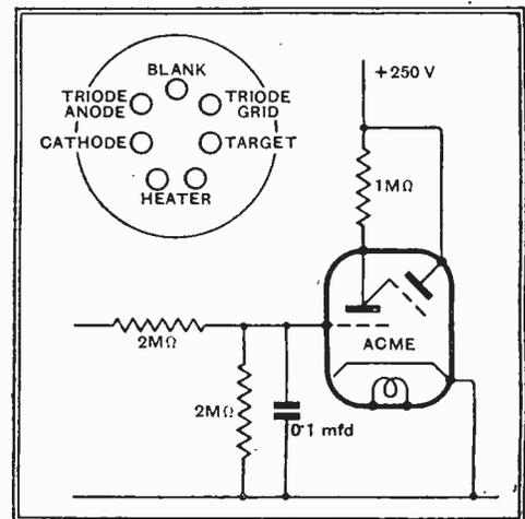
Base connections and circuit for using the ACME indicator.
