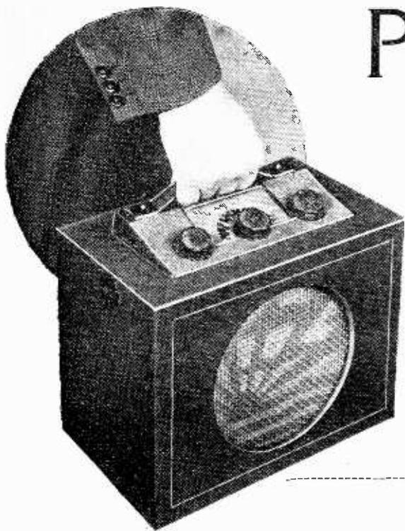
**FEATURES.** *Type.*—Portable battery receiver. *Circuit.*—Pentode RF amplifier—triode grid detector—triode first AF amplifier—pentode output valve. *Controls.*—(1) Tuning. (2) Combined volume and reaction. (3) Waverange and on-off switch. *Price.*—8 gns. *Makers.*—Pye Radio Ltd., Radio Works, Cambridge.
