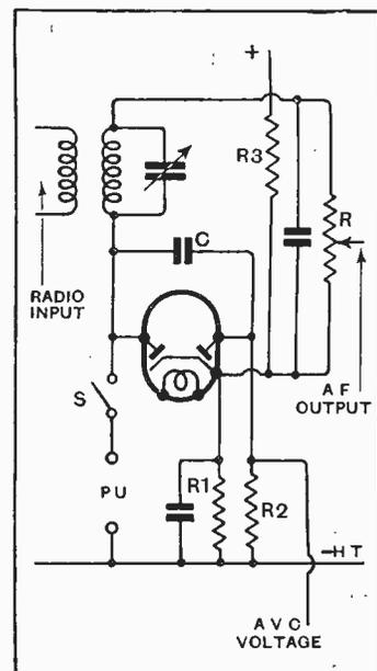
Circuit arrangement when a volume control common to radio and gramophone is used.
