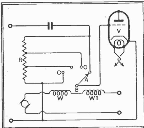
Volume according to the speed: novel application of AVC to a car radio receiver.
