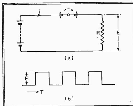
Fig. 1.—Artificially generated interference: operation of the rotary switch in diagram (a) produces a square-topped wave form represented by curve (b).
