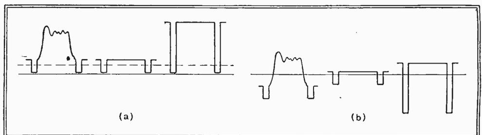
Fig. 23.—Three typical signals are shown at (a), the first corresponding to a normal line, the second to a black line, and the third to a white line. The same signals are shown at (b) with the DC component removed.
