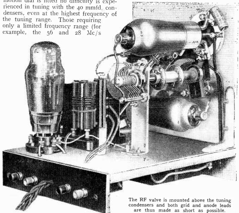
The RF valve is mounted above the tuning condensers and both grid and anode leads are thus made as short as possible.
