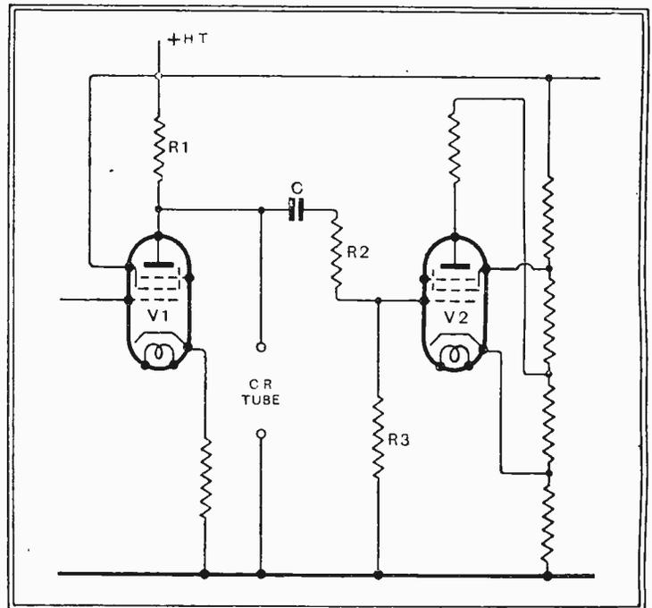
Fig. 22.—This circuit is the same as that of Fig. 21 save for the insertion of the condenser C. This removes the trouble of inconsistent operation, but proper synchronisation cannot be obtained because the condenser removes the DC component of the signal.
