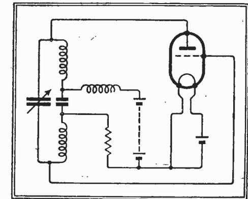
Fig. 10.—The Franklin circuit has a close family resemblance to the Hartley.
