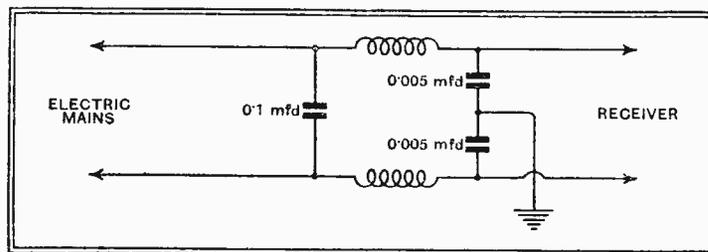
Fig. 6.—A choke-condenser filter applicable to general use.
