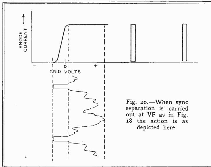
Fig. 20.—When sync separation is carried out at VF as in Fig. 18 the action is as depicted here.
