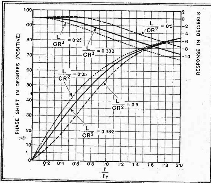
gible effect and the coupling consists essentially of  $L$ ,  $R_1$  and  $C_1$ , this last consisting of the total of the strap capacities. This form of coupling was discussed in some detail in Part IV with particular reference to its use as an IF amplifier, and it was shown that the best compromise be-
