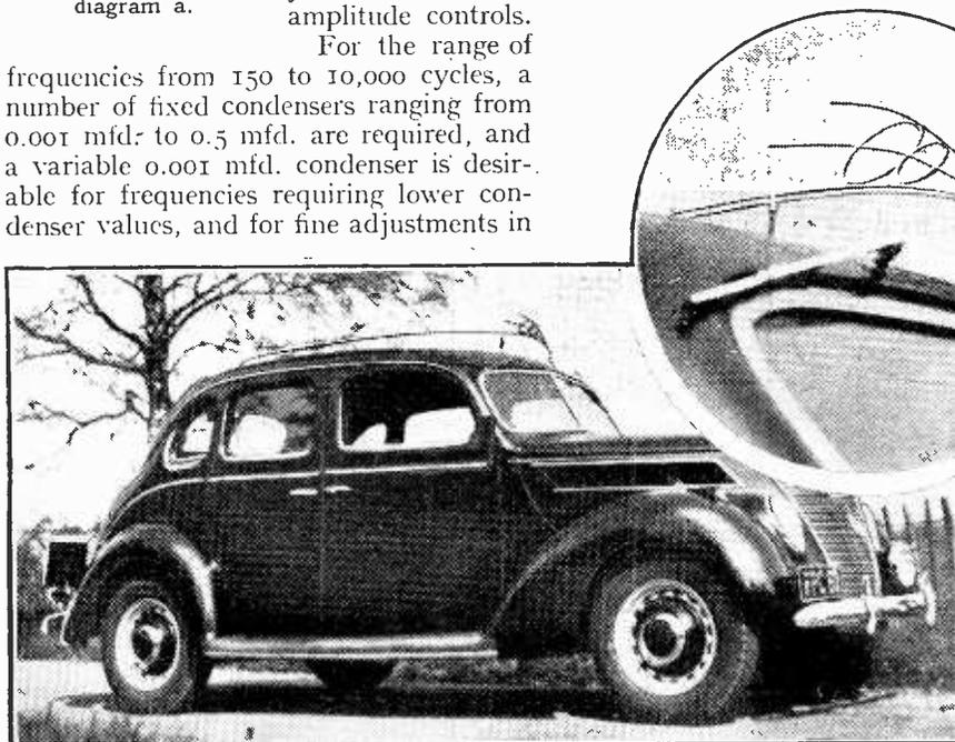
**SYMBOLICAL AERIAL.**—A Ford car fitted with an aerial taking the form of the familiar "V8" device. The external aerial, more effective and conducive to a better signal-to-noise ratio than the concealed type, is gradually coming into use on cars fitted with broadcast receivers.
