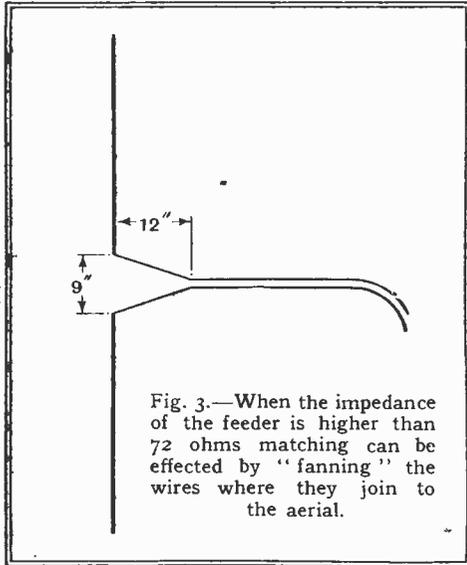
Fig. 3.—When the impedance of the feeder is higher than 72 ohms matching can be effected by "fanning" the wires where they join to the aerial.
