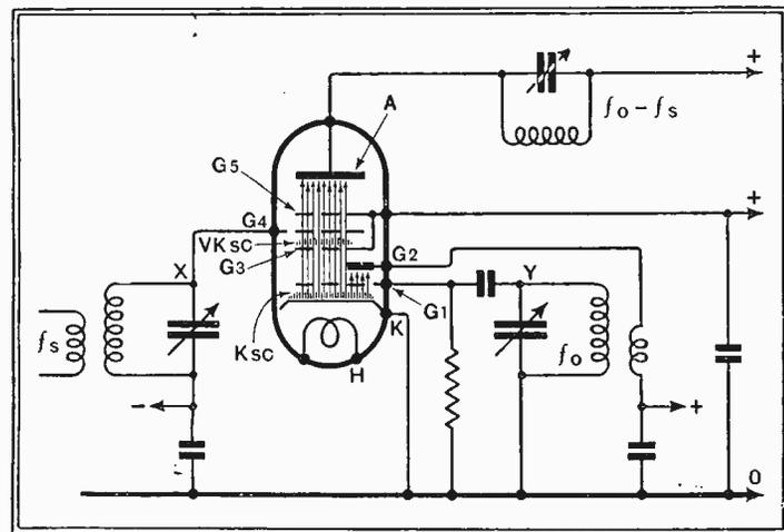
ing to illustrate the instantaneous density of electrons. The accompanying table gives an explanation of the function of the electrodes as well as their potentials relative to cathode. The characteristic in Fig. 15 shows the quantity of electrons in the virtual cathode space charge as a function of the voltage on the first grid.
