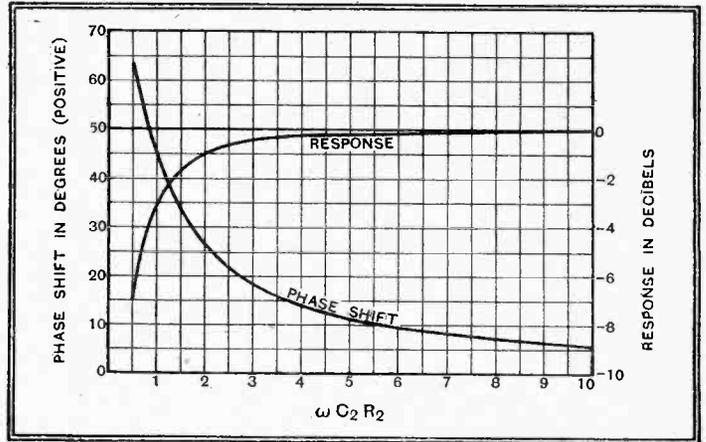
Fig. 29.—The response and phase shift at low frequencies caused by the coupling condenser  $C_2$  and grid leak  $R_2$  are shown here.
