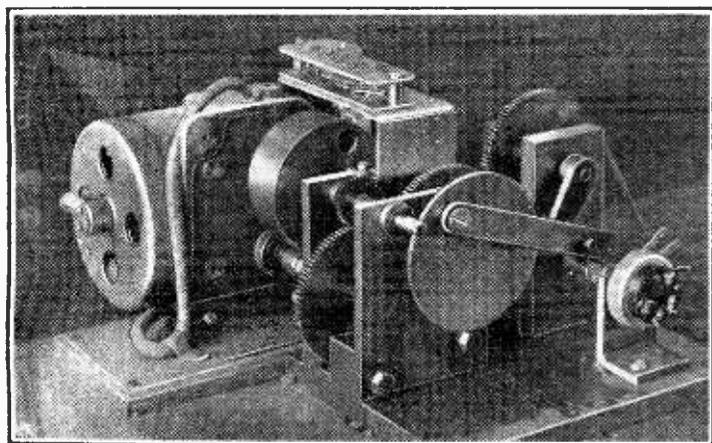
Life tests of volume controls and on-off switches are carried out with this reciprocating mechanism. The machine runs day and night and a counter at the top records the number of movements made.
