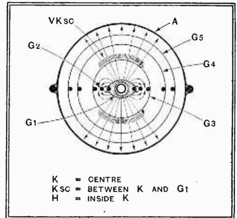
Fig. 14.—Representation of a section through a heptode.
