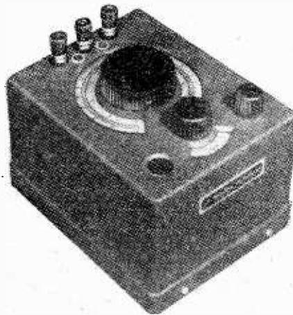
AC mains operated resistance, capacity and general-purpose measuring bridge.
