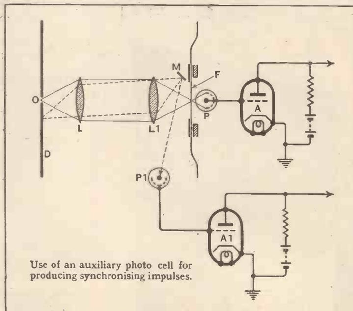
Use of an auxiliary photo cell for producing synchronising impulses.
