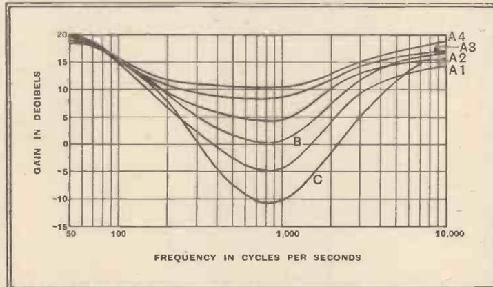
Fig. 4.—The response curves obtained are shown here. A1 to A4 are for  $C_1 = 0.0003 \mu\text{F}$ ,  $C_2 = 0.015 \mu\text{F}$  and  $R_1 = 75,000$  ohms with different settings of the cathode potentiometer. Curves B and C are respectively with  $R_1 = 0$  and  $C_2 = 0.01 \mu\text{F}$ .
