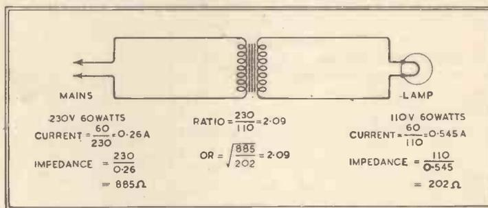
Fig. 1.—Illustrating the functioning of a power transformer working under constant operating conditions.
