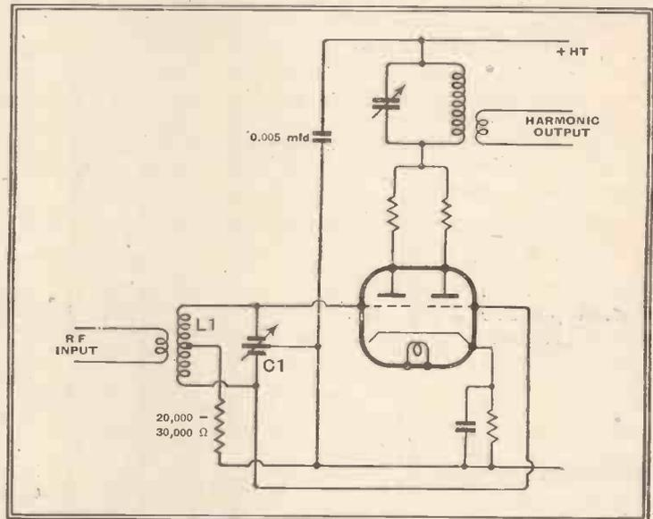
Fig. 2.—A push-pull doubler suitable for frequencies up to 28 Mc/s.
