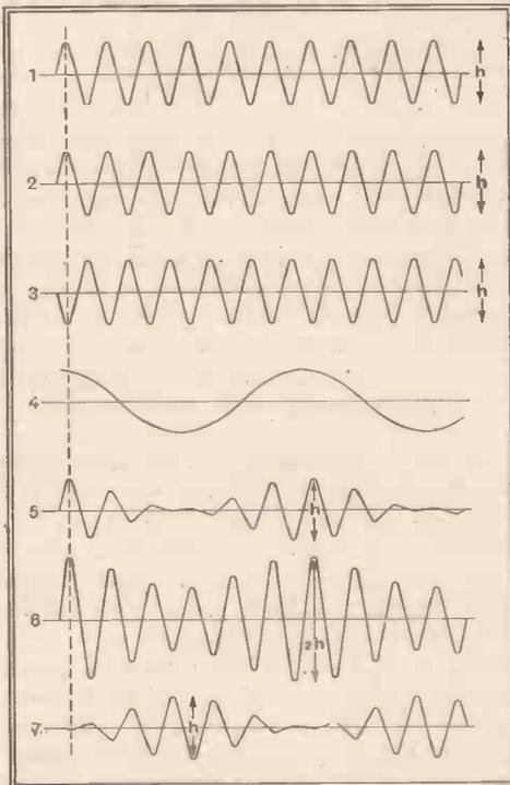
Fig. 4.—Effect of high-speed switch on received signals.
