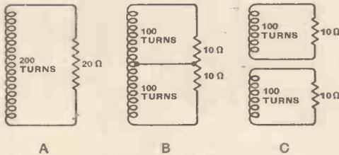
rectly designed to supply a load of 20 ohms as shown, and for the sake of argument let the number of turns be 200. Then according to the well-known rule that the ratio of turns is proportional to the square root of the ratio of impedances, it looks as if a 100-turn winding ought to be correct for supplying a quarter of the load resistance—5 ohms.
