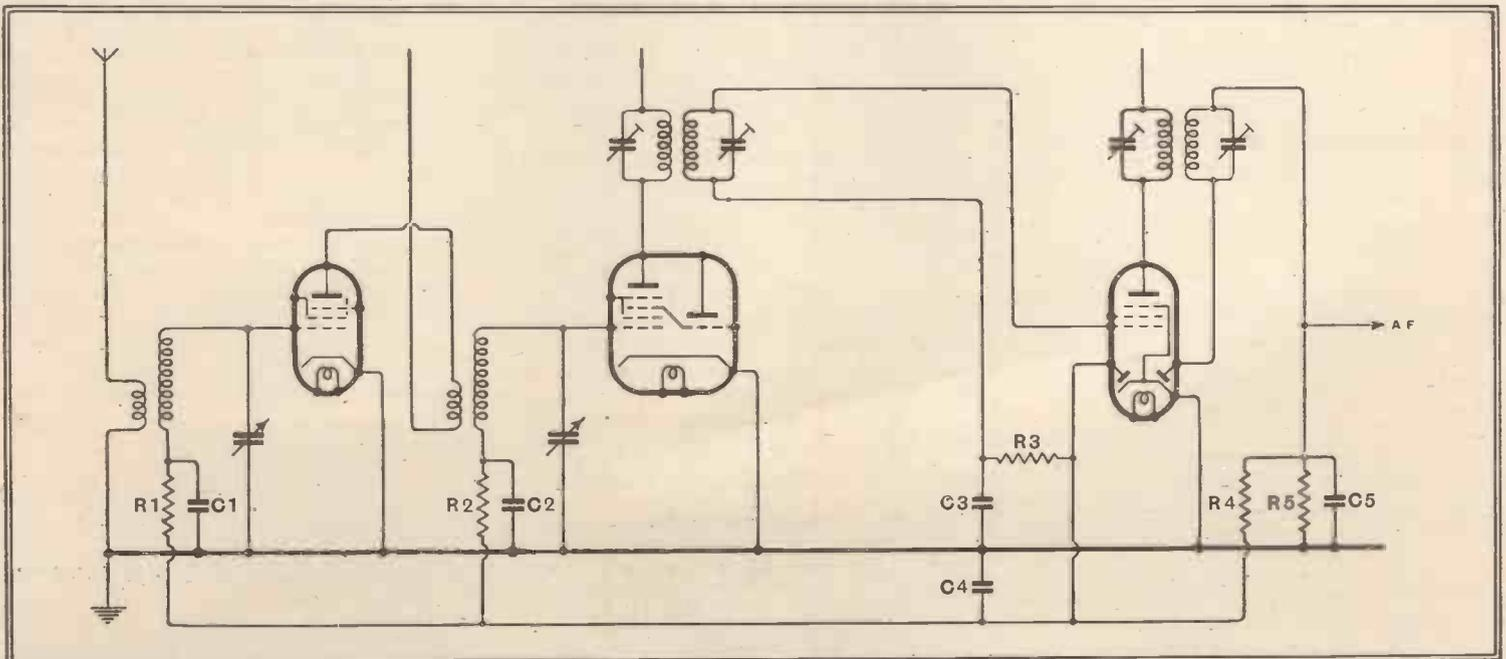
Fig. 1.—This diagram shows the simple arrangement which can be used with the valves. Initial grid bias is not essential.
