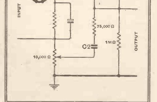
Fig. 3.—The new tone-control circuit; the response is varied by the cathode potentiometer.
