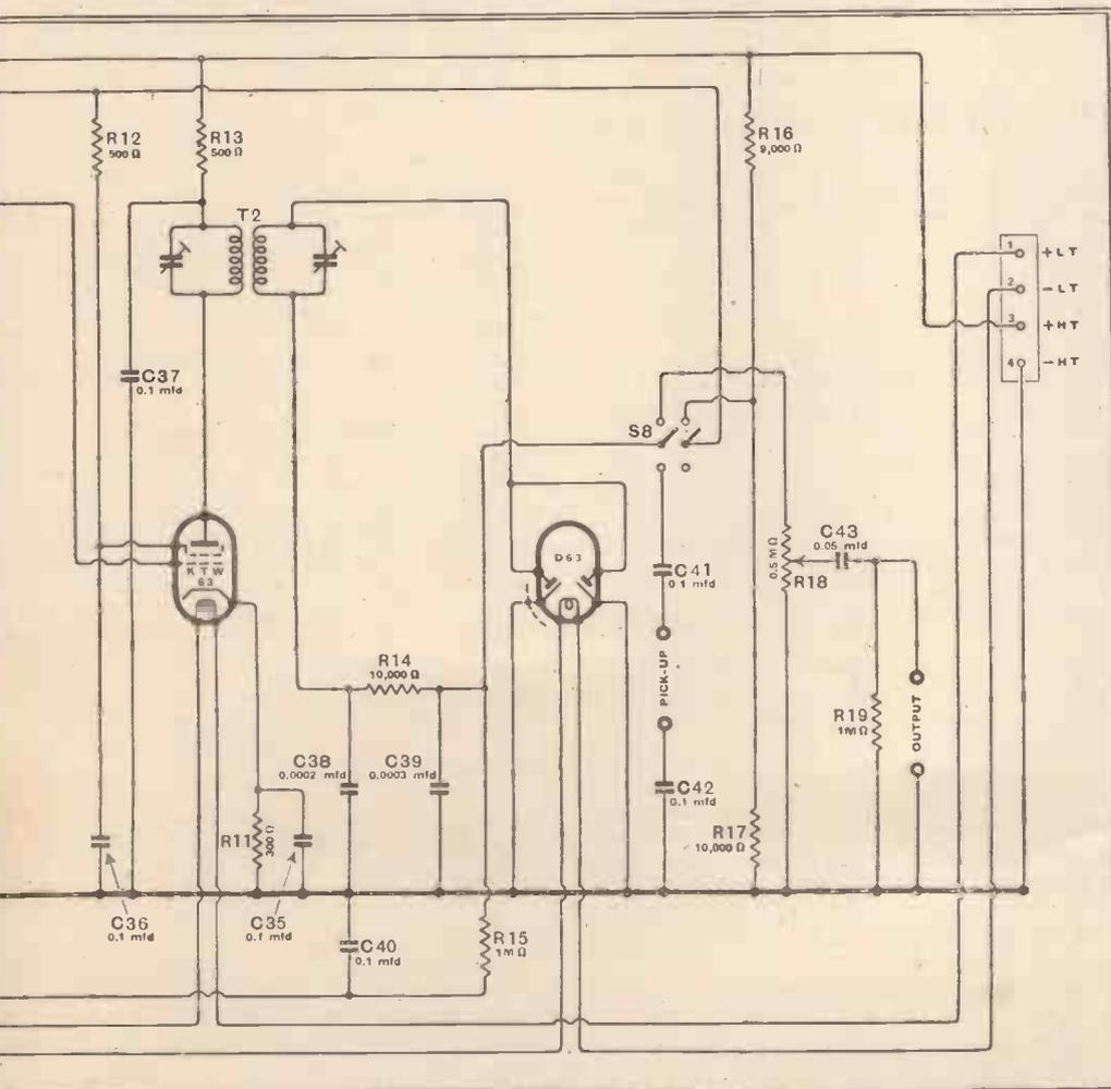
Fig. 1. This diagram shows the complete circuit of the receiver portion. Isolating condensers C1, C2, C41 and C42 are connected in the aerial, earth and pick-up leads.
