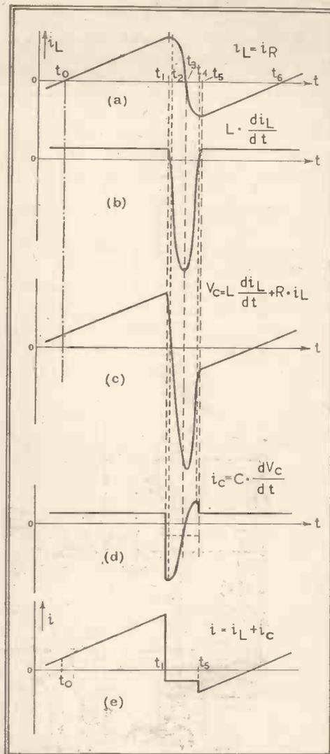
Fig. 2.—The method of determining the relation between the coil and input currents is shown here. (a) represents the desired coil current, (b) the voltage across the coil, and (c) the voltage across the condenser; (d) shows the condenser current and (e) the line current.
