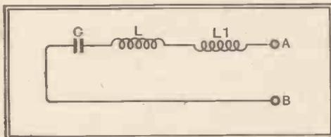
Fig. 4.—Equivalent circuit of a fixed condenser (neglecting resistance).
