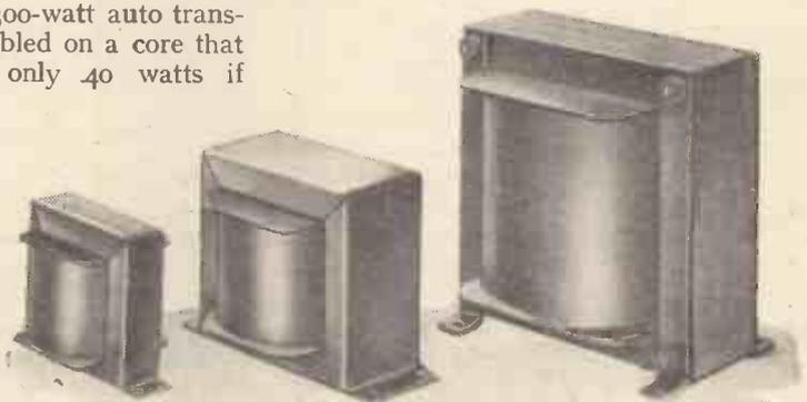
Fig. 6.—All these transformers handle the same wattage but the smallest and medium-size models are auto-wound. The largest weighs 29½ lb., the medium-size one 12 lb. and the smallest 3½ lb.
