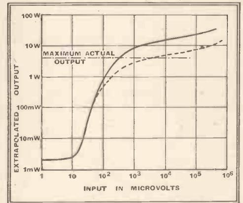
Fig. 2.—AVC characteristic, again taken at 1,000 kc/s, obtained by the ascending signal strength method. Valuable information on the design is revealed, including the desirability of reducing the delay voltage to alter the characteristic to the position shown by the dotted line.
