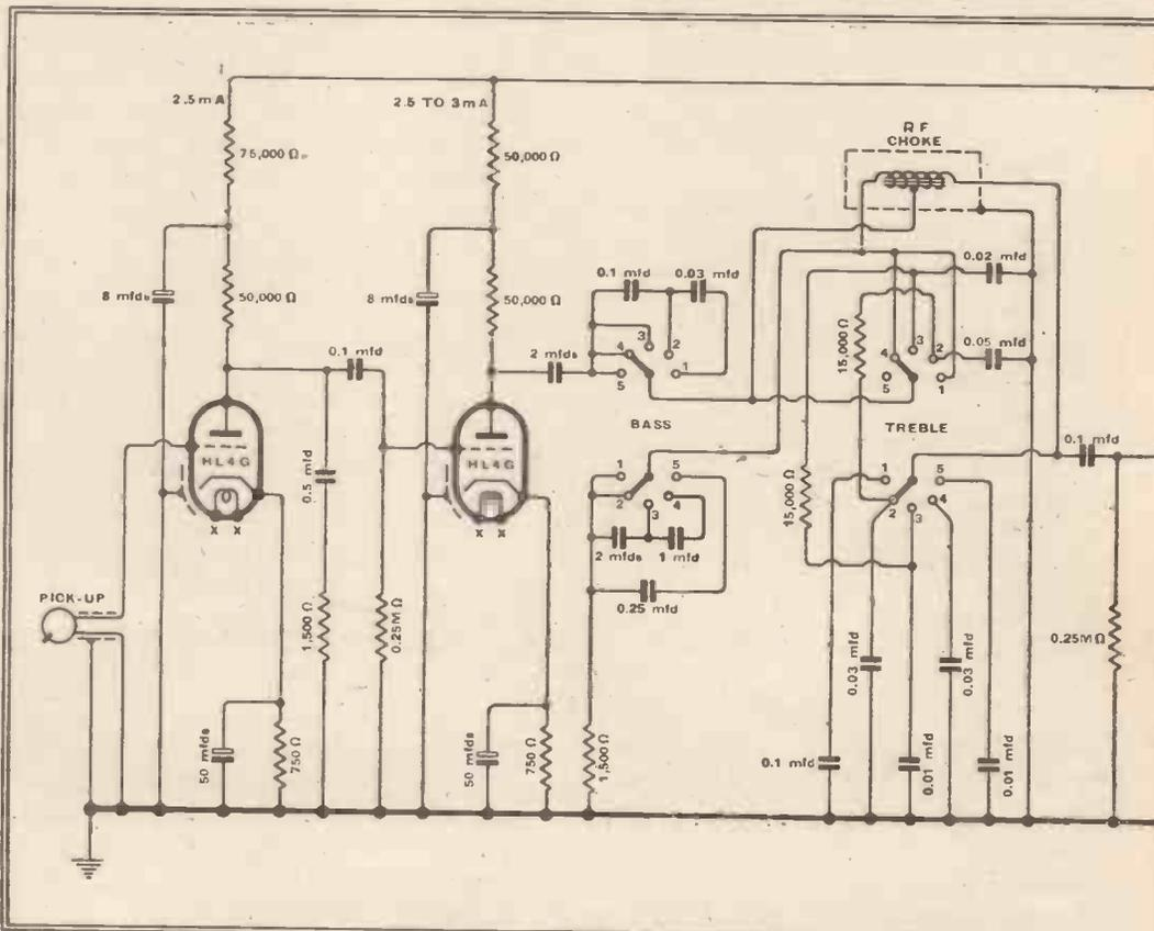
Fig. 1.—Complete circuit diagram of amplifier and tone control.
