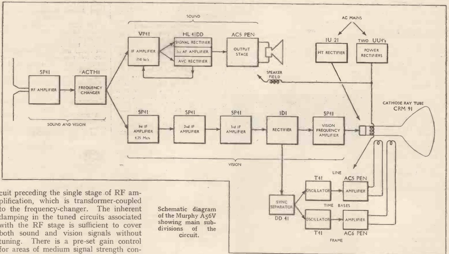
Schematic diagram of the Murphy A56V showing main subdivisions of the circuit.
