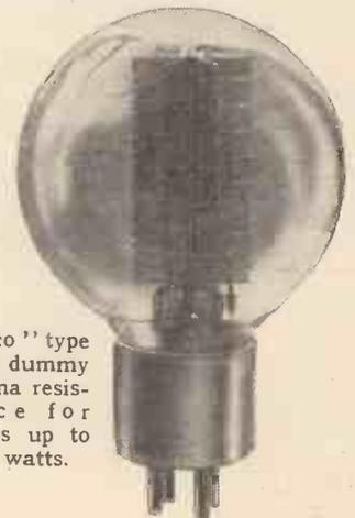
"Omco" type D.100 dummy antenna resistance for powers up to 100 watts.
