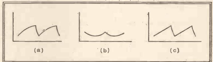
Fig. 4.—The usual exponential waveform (a) is obtained across C2 of Fig. 3 and the semi-circular wave (b) across C3. The output wave (c) is linear and is the sum of (a) and (b).
