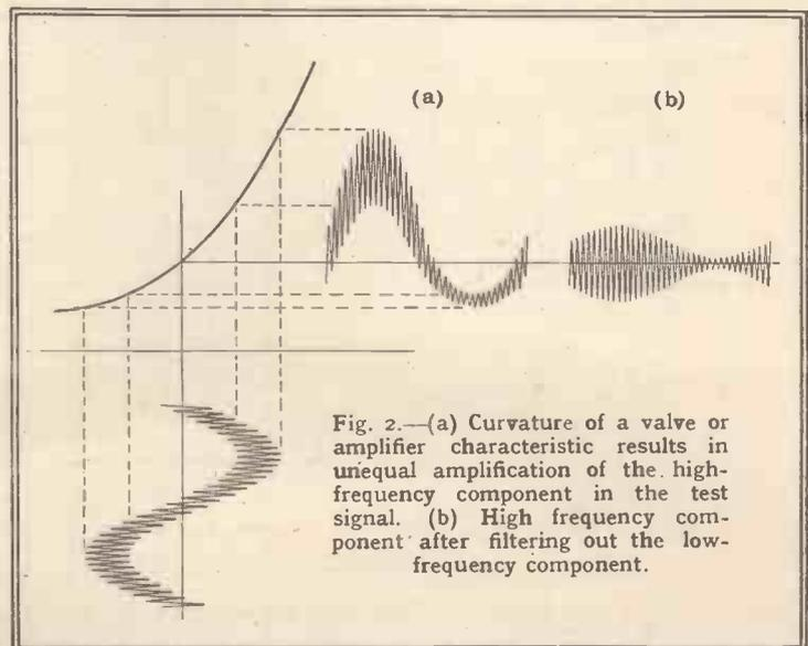
Fig. 2.—(a) Curvature of a valve or amplifier characteristic results in unequal amplification of the high-frequency component in the test signal. (b) High frequency component after filtering out the low-frequency component.
