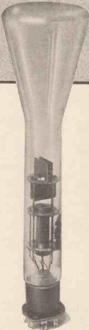
**T**HE 4096 A Cathode Ray Tube is a hard vacuum tube suitable for use with anode voltages from 800 to 2,000 volts and has a screen diameter of 3 inches. The screen provides a blue spot of high actinic value necessary for photographic purposes and, in addition, owing to its intense brilliance, is suitable for visual work.
