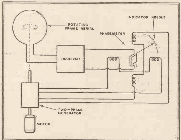
Fig. 1.—Simplified diagram of a single-frame radio compass.
