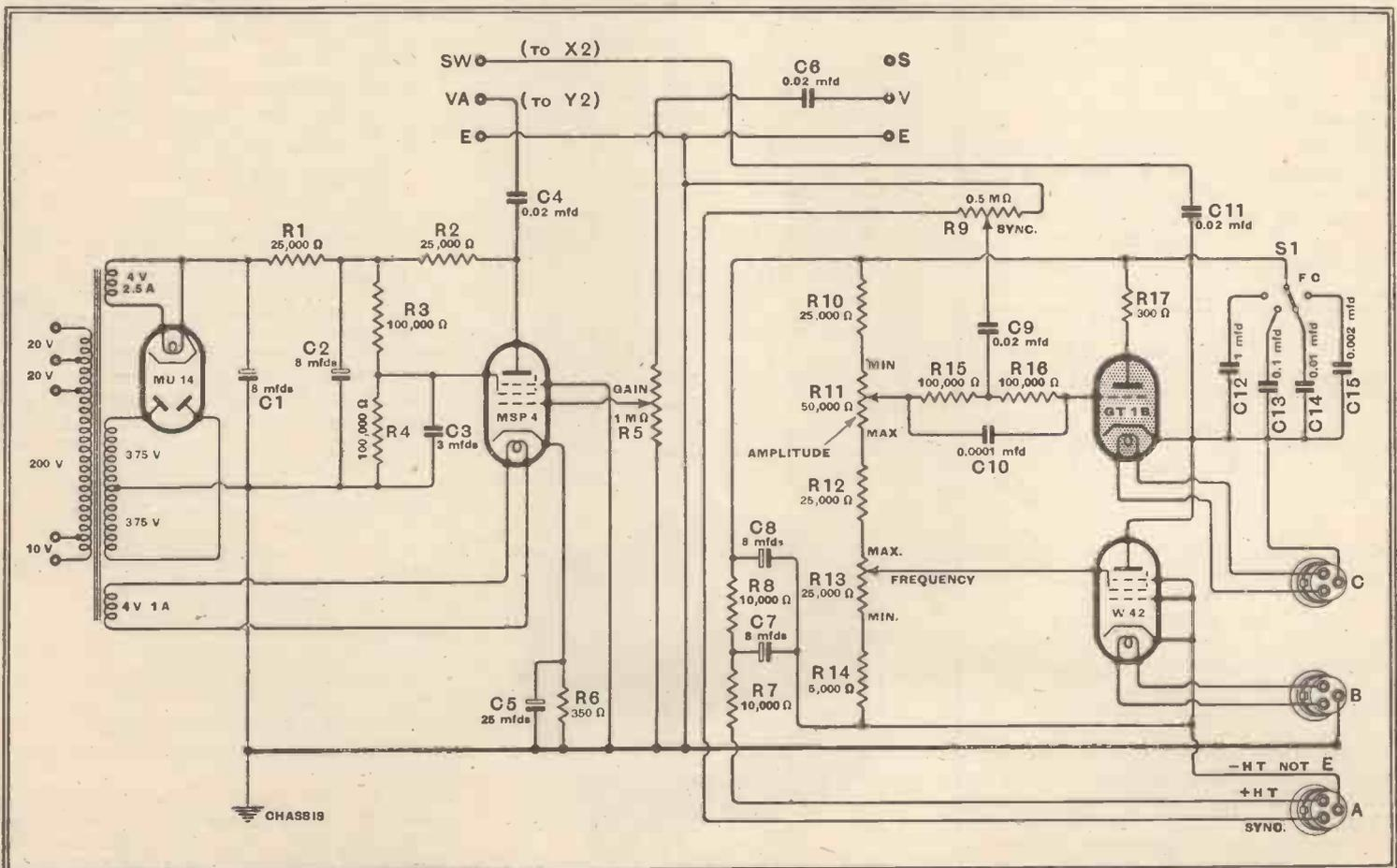
Fig. 3.—Circuit diagram of the time-base unit incorporating an amplifier for the observation of waveform.
