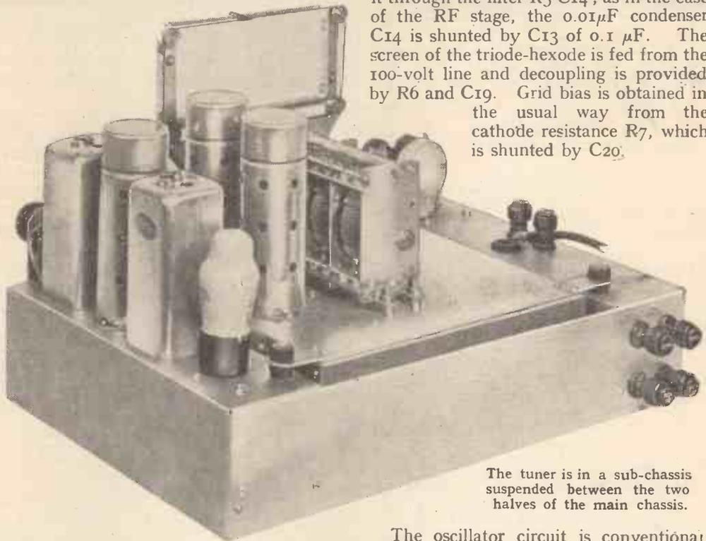
The tuner is in a sub-chassis suspended between the two halves of the main chassis.
