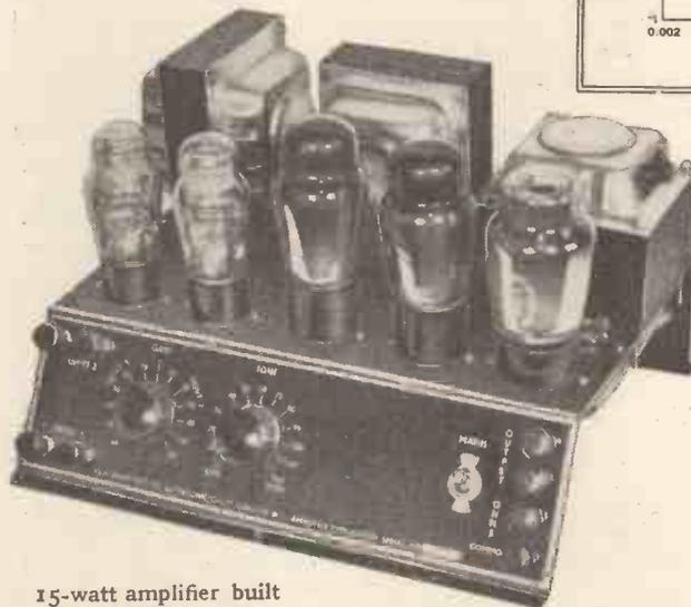
15-watt amplifier built from a kit of parts.
