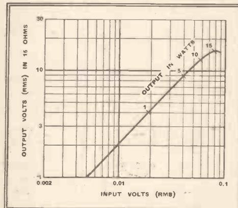
Input-output curve of the Film Industries amplifier at 400 c/s. Output resistance 16 ohms.
