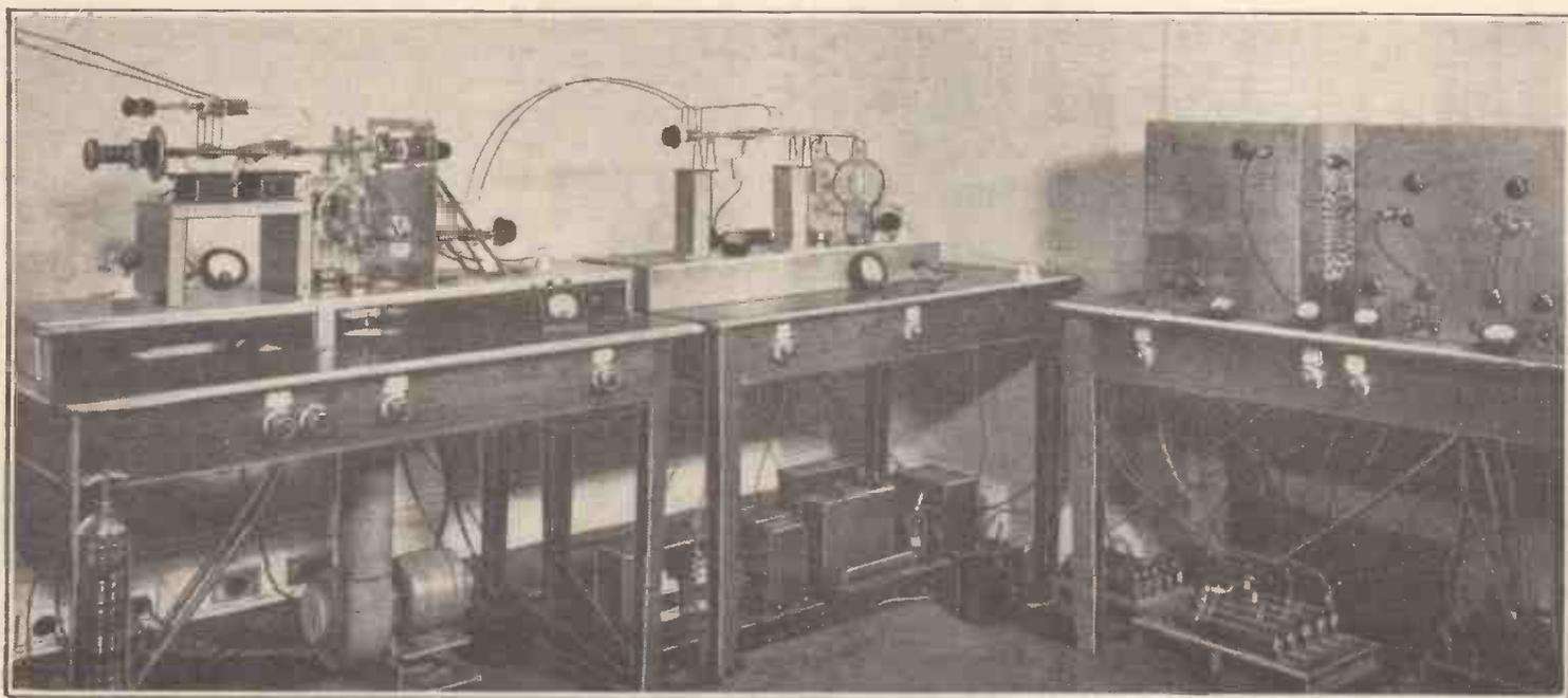
The power amplifying stages of the Yonkers station. On the right are the earlier amplifying stages, in the centre the push-pull driver and, on the extreme left, the push-pull output stage, which delivers 600 watts at 110Mc/s. The output valves are air-cooled by a blower under the bench.
