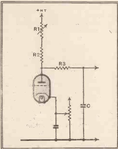
Fig. 1.—The conventional gas-triode saw-tooth oscillator.
