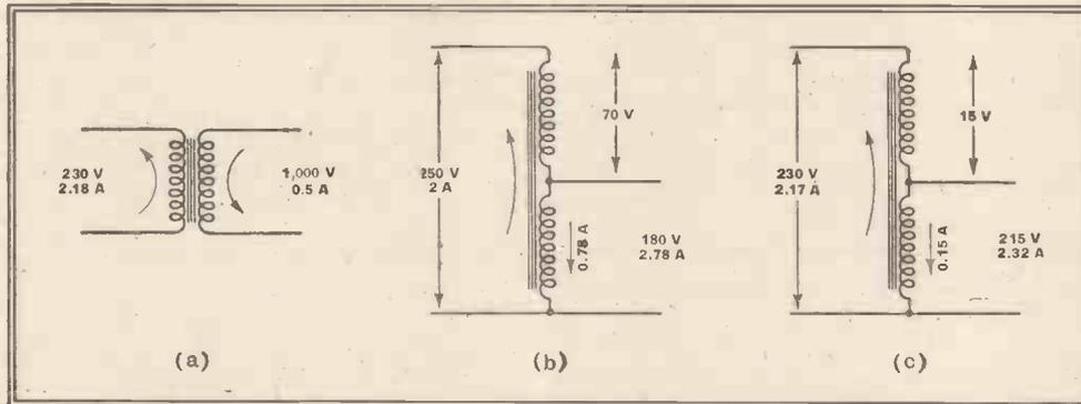
Fig. 7.—Voltages and currents of the three transformers illustrated in Fig. 6 (a) the large model, (b) the medium-size one and (c) the smallest.
