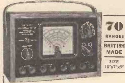
**MODEL 80A.** This precision built Universal Meter with its sturdy 4 1/2" Moving Coil movement covers D.C. volts 0.002-2,000; A.C. Output volts 0.2-2,000; D.C. Current 10.A-20 Amps; A.C. Current 10.A-5 Amps. Resistance 0.1 Ohms-5 megohms. Output -18 to +60 DB. at the touch of two switches. Although unusually low in price the TAYLOR METER is extremely reliable, sensitive and accurate.
