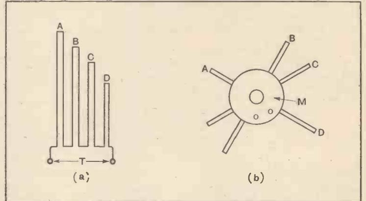
Use of quarter-wave coaxial or parallel conductors as rejectors for waveband filtering.
