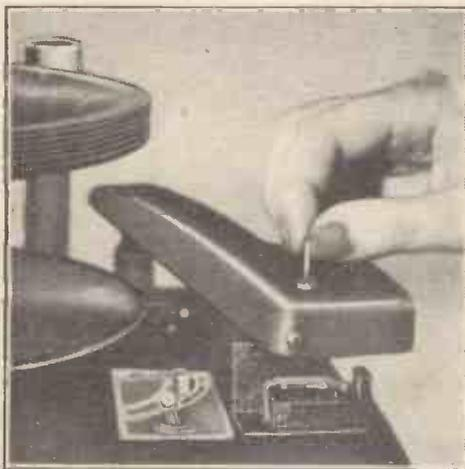
Needle loading from the top and automatic needle ejection are features of this RCA crystal pick-up. The needle is inserted in a hole at the top of the head and the point comes to rest against the bracket below, while the normal screw retainer is adjusted. To remove the needle, the screw is loosened and the pressing of a lever withdraws the retaining bracket to reveal a container into which the used needle drops.
