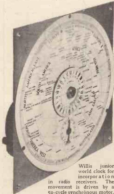
Willis junior world clock for incorporation in radio receivers. The movement is driven by a 50-cycle synchronous motor.
