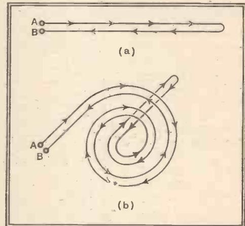
Fig. 2.—Diagram (a) shows a conductor bent back on itself; winding the same conductor into a helix, as in diagram (b), has a negligible effect in increasing inductance.
