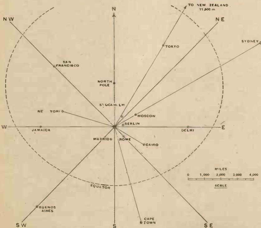
Fig. 1.—Diagram showing approximately the true direction and distance from London of some of the world's broadcasting centres.
