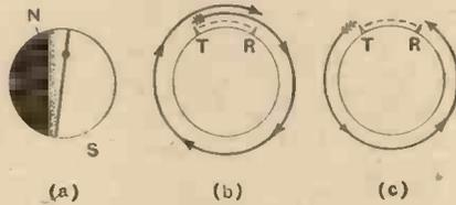
Fig. 2.—Explaining the production of round-the-world echo signals. (a) Lighting conditions on a winter morning, showing echo path. The lighter shaded part represents twilight zone. (b) A forward round-the-world echo path and (c) a backward echo path. Actually the signals would not have a circular path as shown, but would travel round the world in several reflections between layer and earth. Dotted line represents direct signal between transmitter and receiver.
