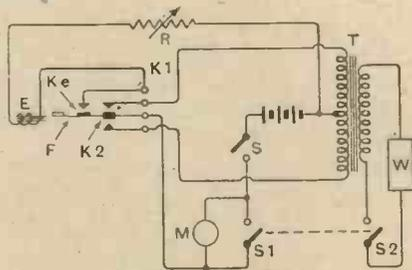
By means of the rheostat R, energising current is increased to compensate for wear of the vibrator contacts
