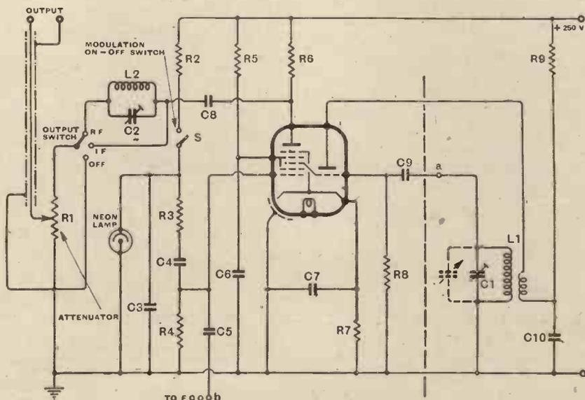
Fig. 3.—The mixer circuit shown in this diagram is suitable for a portable unit. Component values are: R1, 100Ω var.; R2, 2 MΩ; R3, 2 MΩ; R4, 25,000Ω; R5, R6, 10,000Ω; R7, 300Ω; R8, 30,000Ω; R9, 25,000Ω; C3, C4, 0.001μF; C5, 50μμF; C6, C7, 0.1μF; C8, 0.01μF; C9, 0.001μF; C10, 0.1μF. Valve: Mazda TH41.
