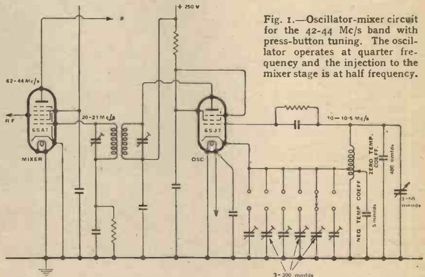
Fig. 1.—Oscillator-mixer circuit for the 42-44 Mc/s band with press-button tuning. The oscillator operates at quarter frequency and the injection to the mixer stage is at half frequency.
