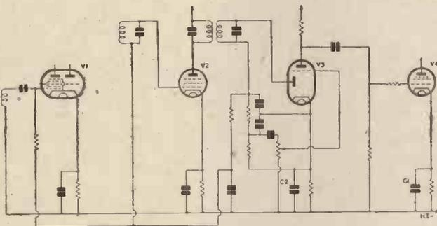
FIG. 1. *The Typical Cathode Bias System*
