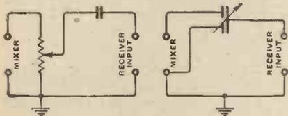
Fig. 2.—Two simple forms of attenuator which can be used to control the amount of test signal injected into the receiver.
