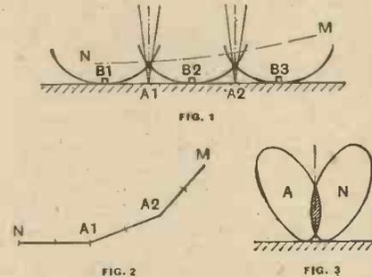
Radio marker system for aircraft
