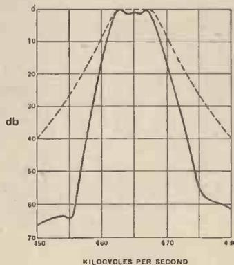
Fig. 8.—Modification of the circuit of Fig. 7 with (full line) response characteristic compared with two ordinary transformer-coupled IF stages (dotted line).
