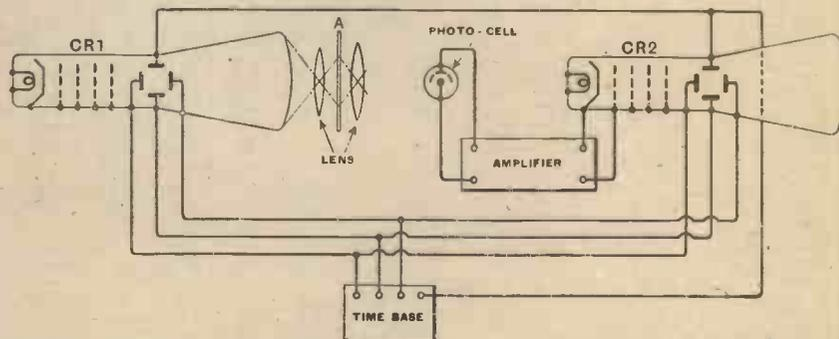
The diagram shows the connections adopted for CR1 and CR2 to create a positive image of a photographic negative.
