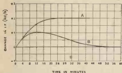
Fig. 2.—Frequency drift of the circuit shown in Fig. 1. Curve A uncompensated, curve B compensated by negative temperature coefficient condenser. The positive change in IF is due to the oscillator being on the low frequency side of the signal.
