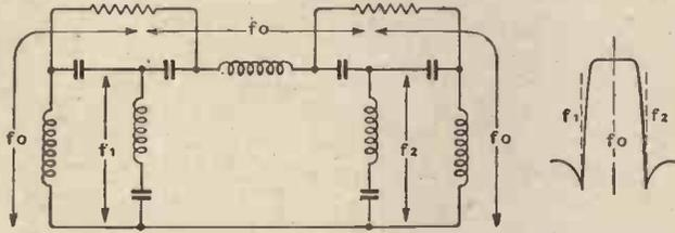
Fig. 7.—Band-pass circuit including rejection circuits designed to improve selectivity outside the pass-band. The side dips are usually located 9 kc/s from the mid-frequency.
