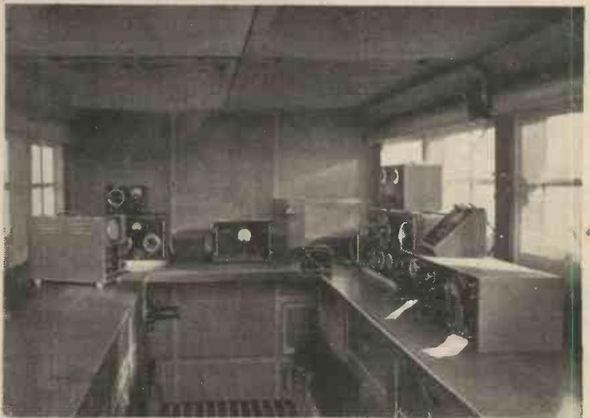
A mobile test room mounted on a six-wheel lorry chassis. Some of the test apparatus with which it is equipped can be seen on the benches. Lockers and drawers under the benches contain other apparatus, tools and spare parts.
