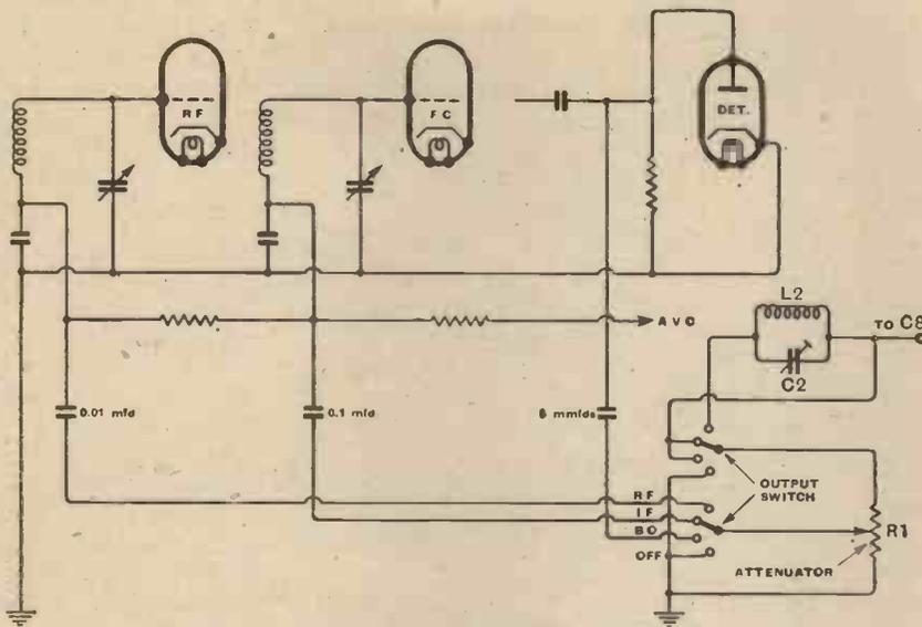
Fig. 4.—If the mixer is incorporated in a receiver, it can be arranged to act as a BO in addition to providing test signals. This diagram shows how the output circuit of Fig. 3 can be modified, and suggests a method of injecting the test signals into the receiver.
