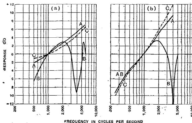
are plotted in Fig. 8 (a). The hypothetical case of  $CD=0$  is plotted in Fig. 8 (b). It will be clear that frequency distortion is only severe if  $(N-M)\lambda$  is large, or  $CD$  small. The former condition will be quite normal on SW, but it is not simulated
