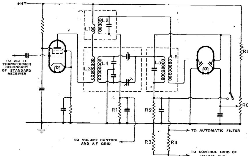
Fig. 1. Carrier boosting circuit. Values of components: L1, small 8-turn coupling coil; L2, 90  $\mu$ H, shunted by 1350  $\mu\mu$ F; L3, L4, L5, L6, 860  $\mu$ H; R1, 0.2 megohm; R2, 0.5 megohm; R3, R4, 2 megohms; R5, 50,000 ohms; R6, 10,000 ohms.
