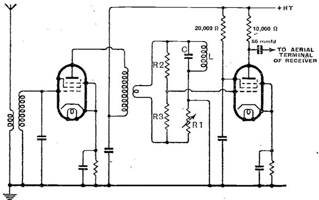
Fig. 5. Circuit for producing artificial selective fading.
