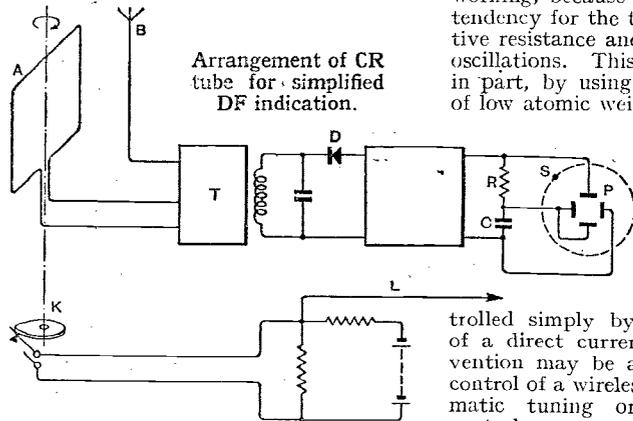
The output from the latter is then rectified at D and applied, through a phase-splitting circuit R, C, to the deflecting plates of a cathode-ray tube P. In the ordinary way, this would cause the electron beam to trace out the circular path shown in dotted lines on the fluorescent screen, the trace being continuously visible.
