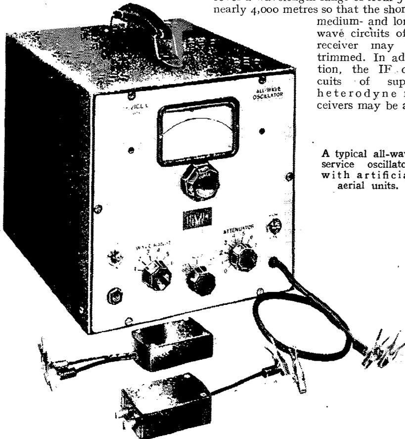
A typical all-wave service oscillator, with artificial aerial units.
