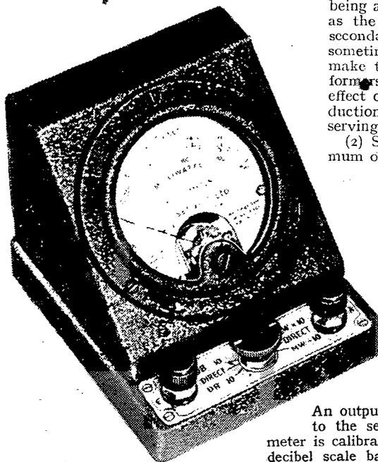
An output meter, a companion instrument to the service oscillator. This particular meter is calibrated in milliwatts and also has a decibel scale based on a zero value of 50 mW.
