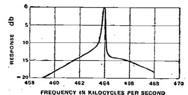
Fig. 2. Carrier attenuation: measured response obtained with circuit of Fig. 1.
