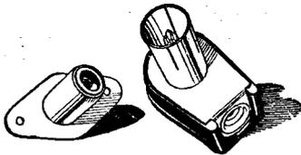
**COAXIAL PLUG and SOCKET** the first mass-produced type for coaxial leads. Supplied to grip air-spaced or solid di-electric cables. For mounting on chassis or cover of conduit box. All metal parts silver plated, moulded bakelite cover. Socket in each case is complete with plug.
