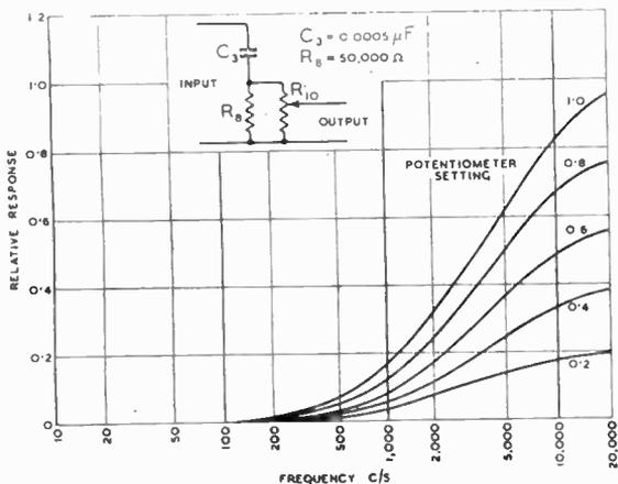
Fig. 10. Modified treble tone control filter showing the effect of varying the setting of the potentiometer  $R_{10}$ .
