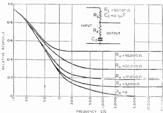
Fig. 2. Basic bass tone control filter showing the effect of varying the resistance  $R_4$ .
