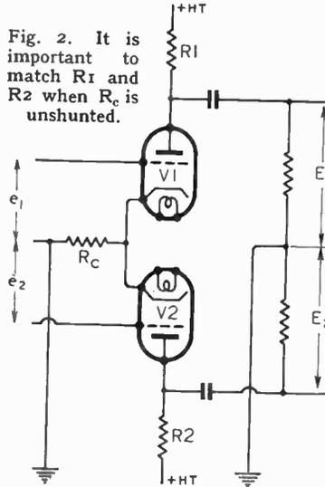
Fig. 2. It is important to match  $R_1$  and  $R_2$  when  $R_c$  is unshunted.
