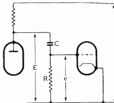
Fig. 1. Essential elements of a resistance-capacity coupling.
