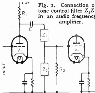
Fig. 1. Connection of tone control filter  $Z_1, Z_2$  in an audio frequency amplifier.
