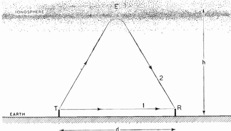
Fig. 7. Principle of technique used in determining height of reflecting regions in the ionosphere. Two sets of waves, 1 and 2, reach the receiver R from the transmitter T, along TR and TER respectively. From the difference in time of arrival, the path difference of these sets of waves, and so the height of the region E, can be determined.
