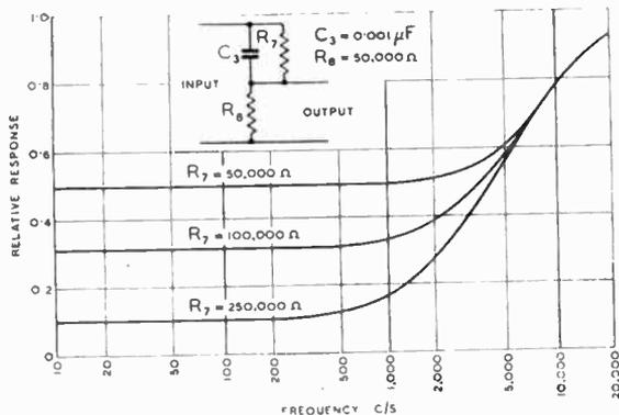
Fig. 7. Basic treble tone control filter showing the effect of varying the resistance  $R_7$ .
