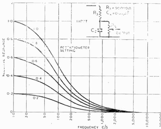
Fig. 5. Modified tone control filter, showing the effect of varying the setting of the potentiometer  $R_4$ .
