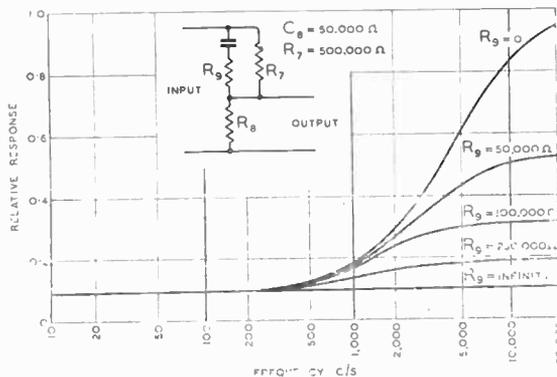
Fig. 9. Effect of varying the resistance  $R_9$  on the treble tone control filter.
