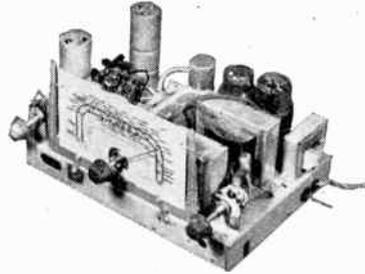
Aluminium screened coils, excellent short wave reception (the special coils used in this circuit give a performance equal to a superhet), 44 watts output, complete with loudspeaker, all parts, wiring and theoretical diagram—nothing extra to purchase. Chassis dim.: 12" x 8" x 6" to top of dial. 200/250 v. A.C.
