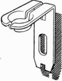
An enlarged view of the "Berricon" Beryllium Copper Socket, which maintains low and non-varying contact resistance for indefinite periods.
