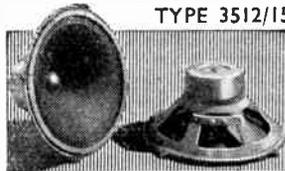
Overall diam. 12 $\frac{1}{2}$ ". Depth 6". Weight 7lb. 15 ozs. Voice Coil Impedance 15 ohms. Fundamental resonance 60 cycles. Flux density 14,000 lines per. sq. cm. Frequency range 50-7,000 c.p.s. Fixing holes 4 holes  $\frac{1}{2}$ " diam. spaced 90° on P.C.D. 12 $\frac{1}{2}$ ".
