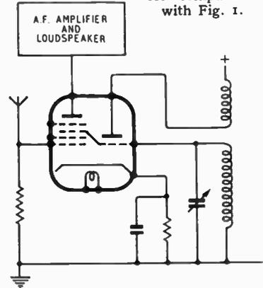
Suppose now we substitute a multiplicative detector for the additive one. Although a triode-hexode (Fig. 3) is not the best for the purpose, it is the most familiar, so will do very well for explanation. The important thing is that the hexode section should work on as nearly as possible a linear part of its control-grid characteristic, otherwise it would act more or less in the same
