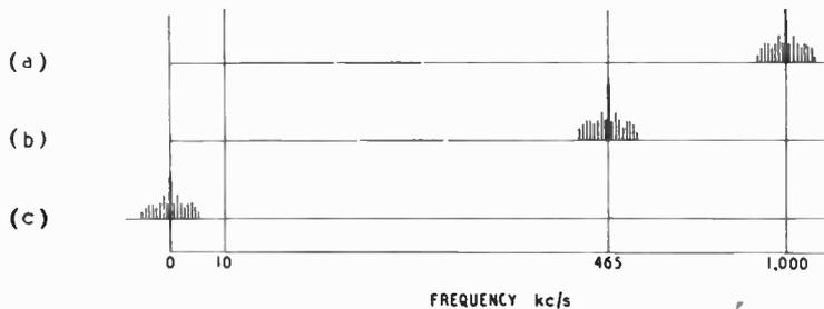
Fig. 4. Spectrum (a) represents a typical broadcast transmission as received, and as applied to the detector in a straight set; (b) the same after the frequency-changer in a superhet; and (c) after the modulator in a synchronyne.
