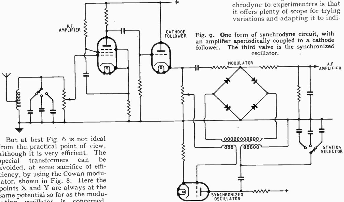
Fig. 9. One form of synchrodyne circuit, with an amplifier aperiodically coupled to a cathode follower. The third valve is the synchronized oscillator.
