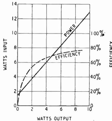
Fig. 7. Typical input-output characteristic of vibrator transformer.
