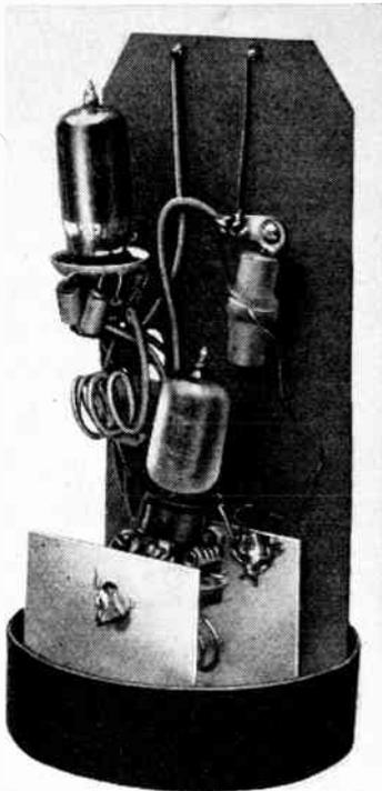
The inexpensive converter used for the American experiments in A.M. broadcasting to small communities on 87.75 Mc s.
