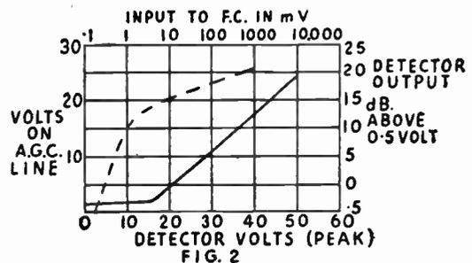
The graph of volts on AGC line against peak detector volts (in full line) in Fig. 2 shows that the change in AGC line voltage over the range 0 to 15 peak detector volts is only 0.5 volts over compared with 9 volts from 15 to 30 peak detector volts. The AGC characteristic for 30% modulation of a typical receiver using E/UAF42 is shown (in dotted line) in Fig. 2, the delay operates from 0.2 to 1mV and the AGC characteristic is flat to within 5db from 1 to 1000mV signal.
