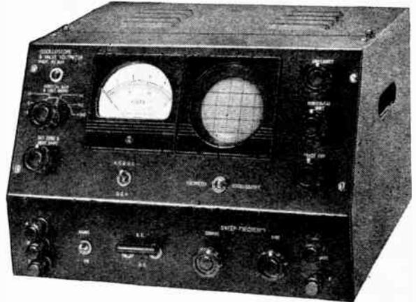
THE VOLTSCOPE—A combined valve-voltmeter and oscilloscope. VALVE-VOLTMETER—Infinite Input Resistance for D.C. ranges 0 to 300 volts. A.C. ranges 0 to 150 volts in 5 ranges. 3½ inch scale meter. OSCILLOSCOPE—3 inch screen tube provided with balanced amplifiers for Y and X plates giving a 5 times trace expansion. Maximum sensitivity 150mV/cm. Response from D.C. to 100 kcs.
