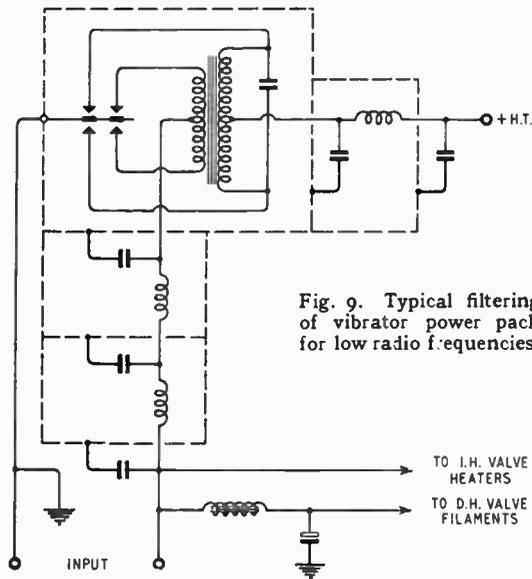
Fig. 9. Typical filtering of vibrator power pack for low radio frequencies.
