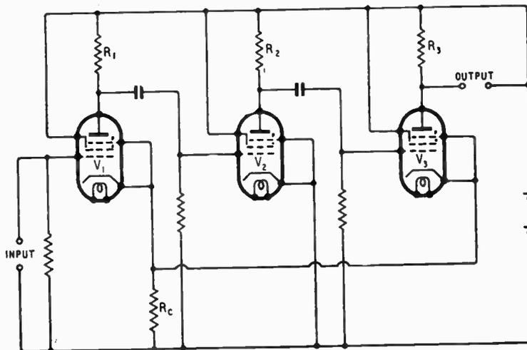
Fig. 1. Feedback circuit for wide-band amplifiers.
