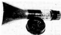
**CATHODE RAY TUBES—VCR97** (equals MULLARD ECR90) 6in. electrostatic tube, green screen, short persistence, high sensitivity. Recommended in last month's issue of "Wireless World," for use in the construction of an Oscilloscope. Each tube is brand new and individually packed in box for transit. Price 55/- only. With Holder.
