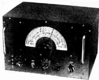
Labgear optional pre-selector or converter unit for A.C. operation.
