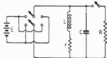
Fig. 2. Equivalent circuit of vibrator and transformer.
