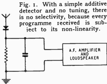
Fig. 1. With a simple additive detector and no tuning, there is no selectivity, because every programme received is subject to its non-linearity.
