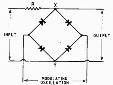
Fig. 8. An alternative synchrondyne modulator, more convenient but less efficient than Fig. 6.
