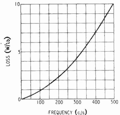
Fig. 8. Loss v. frequency for 0.014-in. transformer sheet.
