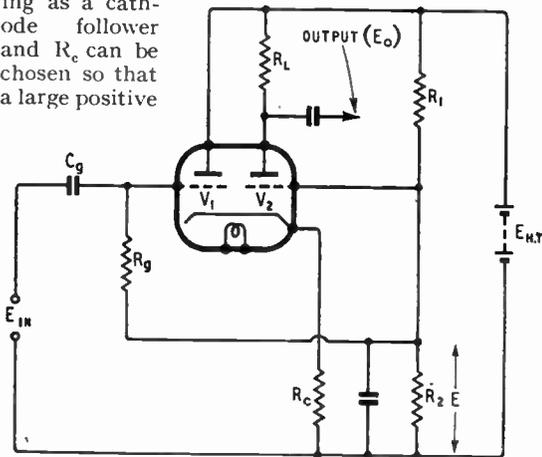
as the standard pentode type) the current charges the grid coupling condenser and imposes an undesired negative bias on the valve. This can only be eliminated by ensuring that such a limiter is driven from a low-impedance source—a requirement which is not imposed by the double triode circuit.
