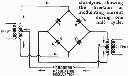
What happens to it depends on their relative phases. If it is in phase, the carrier is full-wave rectified, giving a D.C. (plus carrier harmonics) output in one direction, Fig. 7 (a); while if the phase difference is 90° the change-over in polarity of the carrier occurs half-way through each half-cycle of the modulating signal, and cancels out, giving no output.
