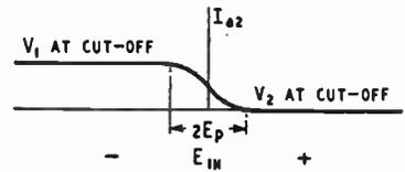
**Fig. 3. Characteristics of limiter.**
