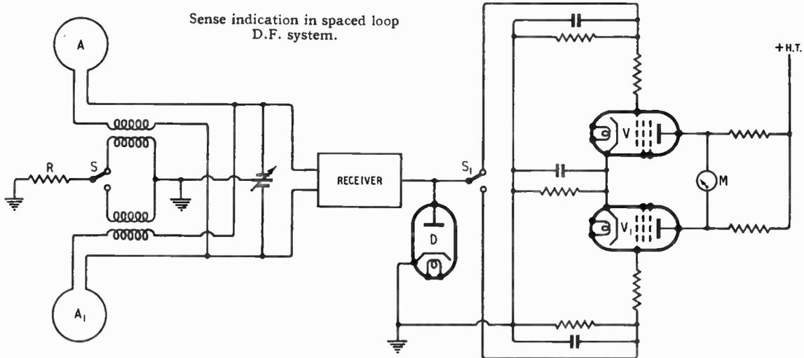
duction of the resistance R in the aerial circuits creates a different sequence of deflections, to right and left, in the centre-zero meter M, as the aerial system is rotated clockwise. This allows the directional sense of each of the four zero channels to be distinguished and identified.
