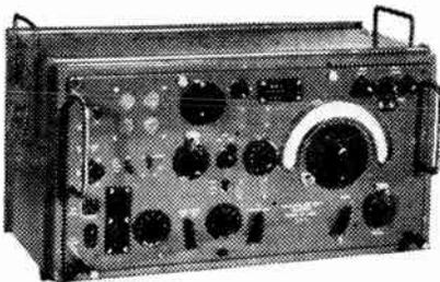
**R107. ONE OF THE ARMY'S FINEST COMMUNICATIONS RECEIVERS.** (See "W.W.", August, 1945). 9 valves, R.F. amp, osc. Frequency Changer, 2 I.F.'s (465 kc.), 2nd Detector, AVC. Af. amp. B.F.O. A.C. mains, 100-250 v. or 12 v. accum. Frequency range 17.5 to 7 mc s., 7.25 mc/s. to 2.9 mc/s, 3.0 to 1.2 mc s. Monitor L.S. built in. Complete. Write for full details, £16/18/-. Carriage paid.
