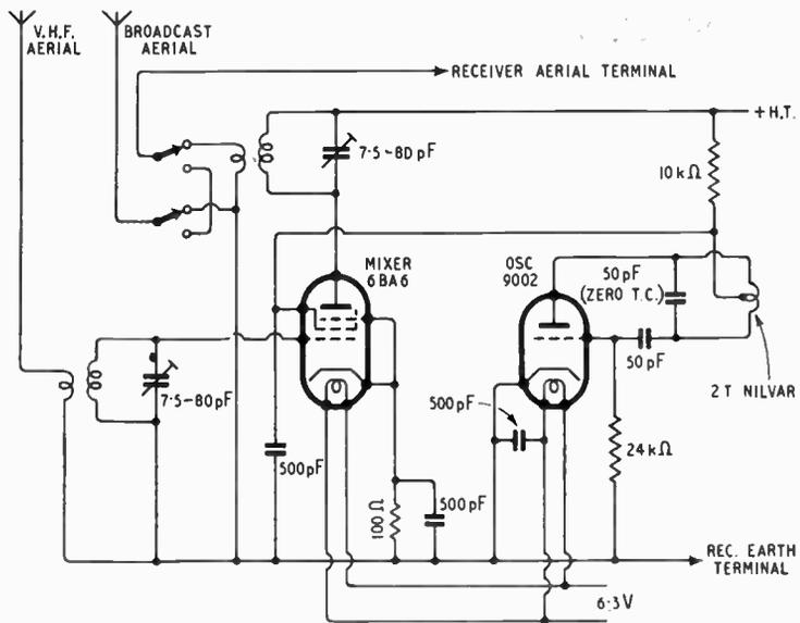
Fig. 1. Circuit diagram of the converter unit described. The input frequency is 87.75 Mc/s and the output 1,500 kc/s.
