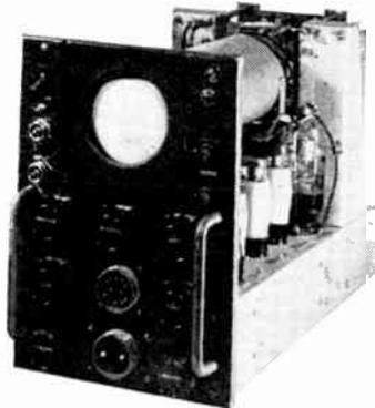
**TEST UNIT TYPE 73** consists of a special purpose Oscilloscope that requires only wiring and the addition of a few condensers and resistors to convert into a standard Oscilloscope, input 230 v. 50 c. A 3½in. C.B. tube and 1 8U220A, 1 EB34, 1 5Z4, 3 6P41, 3 EA50, are included. Controls are "Brightness," "Velocity," "X Shift," "Y Shift," "Focus Amplifier," "In/out," "Calibrate," "on off TX." Price £8/8/-. Carriage and packing 7/6.
