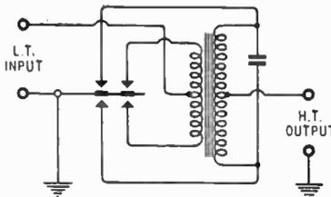
Fig. 1. Circuit of synchronous vibrator with transformer and "timing" condenser.
