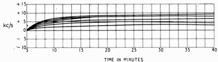
Fig. 2. Frequency stability curves of production models of the converter shown in Fig. 1.
