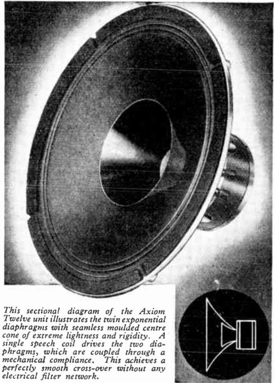
This sectional diagram of the Axiom Twelve unit illustrates the twin exponential diaphragms with seamless moulded centre cone of extreme lightness and rigidity. A single speech coil drives the two diaphragms, which are coupled through a mechanical compliance. This achieves a perfectly smooth cross-over without any electrical filter network.
