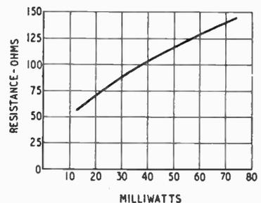
Fig. 3. Characteristic of tungsten-filament lamp used in bridge.
