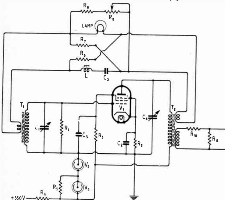
Fig. 1. Circuit diagram of high-stability LC oscillator.  $C_1, C_4$ , 950pF + 100pF variable;  $C_2$ , 2 $\mu$ F;  $C_3$ , 0.1 $\mu$ F;  $C_5$ , 500pF + 10pF variable;  $R_1$ , see text;  $R_2$ , 82 $\Omega$ ;  $R_3$ , 22,000 $\Omega$ ;  $R_6$ , 1,000 $\Omega$ ;  $R_7$ , 100,000 $\Omega$ ;  $R_8$ , 1,500 $\Omega$ ;  $R_9$ , 2,000 $\Omega$  variable;  $R_{10}, R_{11}$ , 50 $\Omega$ ;  $V_1$ , 6AG7;  $V_2, V_3$ , VR150;  $T_1, T_2, L$ , see text.
