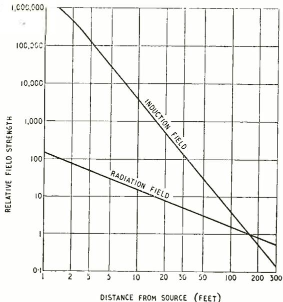
Fig. 6. Relative magnetic field strength at distances measured along the axis of a coil or loop 1ft in diameter energized by current at 1 Mc/s. The distance of the cross-over point (here 156 ft.) is proportional to wavelength.
