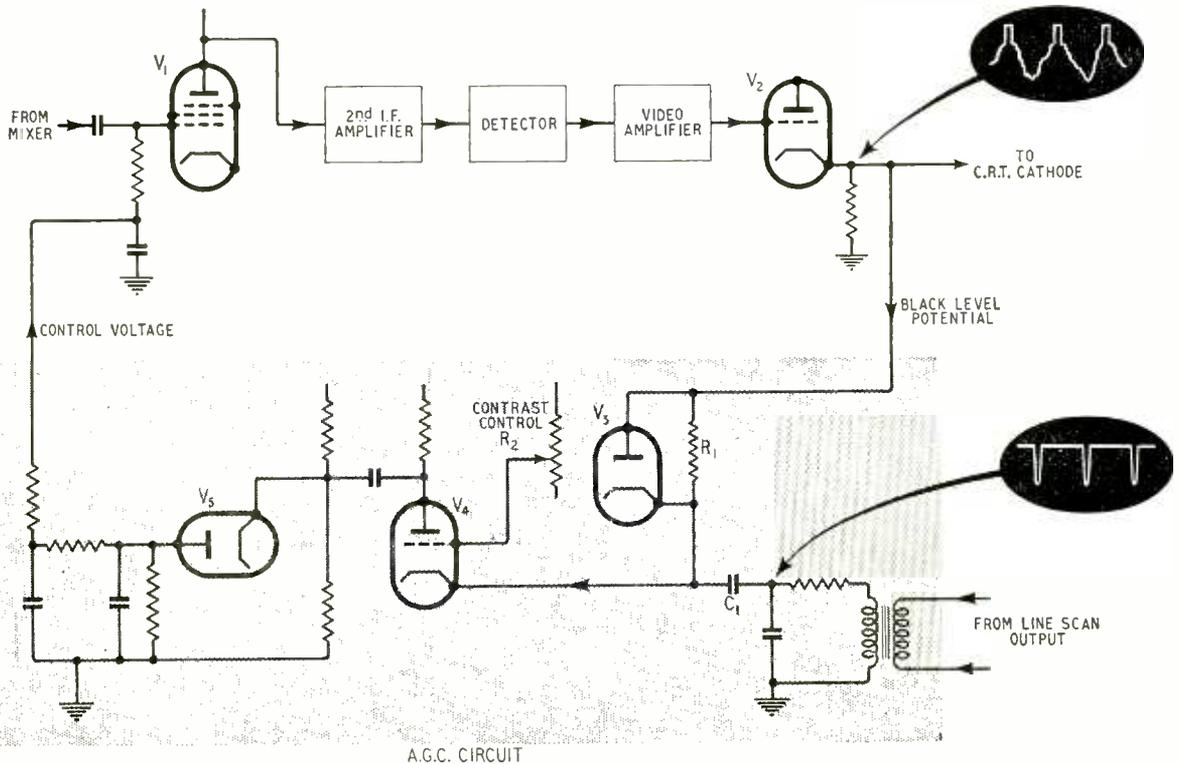
be necessary for the a.g.c. circuit to sample the signal at the correct instants and use these black-level samples to produce the control voltage. In adjusting the gain of the receiver to give correct contrast, its effect would be to maintain constant not the mean brightness of the picture, but the black level, which, of course, is just what is wanted.
