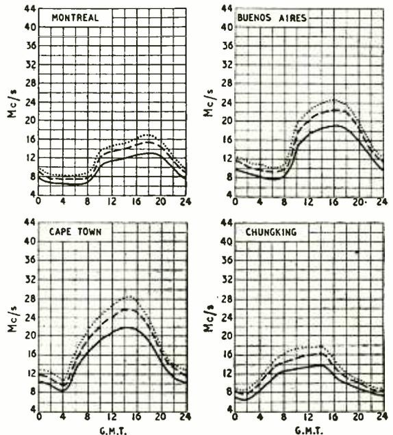
— FREQUENCY BELOW WHICH COMMUNICATION SHOULD BE POSSIBLE ON ALL UNDISTURBED DAYS
