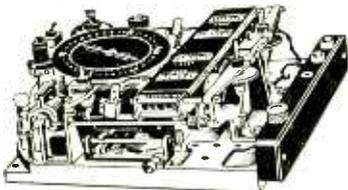
Containing a wealth of gears, drives, and shafts, 3 infinitely variable gears, lamp holders, repeater motors, Veeder counters, has been used by many Universities as a basis of a calculating machine £2/7/6.
