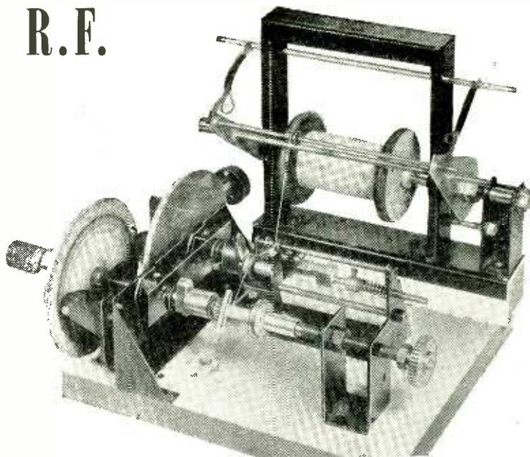
**W**AVE-WOUND COILS are so extensively used that it is thought an account of the author's winding machine may be of interest. It is capable of winding coils up to  $\frac{1}{2}$  in wide and can accommodate formers 2 in long. The machine is of simple construction, does not require any specially machined parts and is made largely from pieces of scrap. Few detailed measurements only are given in the following description as the majority can be varied according to the materials available.
