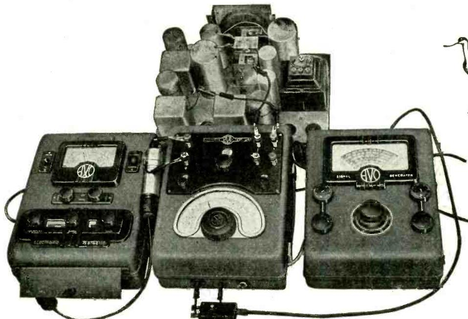
The illustration depicts a set of modern "AVO" testgear being used to measure the "Q" of the secondary winding of the second I.F. transformer on a chassis of unknown characteristics—just one of many tests which can be performed by this combination of instruments.
