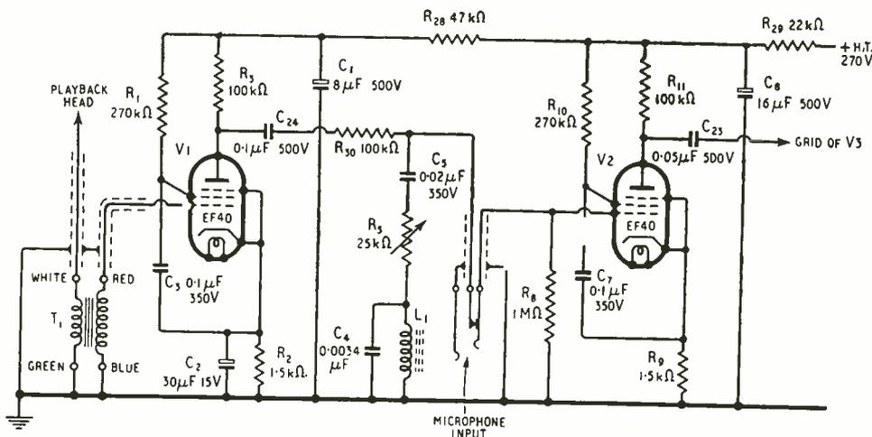
Fig. 3. Playback equalizing circuit. Fixed resistors can all be of  $\frac{1}{2}$ -watt rating, but  $R_3$  and  $R_{11}$  should be of the high-stability type. A silvered-mica capacitor should be used for  $C_4$ . Transformer Type 977 and choke Type 727, made by Wright and Weaire, can be used for  $T_1$  and  $L_1$  respectively.
