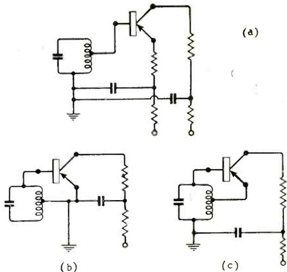
Fig. 5. Variants of the base-controlled oscillator circuit.
