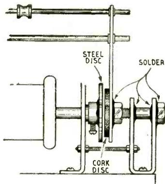
Fig. 7. Details of the tension-operated wire brake.
