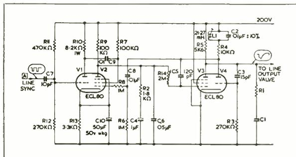
Fig. 1—Typical "Flywheel" Synchronising Circuit.
