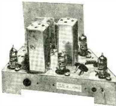
Superhet. Medium and short wave bands. 200-500 M. and 19-50 M. Uses 1 each 1R5, 1T4, 1S5 and 3S4 valves. 465 Kc/s. I.F. Circuit available.
