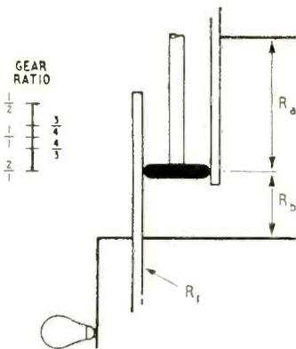
Fig. 3. Method of calculating the gear ratio.
