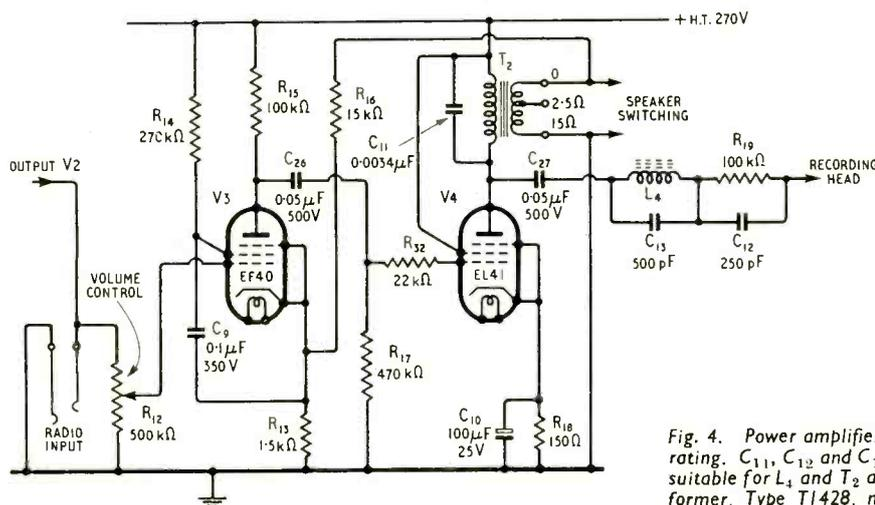
Fig. 4. Power amplifier circuit. Resistors are of  $\frac{1}{2}$ -watt rating.  $C_{11}$ ,  $C_{12}$  and  $C_{13}$  are silvered mica. Components suitable for  $L_4$  and  $T_2$  are the choke Type 666 and transformer, Type T1428, made by Wright and Weaire.
