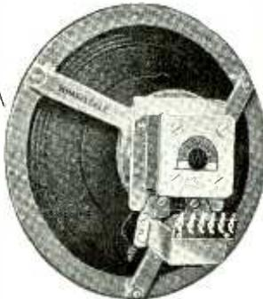
With a flux density of 10,000 lines, the speaker is in every respect equal to the pre-war GOLDEN unit. It is fitted with a wide response cone with bakelised apex, maximum input 6 watts on baffle, 8 watts in reflex cabinet. Speech coil 2-3 ohms or 12-15 ohms. Fitted with heavy die cast chassis. Transformer extra.
