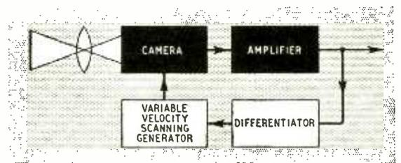
Fig. 6. System for controlling the velocity of the camera scanning beam according to the amount of information in the picture.
