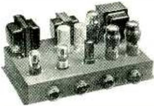
N.S.P. Major 8½ watt Quality Amplifier = PP6V6—Independent Bass and Treble boost and cut—neg. Feedback—provision for Radio Feeder Unit—Freq. response 25 to 20,000 c.p.s ± ½ DB—hum 80 DB down at 6.5 watts—Feedback 14 DB. A.C. Model with Remote Control Unit, £17/10/-.
