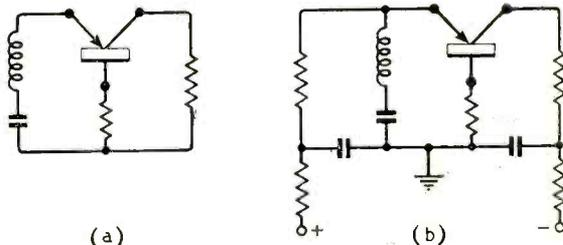
Fig. 6. Oscillator circuit (a) using negative emitter impedance when the base load resistance is high enough, and (b) method of connecting supplies.
