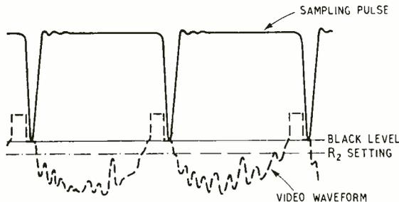
Fig. 2. Showing how the sampling pulses are d.c. restored to the black level potential of the inverted video waveform from the cathode follower.
