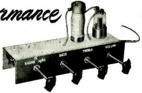
For use with any amplifier and pick-up, this preamplifier employs two valves in a well designed circuit providing variable boost and cut between  $\pm 15$ -20 db at 50 and 10,000 c/s respectively. Fitted also with a three position SELECTOR indicating "Radio," "78" and "33 $\frac{1}{2}$ ." Fixed frequency compensation
