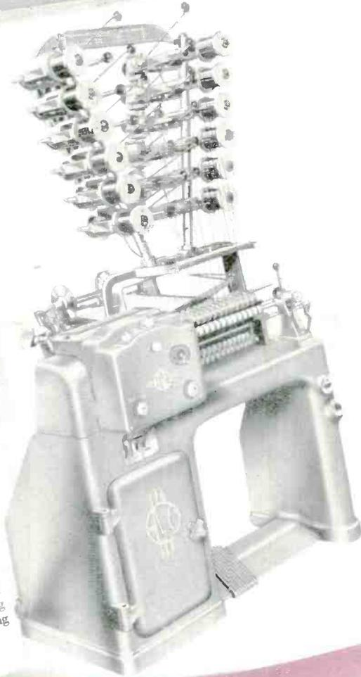
This typical page from our complete Catalogue shows the "Douglas" Fully Automatic Multi-Winder, designed for the high speed production of large quantities of coils with or without paper interleaving.
