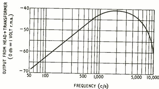
Fig. 2. Frequency response curve (uncompensated) of head and transformer, from a recording made under constant-current conditions.
