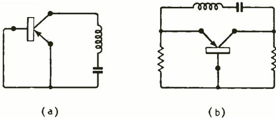
Fig. 8. (a) Shows a resonant circuit in the output (collector) loop of an earthed-emitter circuit. Re-drawn as in (b), with resistors added, it becomes an earthed-base amplifier with feedback from collector to emitter.
