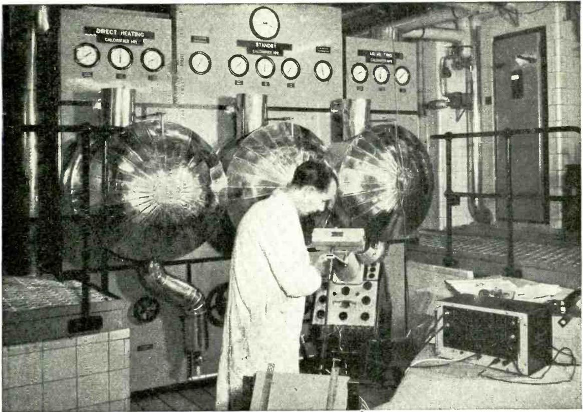
**AT THE NEW HOUSE OF COMMONS** the Research Department of Messrs. **Watford Electric & Manufacturing Co. Ltd.** is using the **Cossor Model 1049 Double Beam Oscillograph and Camera** together with **D.C. Pre-Amplifier Model 1430** to record the dynamic temperature range, the humidity level and the performance of the servo-mechanisms in the automatic controller of one of the air-conditioning plants.
