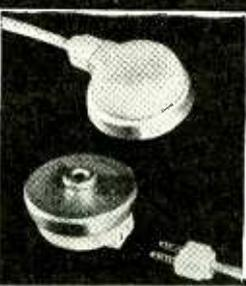
The new Amplivox E.4 Earphone has been primarily developed for use with office dictating machines, industrial equipments and hearing aids where a highly sensitive, lightweight, miniature receiver is needed. Available in D.C. resistances 2-2000 ohms; frequency 100-4000 c.p.s.; diameter .835"; depth .420"; weight 1/2 oz.
