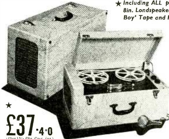
★ Including ALL parts, Valves, Portable Cabinet, 8in. Loudspeaker, Tape-Table, Reel of 'Scotch Boy' Tape and Rewind Spool, and Microphone.
