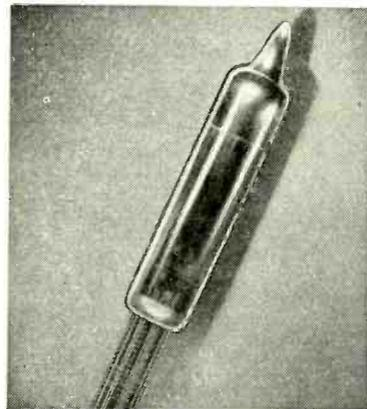
**A.C. Mains Receivers** The filament of the DM70 can usually be fed from a 6.3-volt transformer winding through a series resistor of  $220\Omega \pm 5\%$ . Alternatively, a 3.15V centre-tap on the heater supply can be used, the value of the series resistor then being  $82\Omega \pm 10\%$ .
