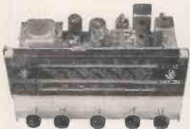
**RG/250.** 10 valve chassis with contrast expansion, variable selectivity. £35.
