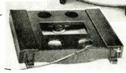
E. D. Parchment, 69, Clapham Road, London, S.W.9. It consists of a curved perforated back-plate with a stretched diaphragm of plastic film, coated on the outside with a metallic film. The whole is housed in a moulded plastic frame measuring approximately  $4\frac{1}{4}$  in  $\times$   $3\frac{1}{4}$  in  $\times$   $\frac{1}{2}$  in.
