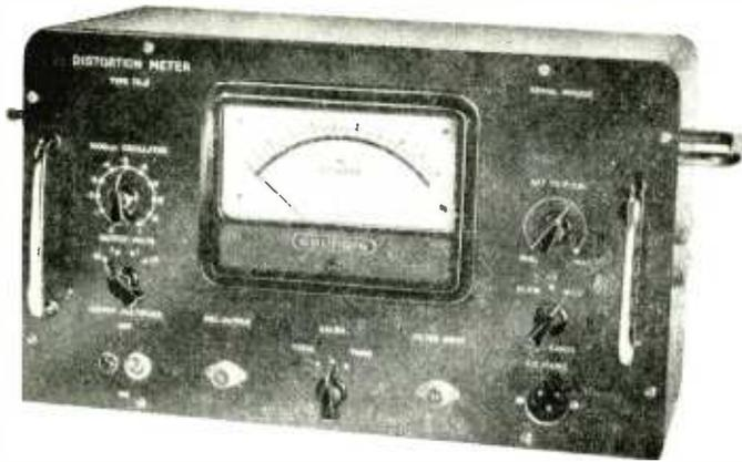
In the Grundig Type TGS distortion meter, controls associated with the 1,000-c/s oscillator are on the left and those for range selection and calibration on the right.
