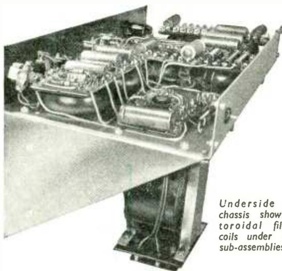
*Underside of chassis showing toroidal filter coils under RC sub-assemblies.*
