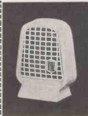
This attractive microphone is housed in a cream plastic case with gold background as illustrated. Fitted with type DX12 crystal insert as used on the famous "CORONATION" microphone, the frequency response is 30-13,000 c/s, and the output level at 1,000 c/s, 1.3 mv.  $\mu$  Bar in 5 Megohms.
