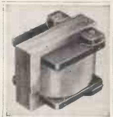
Small, efficient, low priced, size 1in. x ½in. x ½in. overall as illustrated. Uses: For coupling inputs of 3-150 ohms to normal type pentode valves. Specification: Ratio 1-50, Primary 3.5 ohms. Secondary inductance 160 H. at 1,000 c.p.s. Range 6½ octaves ± 2 db. Finish varnish dip, encapsulated block or mu-metal screening can. Quick delivery—low price—maximum efficiency
