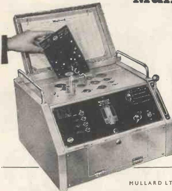
Industries which deal extensively with radio and other electronic equipment are finding the Mullard High Speed Electronic Valve Tester ideal for routine checks. This instrument provides the quickest method of checking large quantities of valves, and can be operated if necessary by non-technical personnel after only a few minutes' instruction. Write for full details and a copy of the folder "High Speed Testing in Industry" to Department E.V.D. at the address below.
