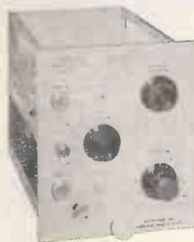
**Type 53A Wide-Band DC Plug-In Preamplifier**—dc to 10-mc passband, 0.035- $\mu\text{sec}$  risetime. Sensitivity 0.05  $\text{v/cm}$  to 50  $\text{v/cm}$ , ac or dc, continuously variable, with nine calibrated steps from 0.05  $\text{v/cm}$  to 20  $\text{v/cm}$ . Two input connectors with 80-db isolation. Price \$85.
