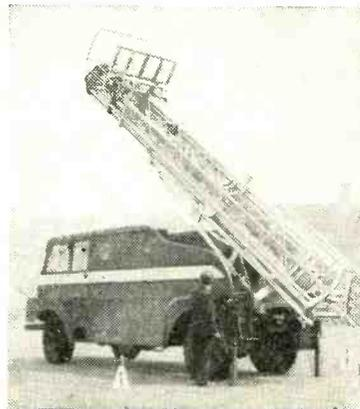
A PARABOLOID four feet in diameter is mounted on top of this 60-ft mobile extendable mast which the B.B.C. has recently introduced for television outside broadcasts. The aerial, which can be remotely rotated through 360°, can be adjusted to within  $\pm 1^\circ$ . When extended the mast is self supporting but provision is made for stay wires if needed.
