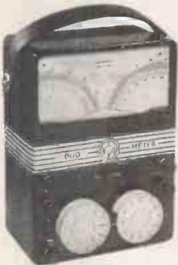
All-purpose test set enabling the simultaneous measurement of current and voltage.
