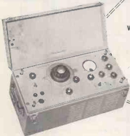
**Video Oscillator type 022B** + 10 to -50 db on 1 volt peak to peak from 10 kc/s - 10 Mc/s.
