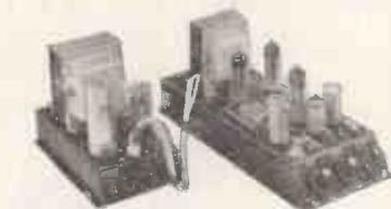
The MULLARD 5/10 Amplifier, built on printed circuit, supplied fully assembled, complete with valves, ready for use. Prices from **15 gns.** depending on make of transformer used.
