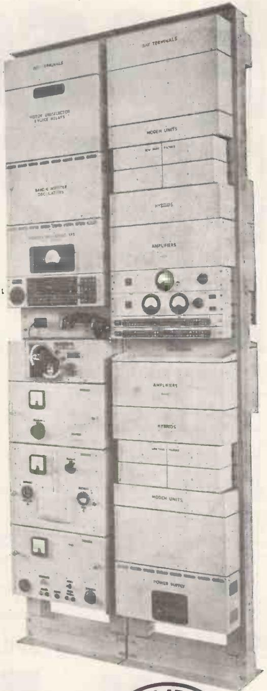
This equipment, which may be switched in or out of use at the radio terminal, provides a very high degree of privacy for speech on a radio-telephone circuit by:-
