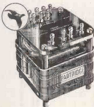
Optimum conditions are obtained in the form of output stage used in this amplifier when about 40% of the primary winding of the output transformer is common to anode and screen grid circuits. The Partridge Type P.3878 is of C-core design with windings of 43% of primary turns, and is specified by the designer for this amplifier.
