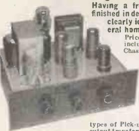
Designed for high quality reproduction up to an output level of 10 watts, having 6V6s in Push-Pull and incorporating negative feedback. It is suitable for use with all types of Pick-ups and most types of microphones and the output transformer provides for use of 3 and 15 ohm speakers.
