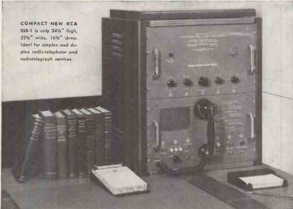
**FOR THE FIRST TIME** in HF Telecommunications, RCA is making available the proved advantages of single-sideband communications . . . at a cost everyone can afford. This technique of communications has been used in intercontinental telephony since 1926, but never before has it been offered at such a low price.
