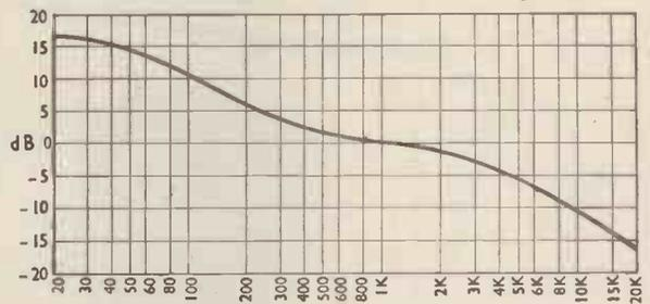
Fig. 2. Replay characteristic for coarse groove records. (Frequency in c/s).
