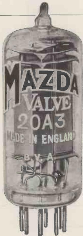
The 20A3 is a miniature indirectly heated tetrode thyatron which can be used as a high speed relay. It has a high control ratio, low grid/anode capacitance and passes a very low grid current. Used in conjunction with a high resistance circuit, the 20A3 can be operated directly from a high-vacuum photo-cell.
