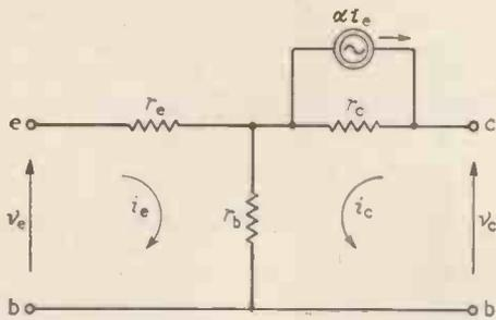
Fig. 1. Low frequency equivalent circuit.
