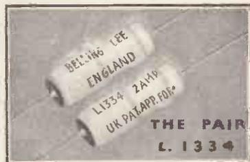
**L.1334. 2 Amp.** This very small inductor is essential for the filtering of interference on band III, and is individually tuned for use on band I. It must be fitted inside the casing of the appliance. When dealing with these very high frequencies, it is generally quite useless to attempt filtering in the flex lead, as the odd 6 in. of lead together with the overall dimensions of the appliance is an appreciable factor of the wavelengths and the whole acts as a radiator of interference.
