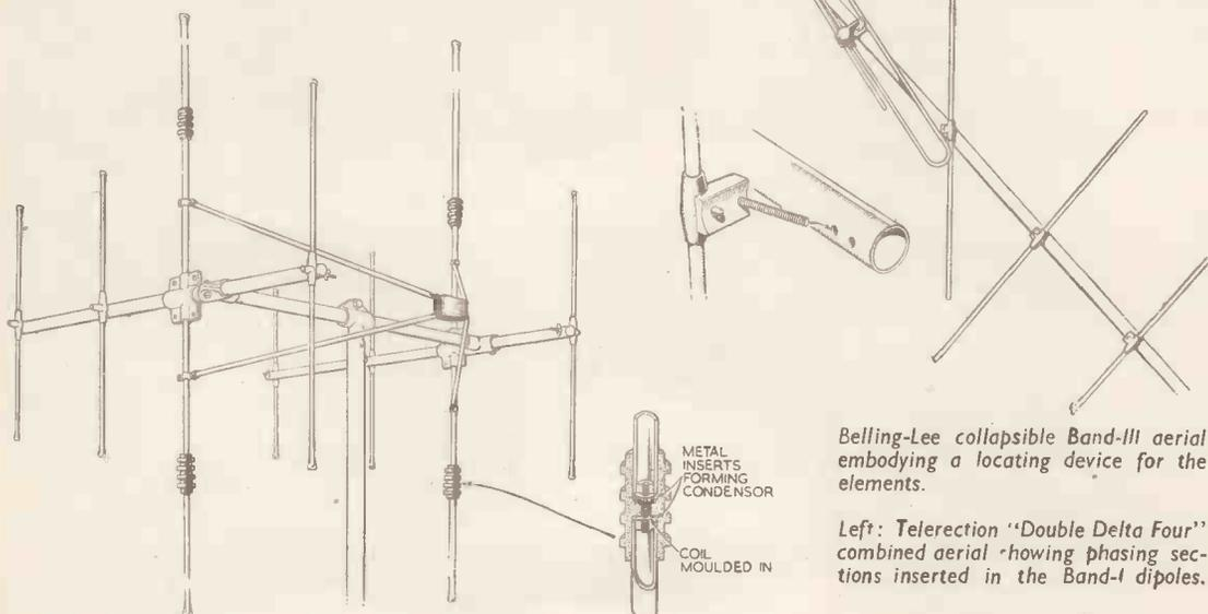
Belling-Lee collapsible Band-III aerial embodying a locating device for the elements.
