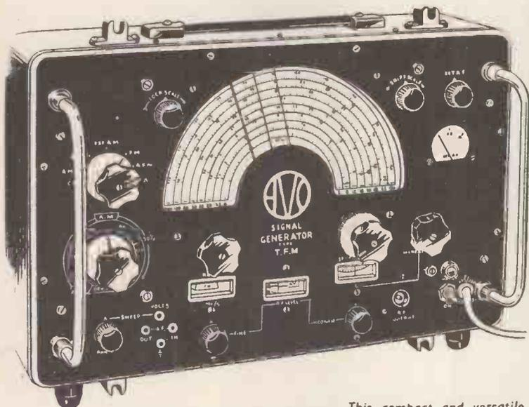
The frequency bands have been chosen in such a manner as to ensure maximum convenience when servicing and aligning T.V. and F.M. receivers.
