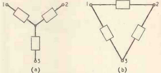
Fig. 1. Diagrams like this (or drawn with inductances in place of the oblongs) are common in books on 3-phase electric supply systems. They are called the star (a) and delta (b).
