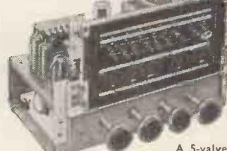
A 5-valve 3-waveband Superhet employing Negative Feedback over entire Audio Stages and having a single valve type 6BW6 output for approximately 4 watts. H.P. TERMS: PRICE **£11-11-0**
