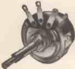
Thorough screening between switch and potentiometer. Concentric operating spindles give independent operation of switch or potentiometer with 'one-control' simplicity. Quick make-and-break action mains switch. Knob location to suit specified requirements. Type 154 with SPST switch, Type 155 with DPST switch.
