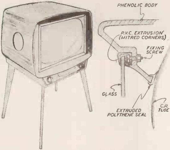
A method of sealing the air space between the glass and the tube face and moulding the mask as an integral part of the cabinet. As an alternative, the front portion alone could be moulded and attached to a simple wrapped-ply cabinet.
