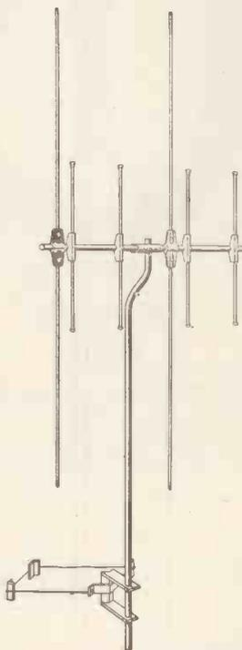
Band I "H" (Dipole and Director) Electronically coupled to 4 Band III elements for CHIMNEY MOUNTING. 17 HILO Models are available in all popular types of mounting, suitable for most areas, in any Band I|Band III channel combinations.
