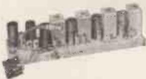
Size 10½ × 2½ × 3in. Frequency 9.72 Mc/s. 2 EF.92s and 1 EF.91 I.F. amps. EB.91. DET/AGC. EF.91 AGC. Amp. and EF.91 Limiter. Circuit supplied.
