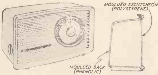
An alternative treatment of the two-piece cabinet in which the front escutcheon is constant. Either a moulded or a wrapped-ply back cover with internal fittings could be used.
