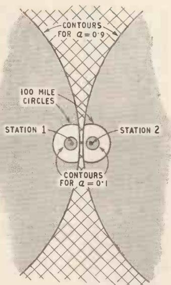
Fig. 2. Service areas (stippled) for capture ratios of 0.1 and 0.9 with co-channel transmitters spaced 100 miles apart.
