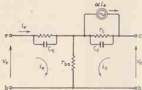
Fig. 2. High frequency equivalent circuit.
