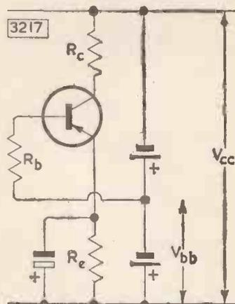
Circuit values can also be calculated, without using graphs. The procedure is as follows. (1) Choose  $V_{cc}$ ,  $V_{bb}$ ,  $I_{c\text{nom}}$ , and  $R_b$ . (2) Then
