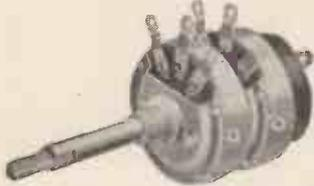
**DUAL POTENTIOMETERS** with concentric operating spindles. Incorporating many outstanding design features, including multiple contact rotors and thorough screening between sections. Control spindles can be supplied to suit customers' requirements. Type 136 less switch. Type 137 with SPST switch. Type 138 with DPST switch.
