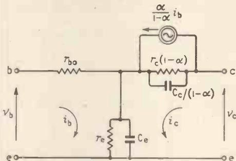
Fig. 4. The circuit of Fig. 3 modified so that amplification is expressed in terms of  $i_b$ .
